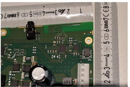
Antenna length: 26.5mm Antenna width: 6.2mm
