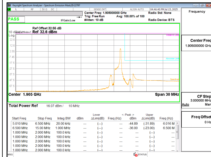
LTE2 10MHz QPSK HIGH Ch RB1-5
