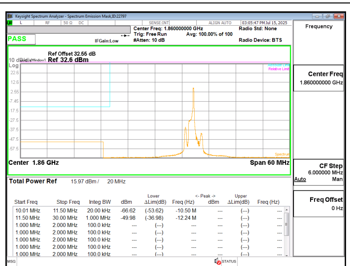
LTE2 20MHz QPSK LOW Ch RB1-5
