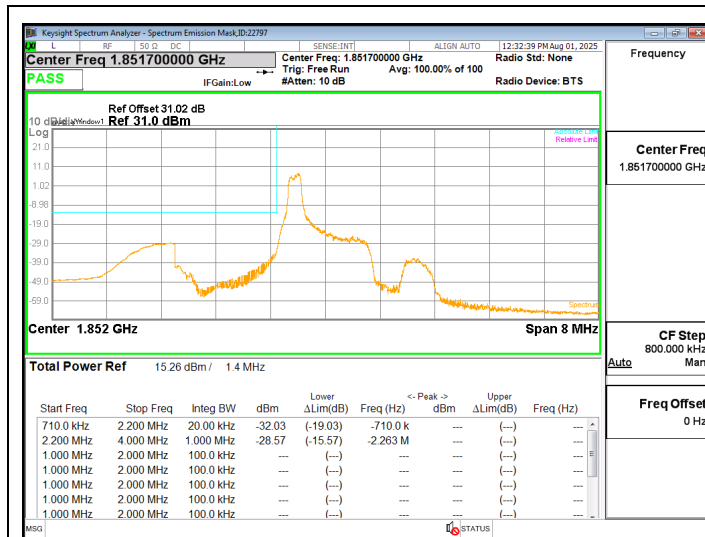
LTE2 1.4MHz QPSK LOW Ch RB1-0
