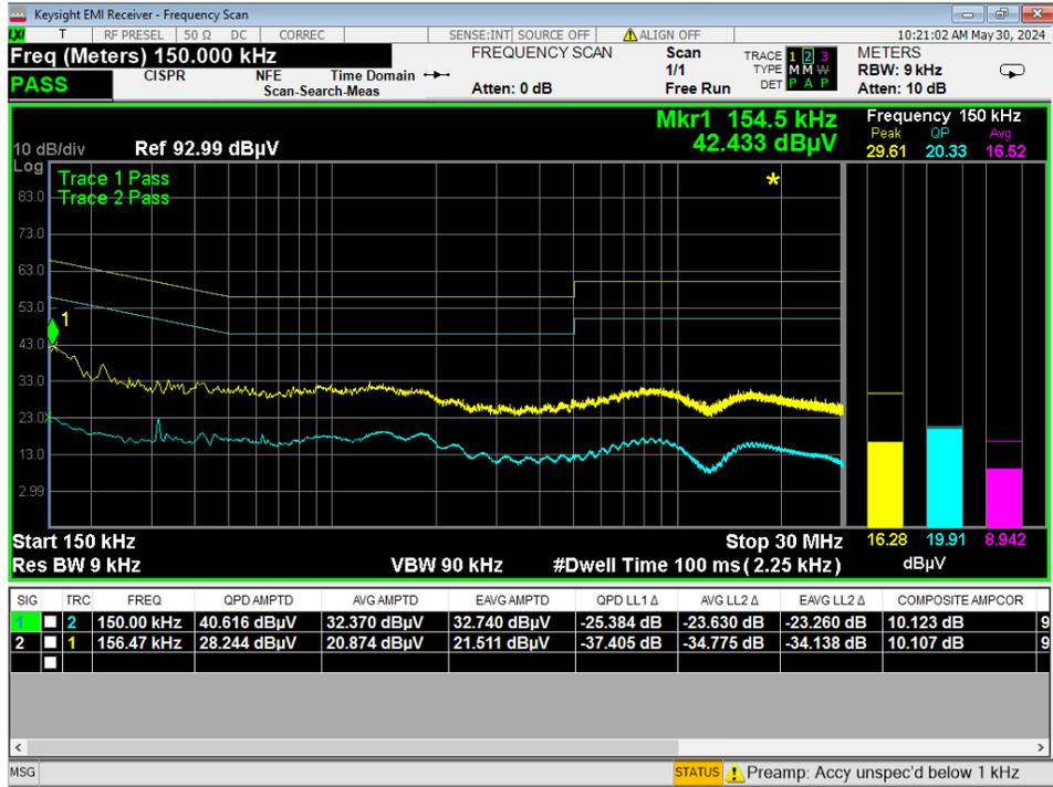
**Figure 6 - Conducted Emissions Plot, Line, TX, 120VAC/60Hz**
