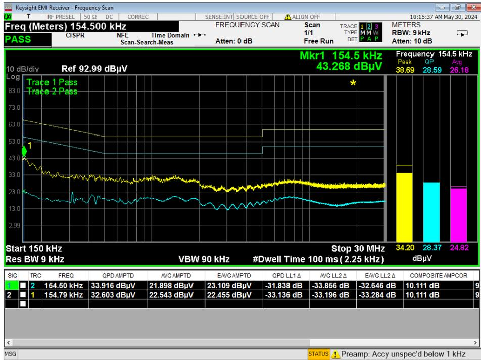
Figure 9 - Conducted Emissions Plot, Neutral, IDLE, 120VAC/60Hz
