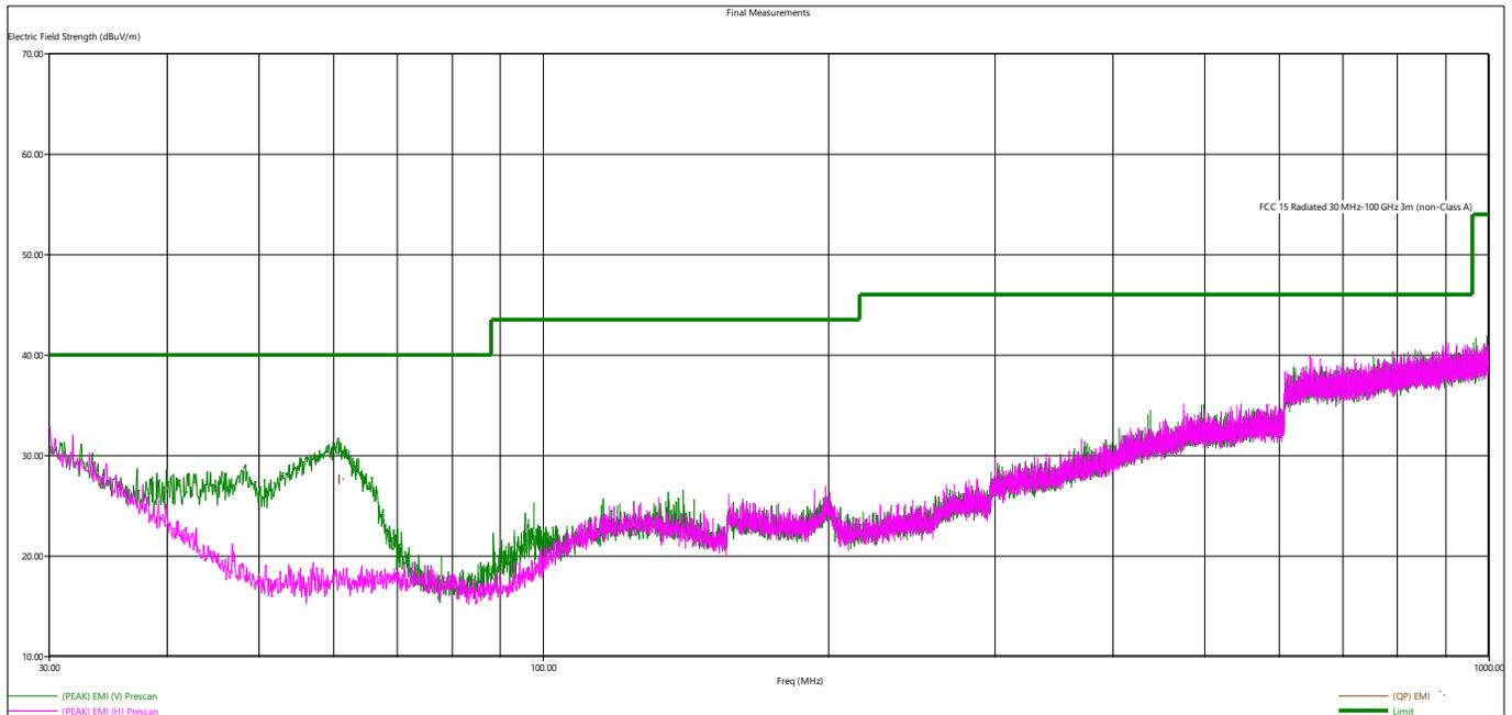
**Figure 5 - Radiated Emissions Plot, GFSK, Low Channel**
