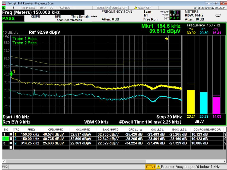
Figure 8 - Conducted Emissions Plot, Line, IDLE, 120VAC/60Hz
