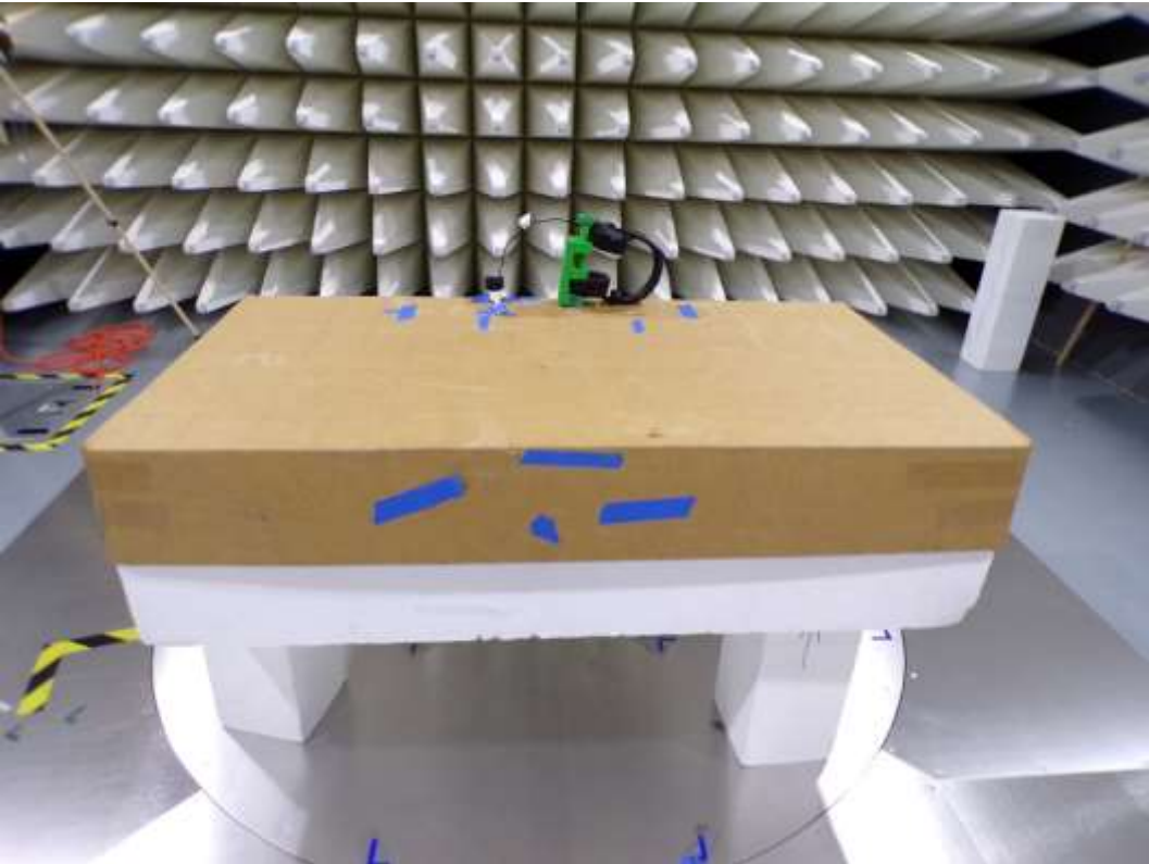
Figure RE09.2: EUT test setup, front view
