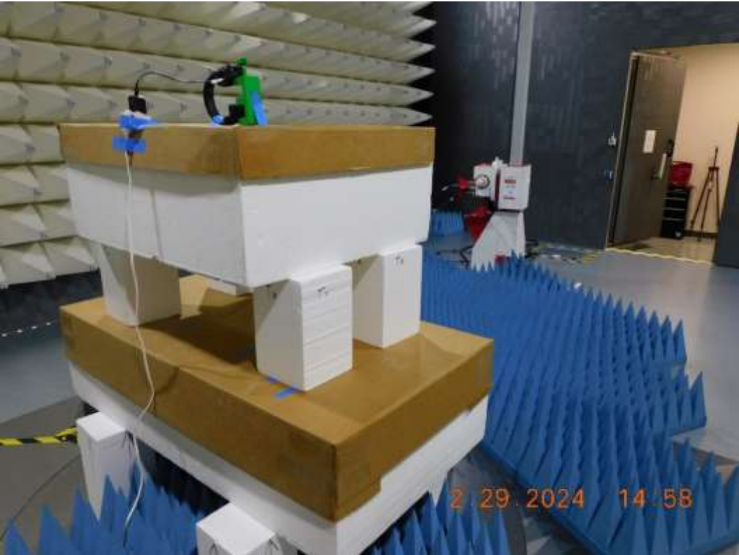
Figure RE03.6: EUT test setup, reverse view
