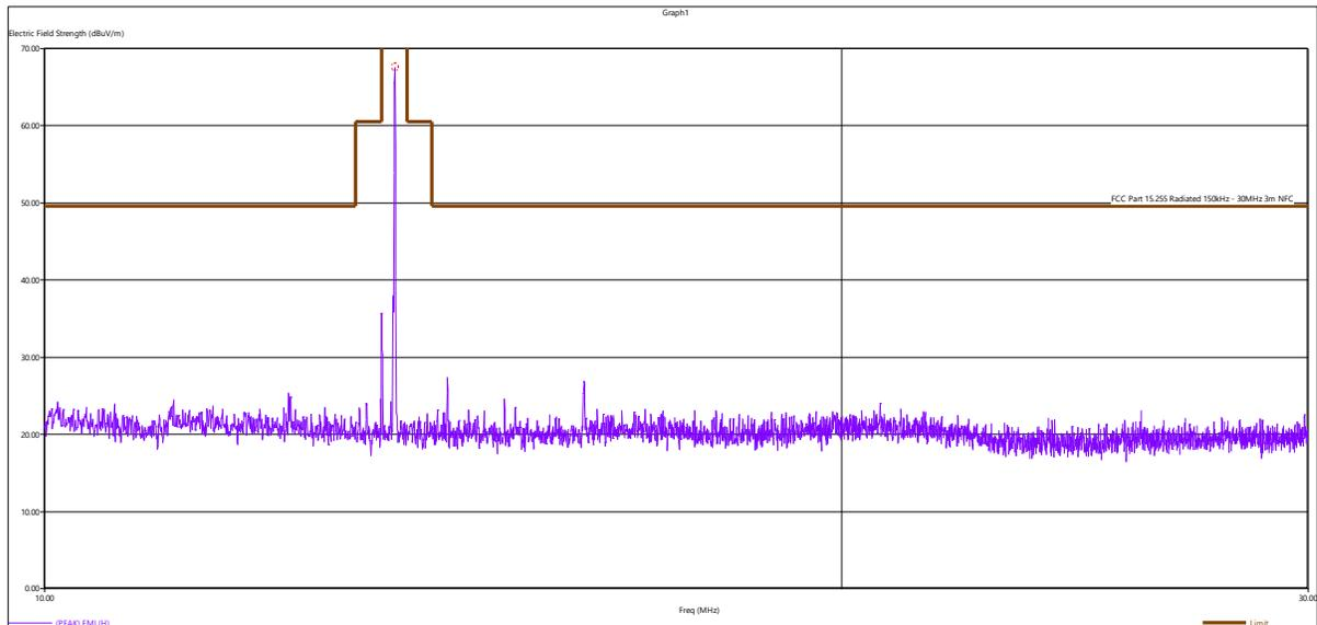
**Figure 1 – NFC Radiated Emissions Plot, 10MHz – 30MHz**
