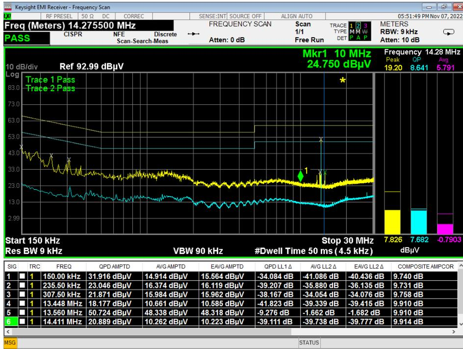
**Figure 7 – Conducted Emissions Plot, Line, NFC**
