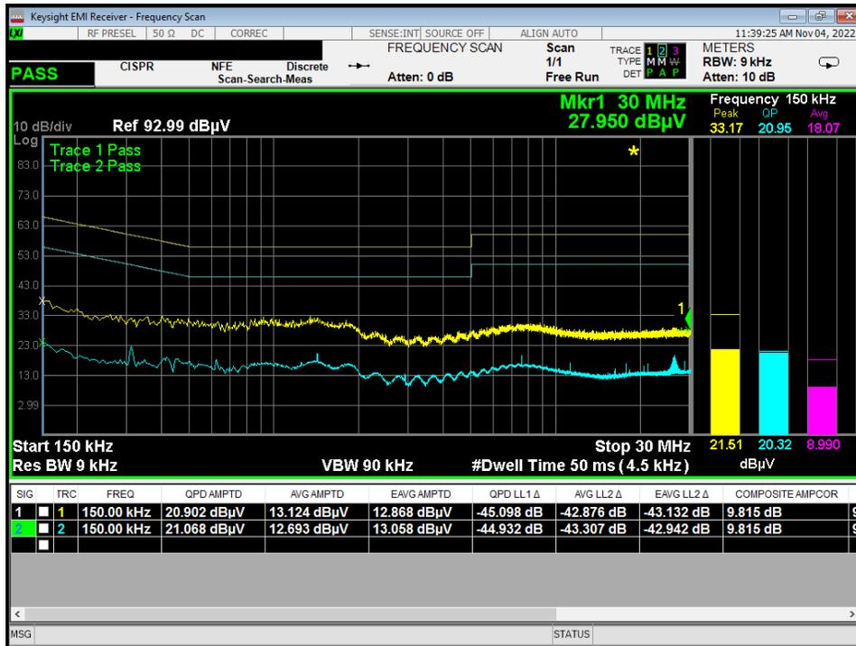
Figure 10 – Conducted Emissions Plot, Neutral, Idle
