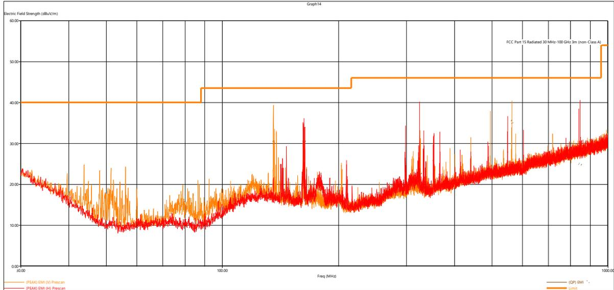
**Figure 2 – NFC Radiated Emissions Plot, 30MHz – 1GHz**
