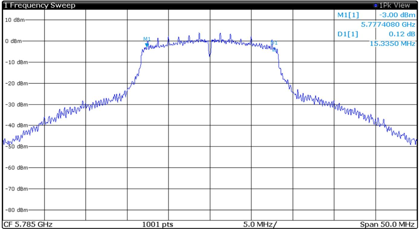
Figure 42 Plot of 6-dB Occupied Bandwidth 5725-5850 MHz Mode 13 (802.11n)
