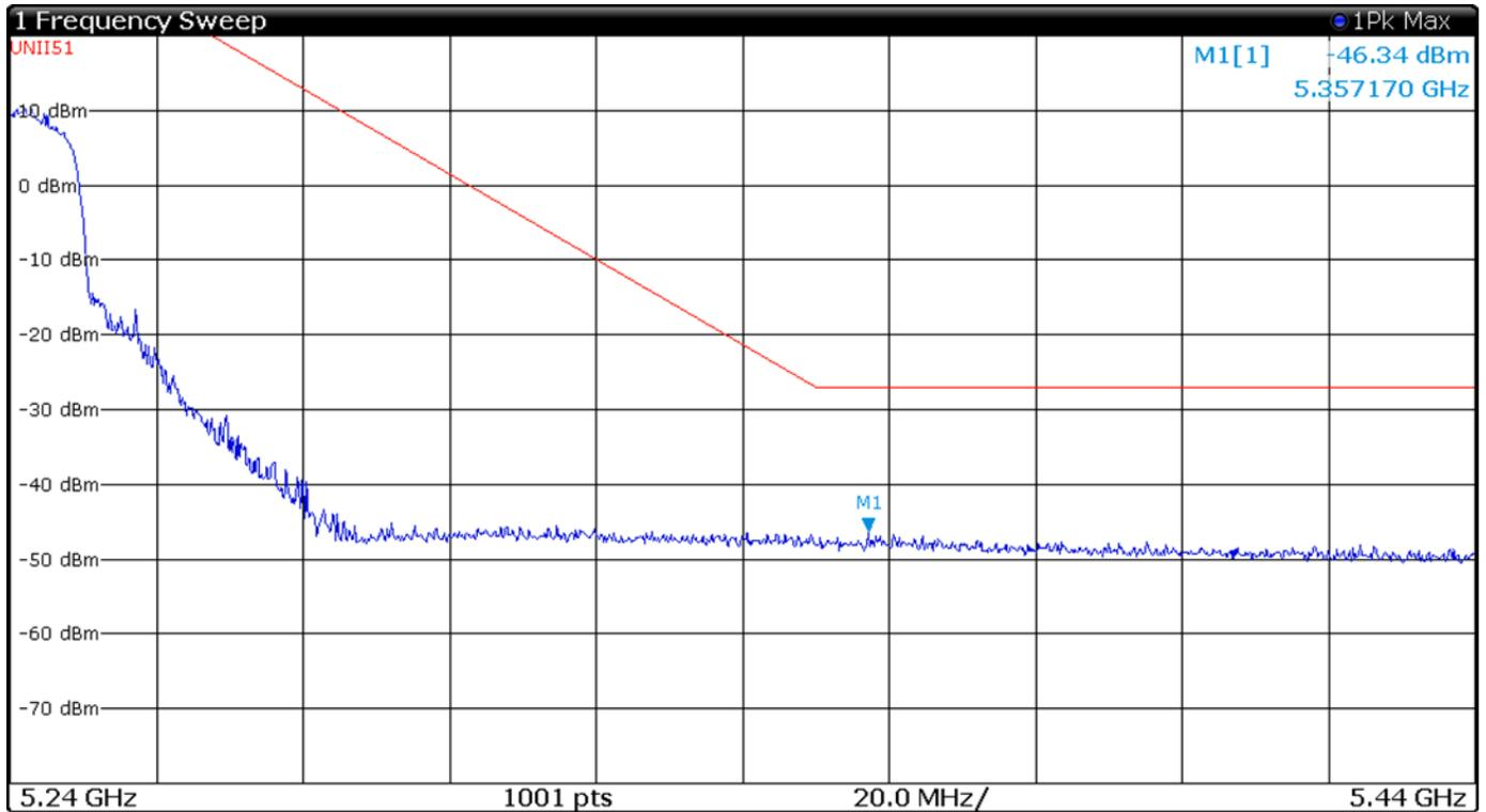
Figure 15 Plot of Upper Band Edge Across 5150-5250 MHz Mode 10 (802.11n40)
