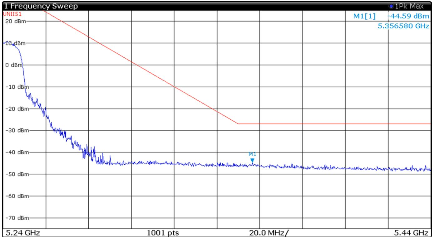
**Figure 14 Plot of Upper Band Edge Across 5150-5250 MHz Mode 9 (802.11n)**
