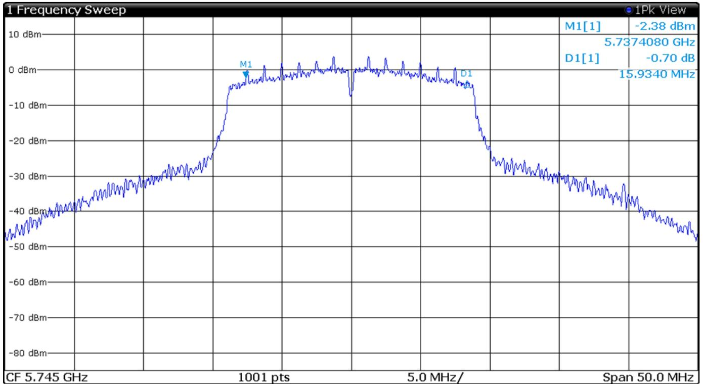
Figure 43 Plot of 6-dB Occupied Bandwidth 5725-5850 MHz Mode 14 (802.11n40)
