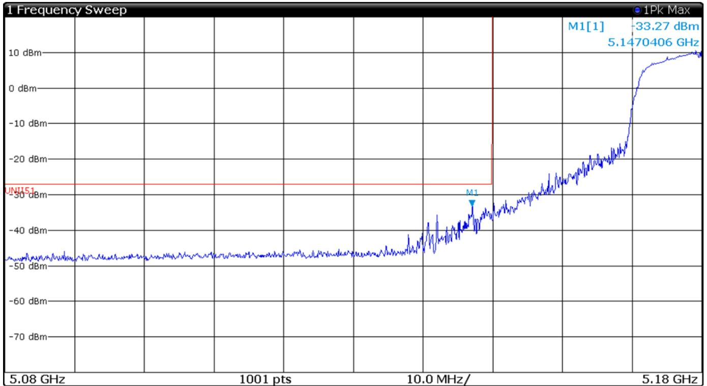
Figure 11 Plot of Lower Band Edge Across 5150-5250 MHz Mode 10 (802.11n40)
