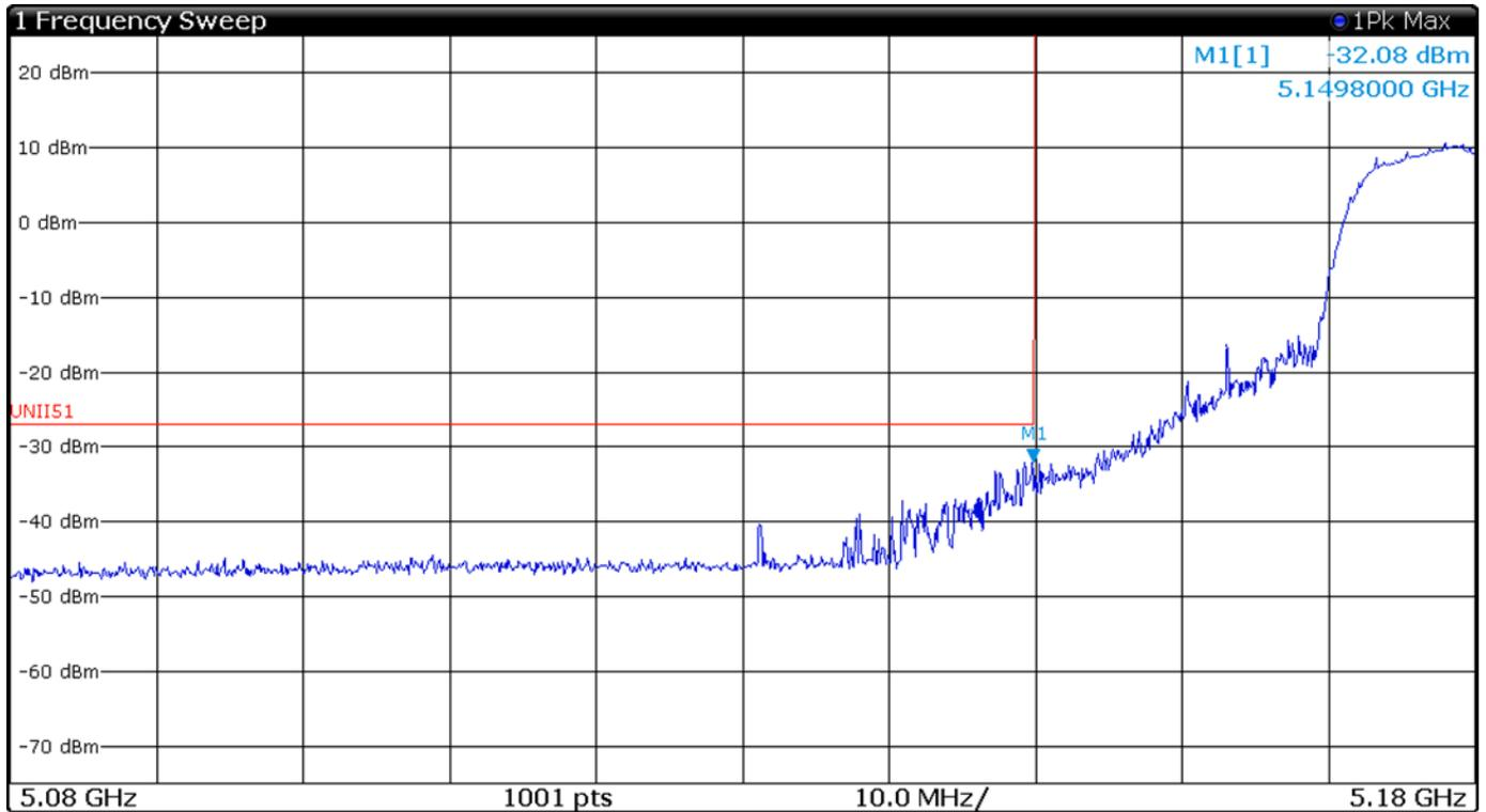
Figure 10 Plot of Lower Band Edge Across 5150-5250 MHz Mode 9 (802.11n)
