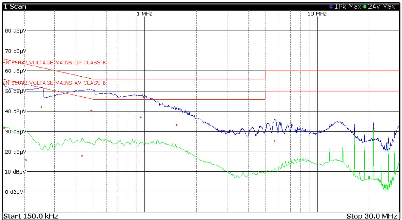
**Table 4 AC Line Conducted Emissions Data L1 (EUT – AC Adapter)**
