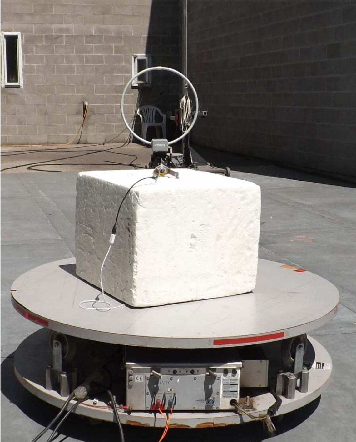
**Figure E20.3 – Setup, Radiated Emissions 30 - 1000MHz**
