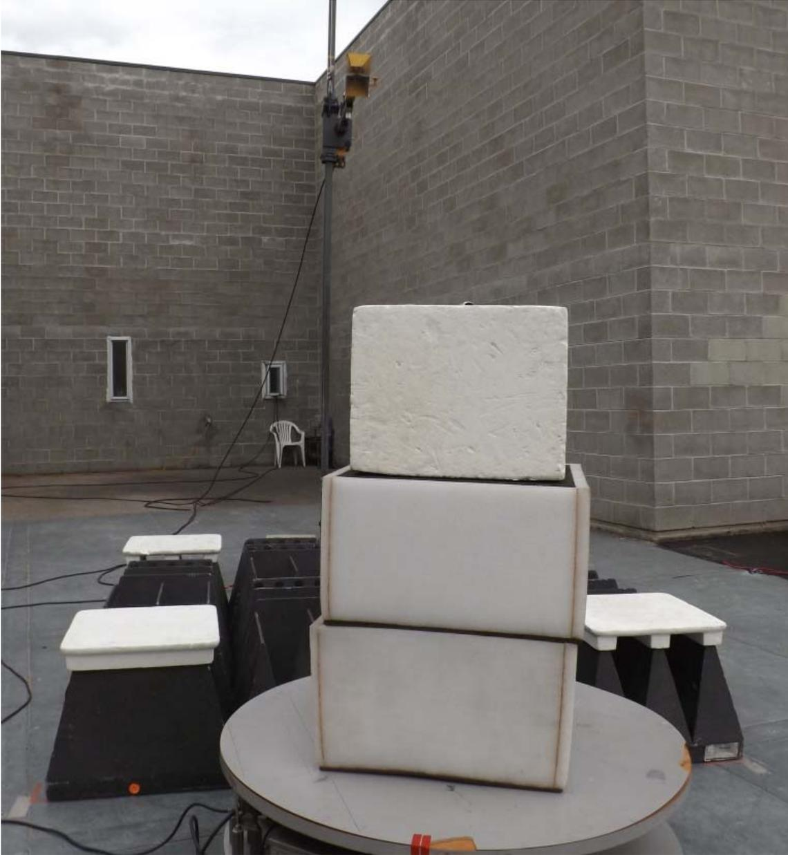
**Figure E20.5 – Setup, Radiated Emissions 18 - 26GHz**
