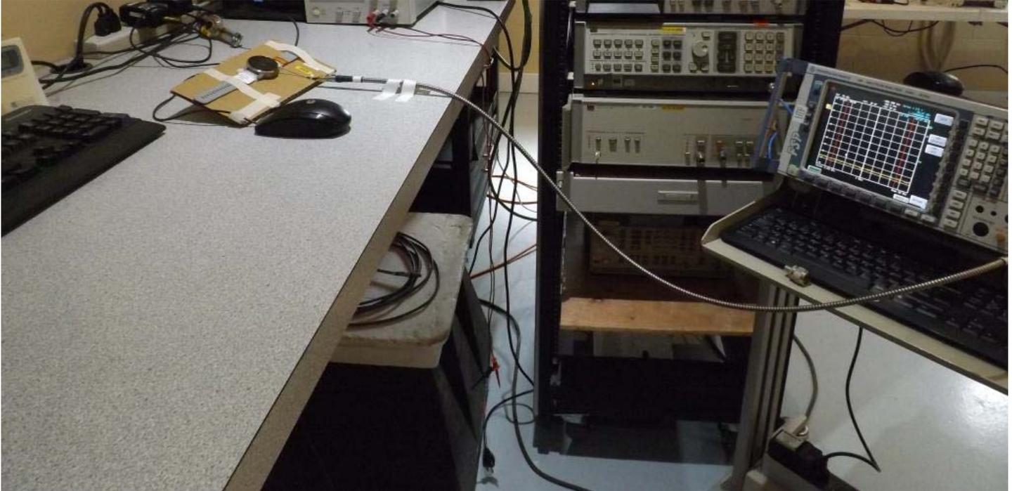
**Figure E20.2 – Setup, Radiated Emissions Below 30MHz**
