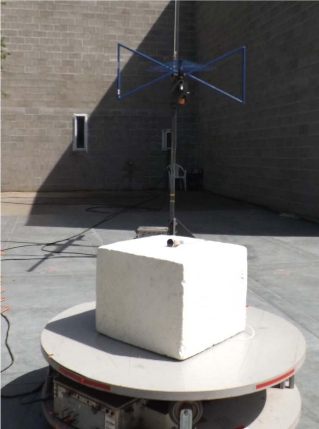
Figure E20.4 – Setup, Radiated Emissions 1 – 18GHz
