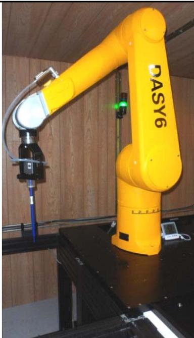
**DASY 6 SAR System with SAM Phantom**
