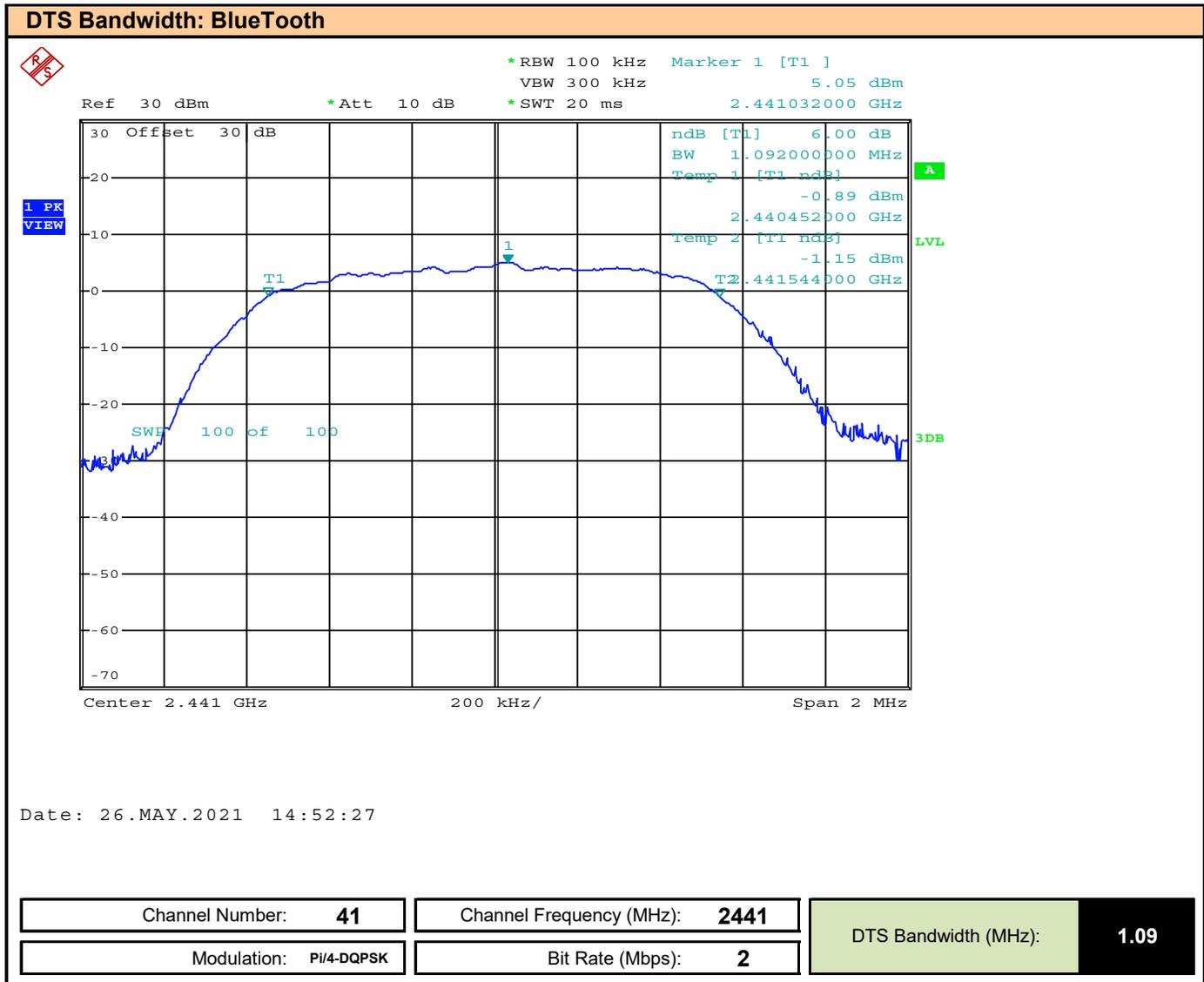
Plot 8.6 – 6dB DTS Bandwidth BT EDR 3MB, 2441MHz
