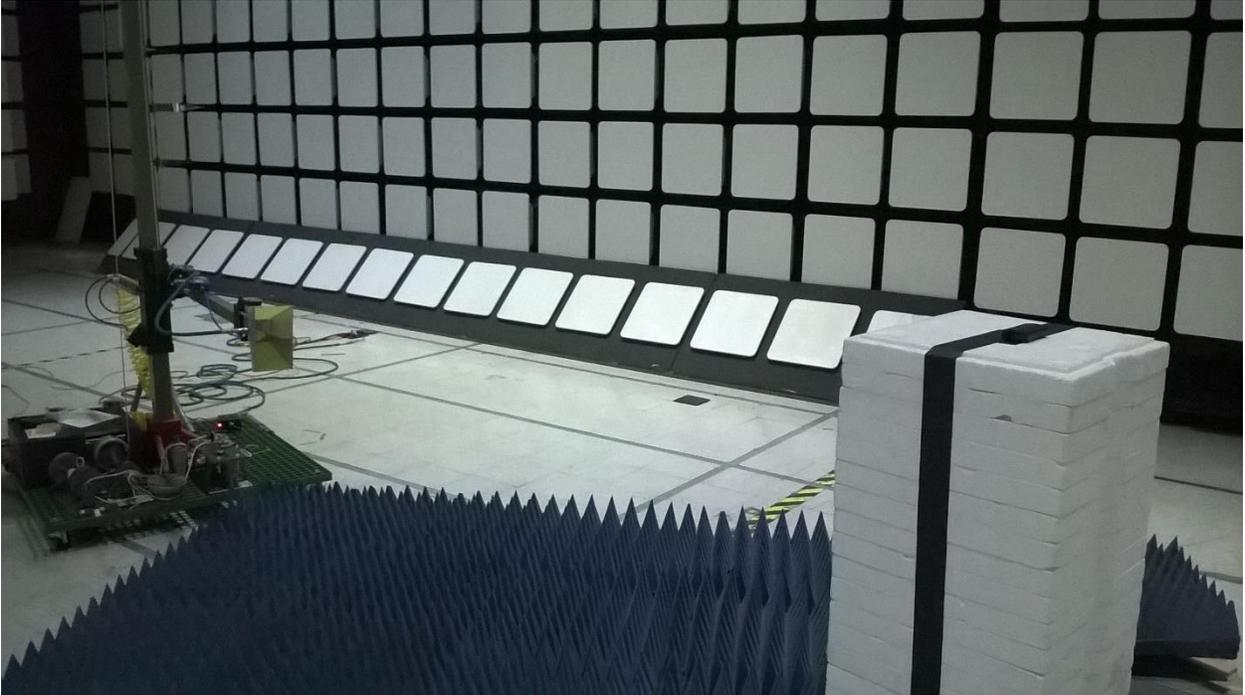
Radiated Emissions Test Setup, 1 - 18 GHz, (EUT not shown)
