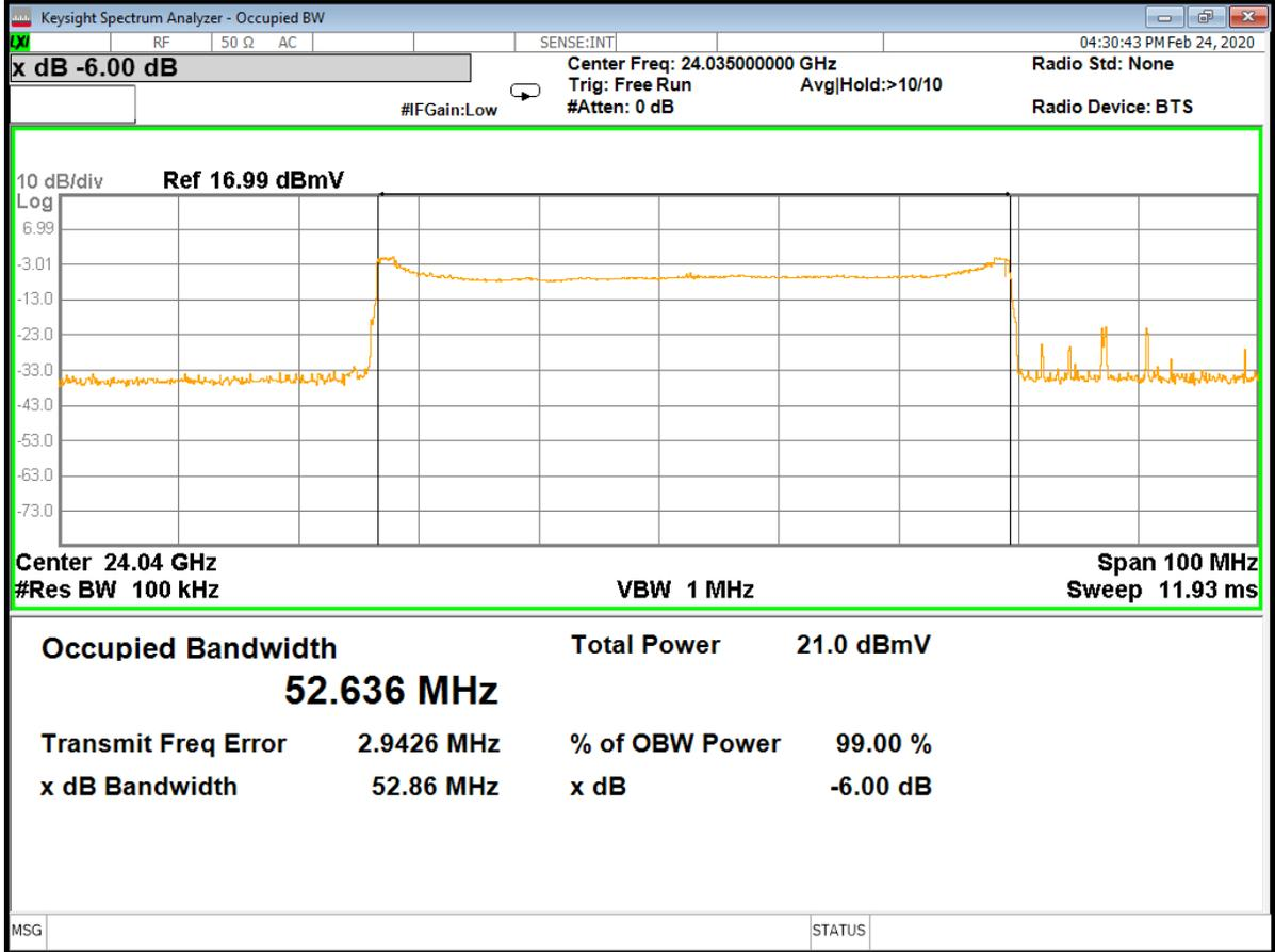
**Figure 39 – Occupied Bandwidth, Low channel (48 MHz)**
