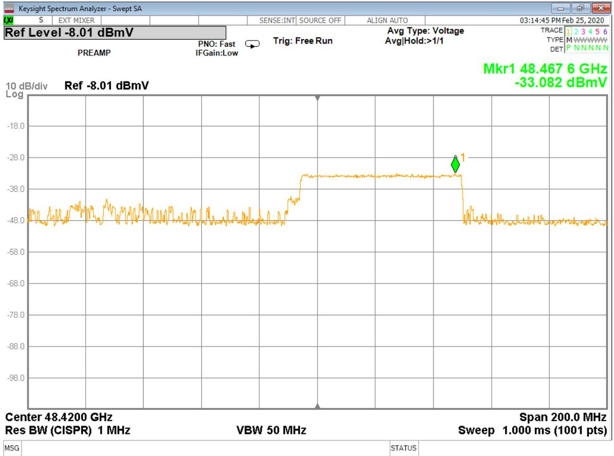
**Figure 10 - Analyzer Measurement – 2<sup>nd</sup> Harmonic, High Channel (24 MHz) (swept frequency)**
