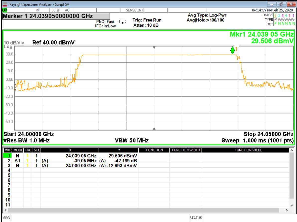
**Figure 30 – Lower Band Edge (24 MHz) (swept frequency), 24.00 GHz**
