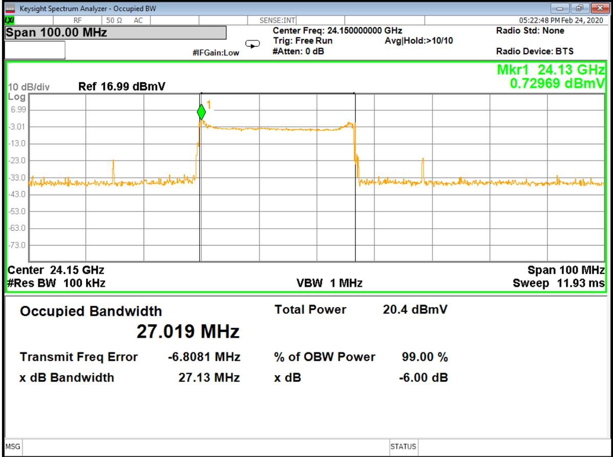
**Figure 37 – Occupied Bandwidth, Mid channel (24 MHz)**
