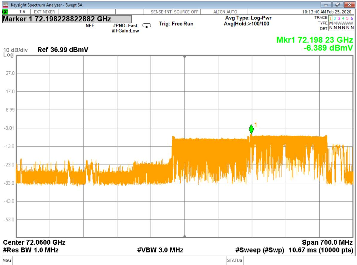
**Figure 14 - Analyzer Measurement – 3<sup>rd</sup> Harmonic, Low Channel (48 MHz) (swept frequency)**
