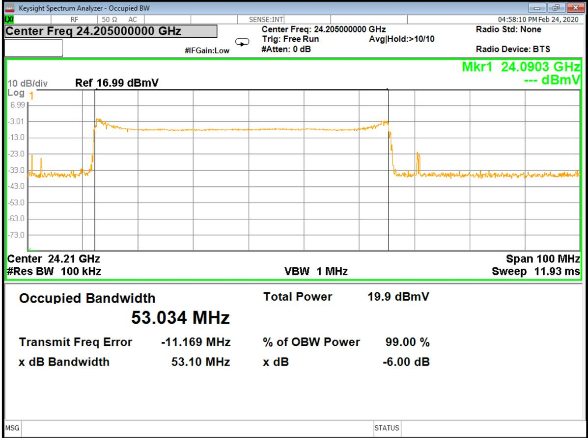
Figure 41 – Occupied Bandwidth, High channel (48 MHz)
