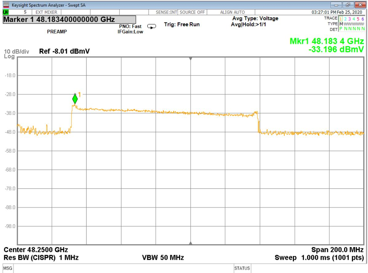
Figure 16 - Analyzer Measurement – 2<sup>nd</sup> Harmonic, Mid Channel (48 MHz) (swept frequency)
