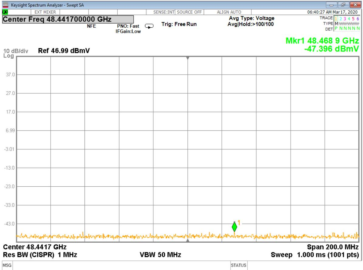
**Figure 28 - Analyzer Measurement – 2<sup>nd</sup> Harmonic, High Channel (Single Frequency)**
