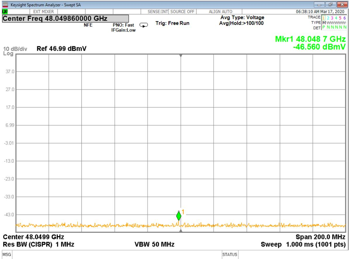
**Figure 22 - Analyzer Measurement – 2<sup>nd</sup> Harmonic, Low Channel (Single Frequency)**
