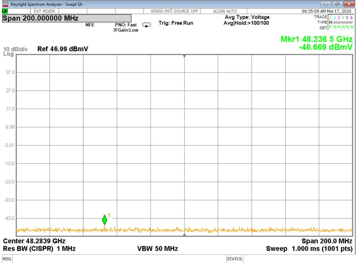
**Figure 25 - Analyzer Measurement – 2<sup>nd</sup> Harmonic, Mid Channel (Single Frequency)**
