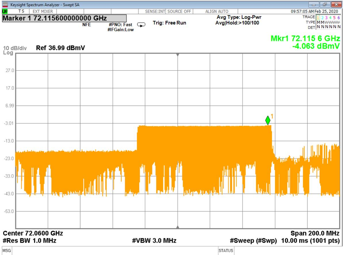
Figure 5 - Analyzer Measurement – 3<sup>rd</sup> Harmonic, Low Channel (24 MHz) (swept frequency)
