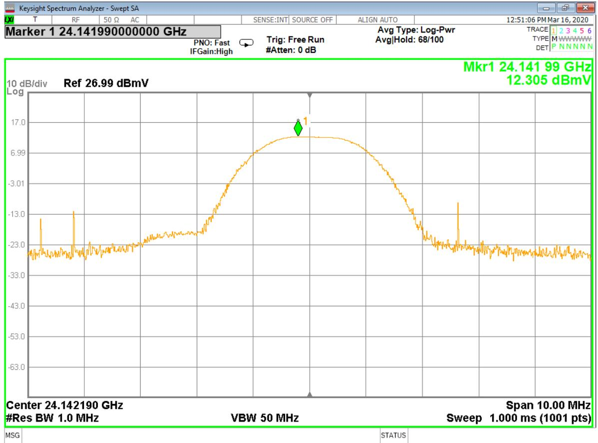
**Figure 24 - Analyzer Measurement – Fundamental, Mid Channel (Single Frequency)**
