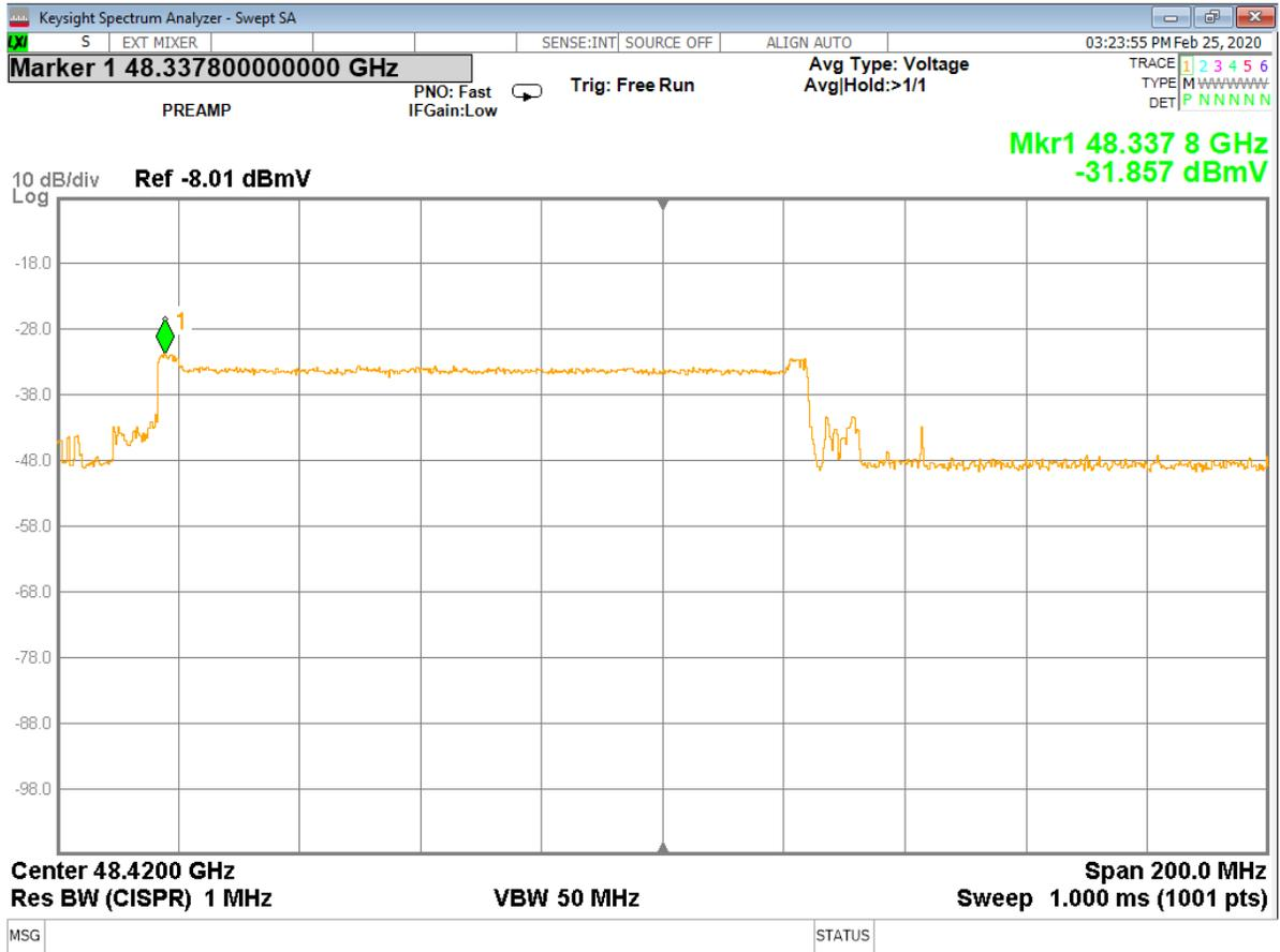
**Figure 19 - Analyzer Measurement – 2<sup>nd</sup> Harmonic, High Channel (48 MHz) (swept frequency)**
