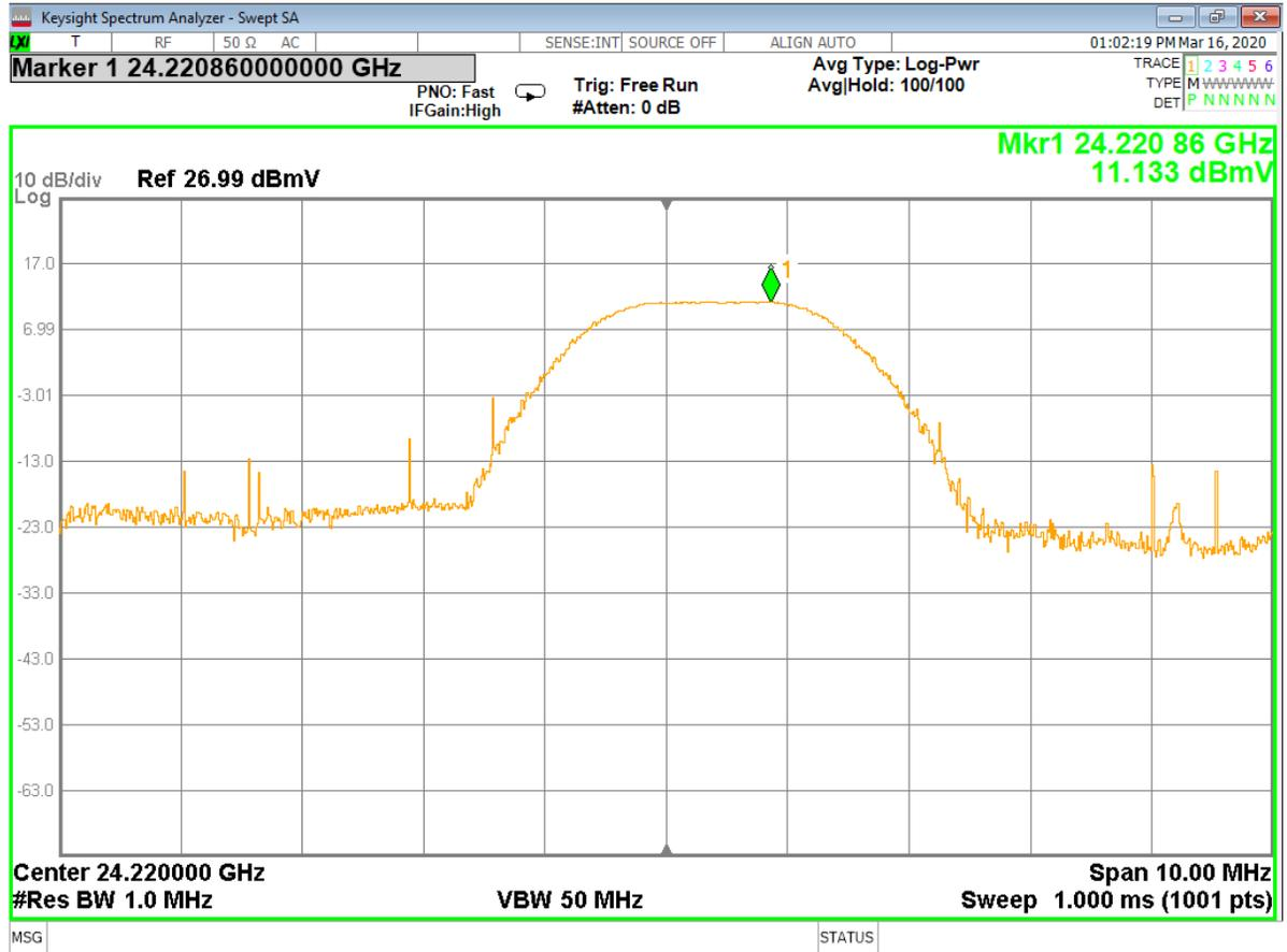
Figure 27 - Analyzer Measurement – Fundamental, High Channel (Single Frequency)
