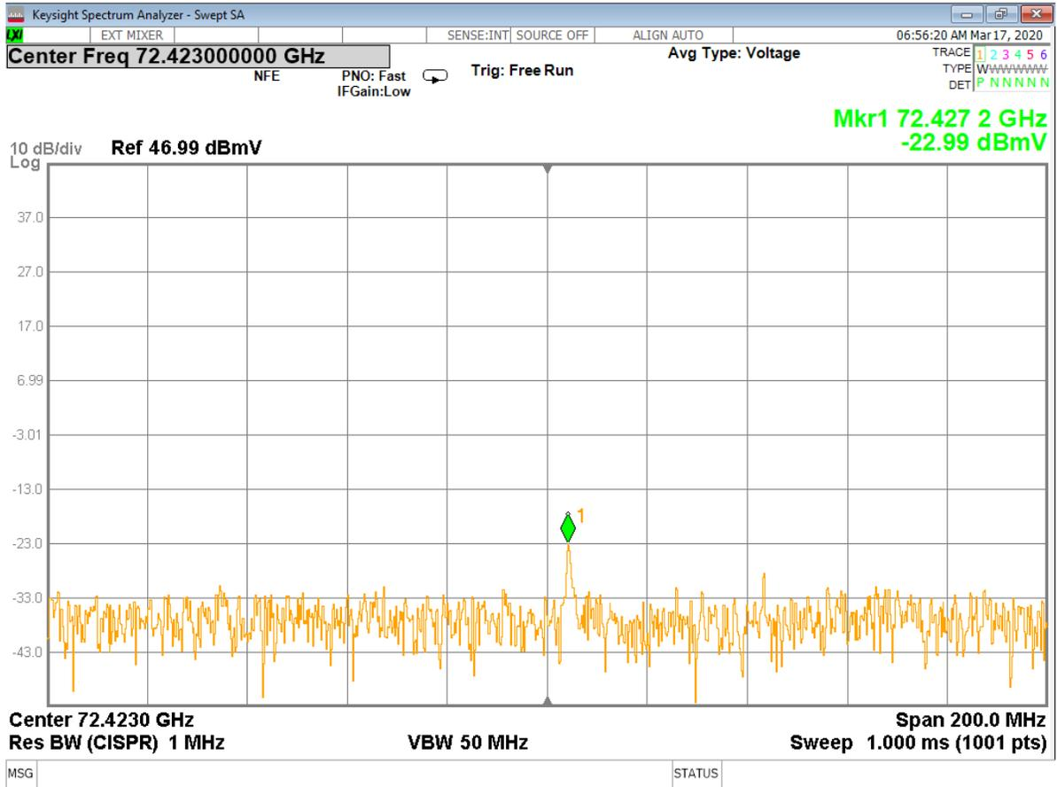
**Figure 26 - Analyzer Measurement – 3<sup>rd</sup> Harmonic, Mid Channel (Single Frequency)**
