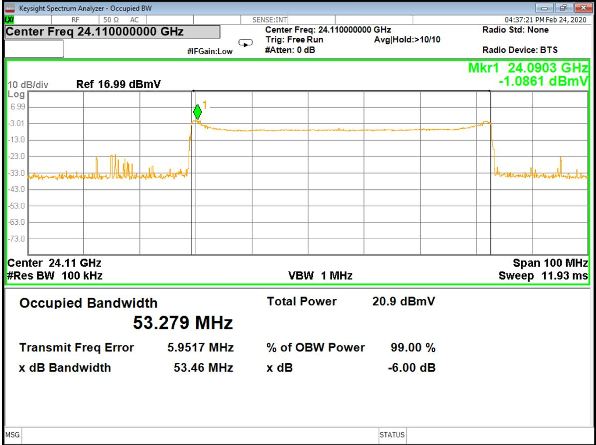
**Figure 40 – Occupied Bandwidth, Mid channel (48 MHz)**
