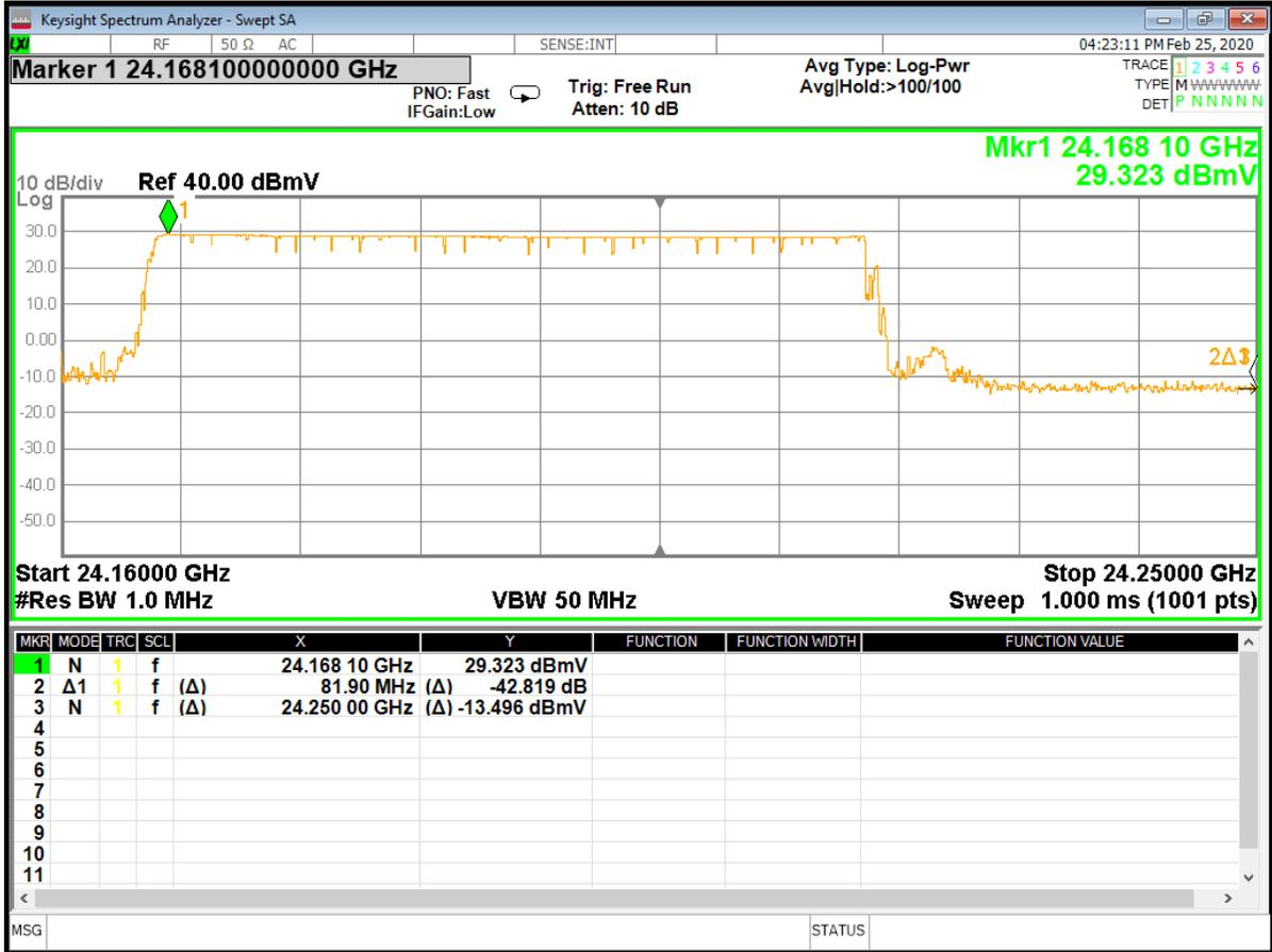
**Figure 33 - Higher Band Edge (48 MHz) (swept frequency), 24.25 GHz**
