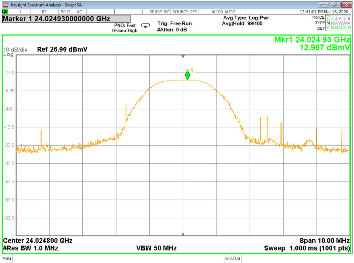
Figure 21 - Analyzer Measurement – Fundamental, Low Channel (Single Frequency)
