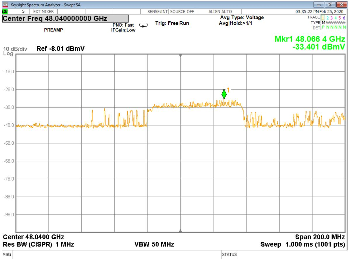
**Figure 4 - Analyzer Measurement – 2<sup>nd</sup> Harmonic, Low Channel (24 MHz) (swept frequency)**
