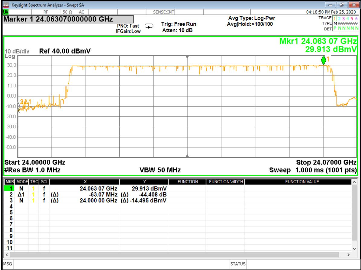
Figure 32 – Lower Band Edge (48 MHz) (swept frequency), 24.00 GHz
