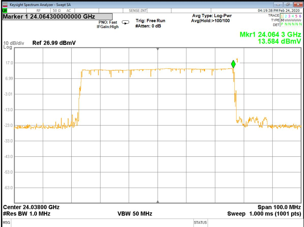
Figure 12 - Analyzer Measurement – Fundamental, Low Channel (48 MHz) (swept frequency)
