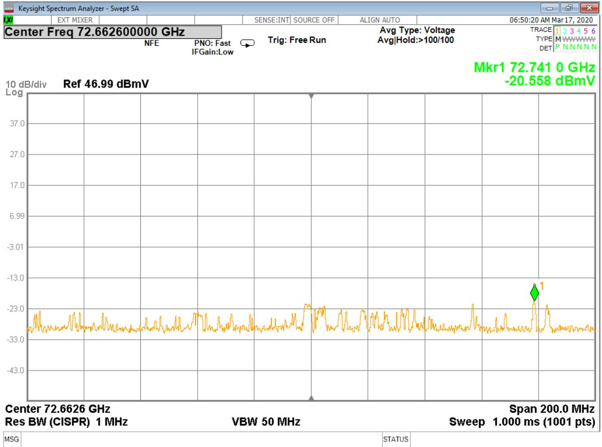
**Figure 29 - Analyzer Measurement – 3<sup>rd</sup> Harmonic, High Channel (Single Frequency)**
