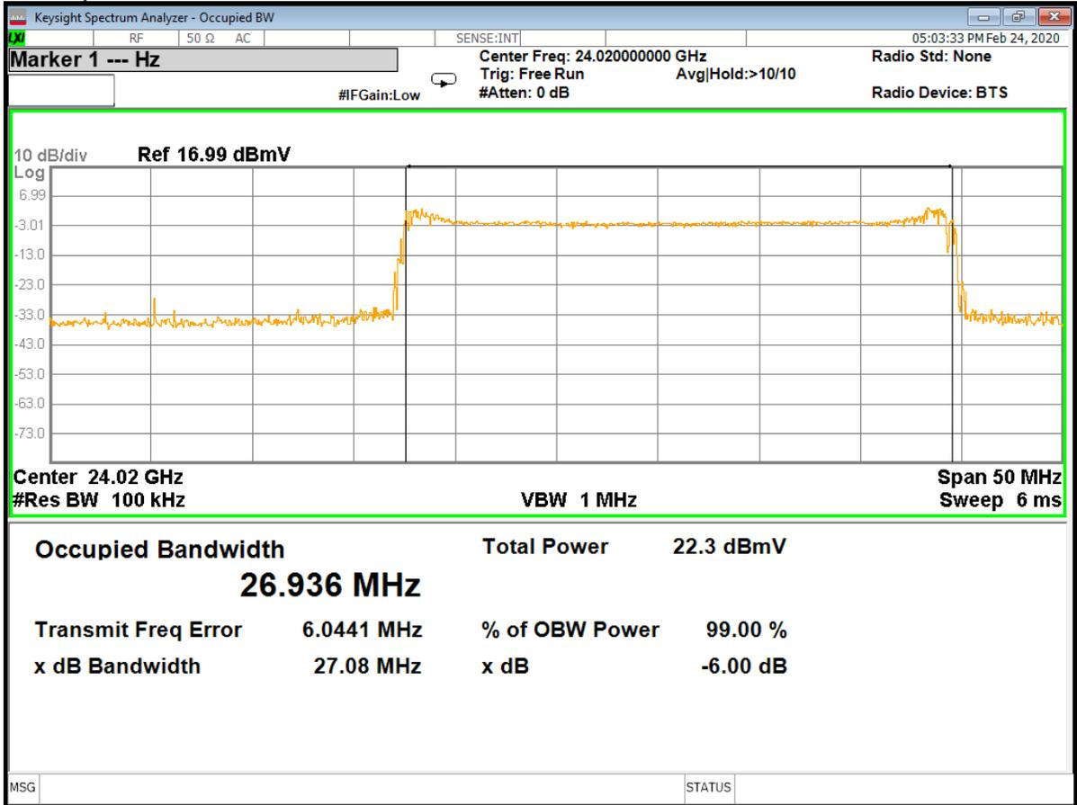
Figure 36 – Occupied Bandwidth, Low channel (24 MHz)
