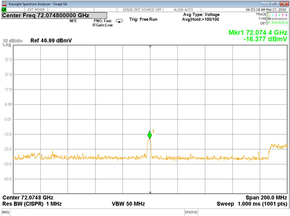
**Figure 23 - Analyzer Measurement – 3<sup>rd</sup> Harmonic, Low Channel (Single Frequency)**
