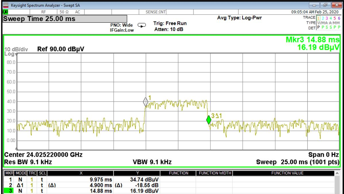
Figure 1 - On time / pulse width = 4.9 ms
