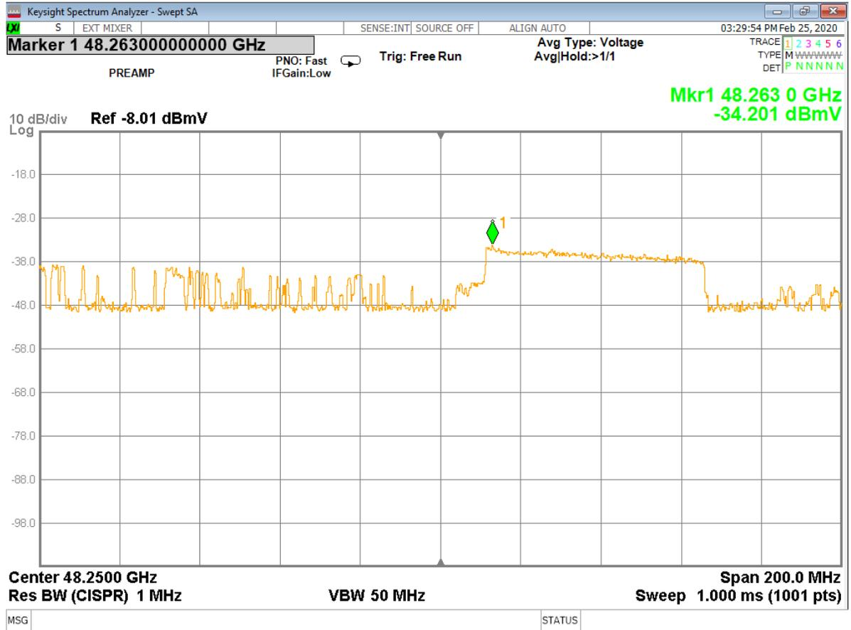
**Figure 7 - Analyzer Measurement – 2<sup>nd</sup> Harmonic, Mid Channel (24 MHz) (swept frequency)**
