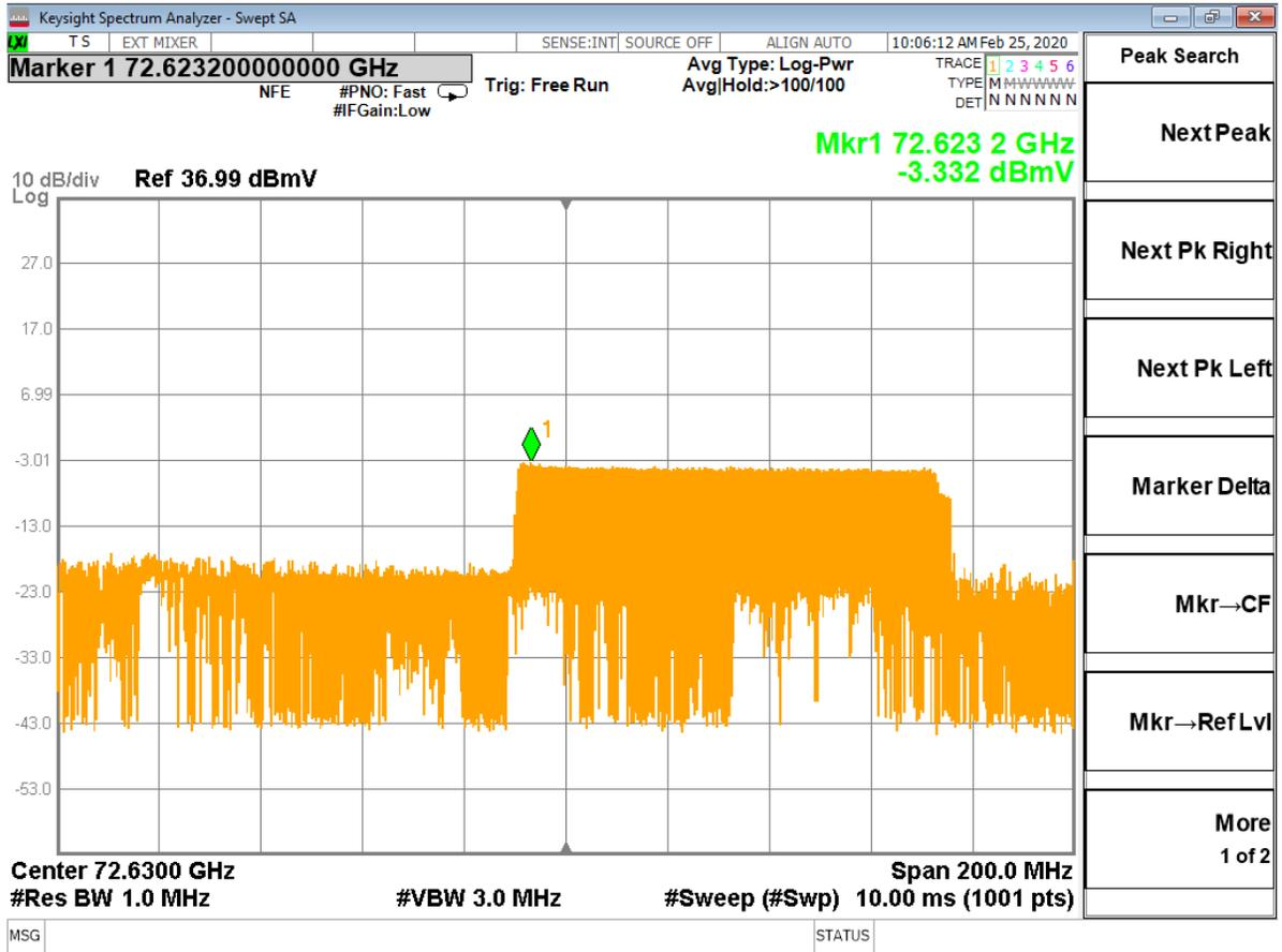
Figure 11 - Analyzer Measurement – 3<sup>rd</sup> Harmonic, High Channel (24 MHz) (swept frequency)
