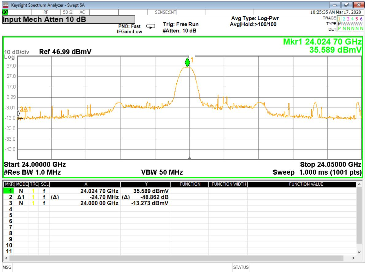
**Figure 34 – Lower Band Edge (Single Frequency), 24.00 GHz**
