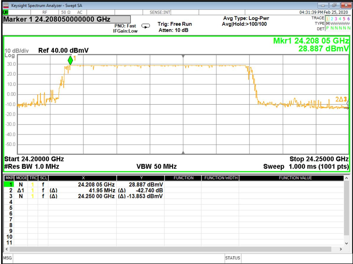
Figure 31 - Higher Band Edge (24 MHz) (swept frequency), 24.00 GHz
