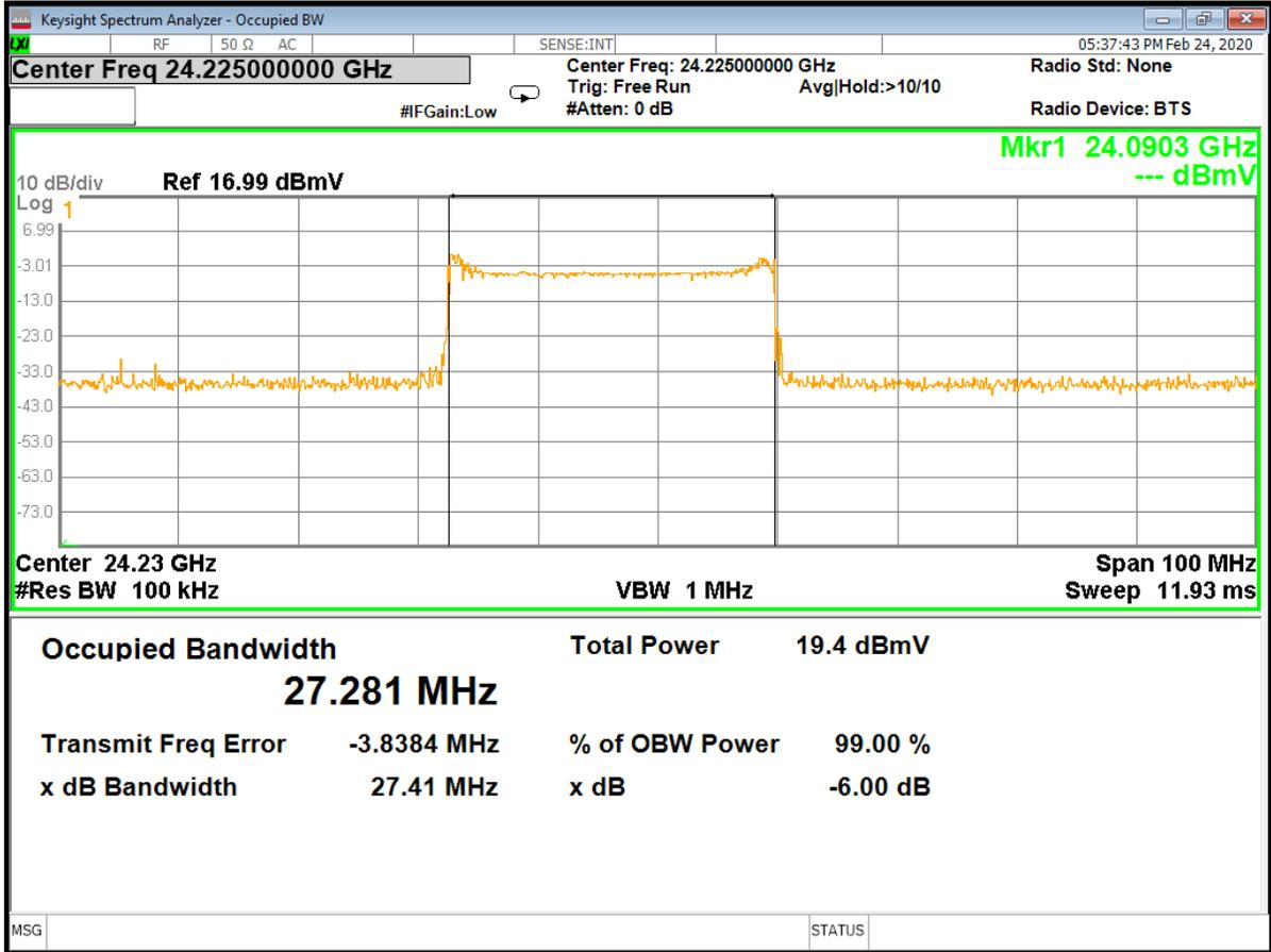
**Figure 38 – Occupied Bandwidth, High channel (24 MHz)**
