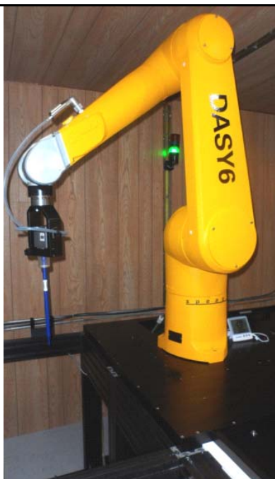
DASY 6 SAR System with SAM Phantom
