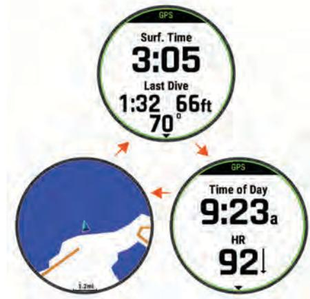
**Surface interval screen:** Displays the current surface interval time, as well as the elapsed time, maximum depth, and temperature for your last apnea dive.
