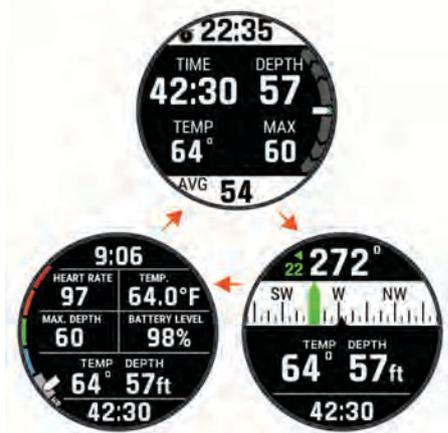
**Dive stopwatch:** Displays the bottom time stopwatch; current, maximum, and average depth; and rate of ascent or descent (*Using the Dive Stopwatch, page 6*).
