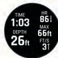
**In-dive screen:** Displays the information about the current dive, including the elapsed time, current and maximum depth, heart rate data, and rate ascent or descent.
