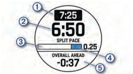
The device displays your target split pace ①, current split pace ②, completion progress for the split ③, distance remaining in the split ④, and overall time ahead or behind of your target pace ⑤.
