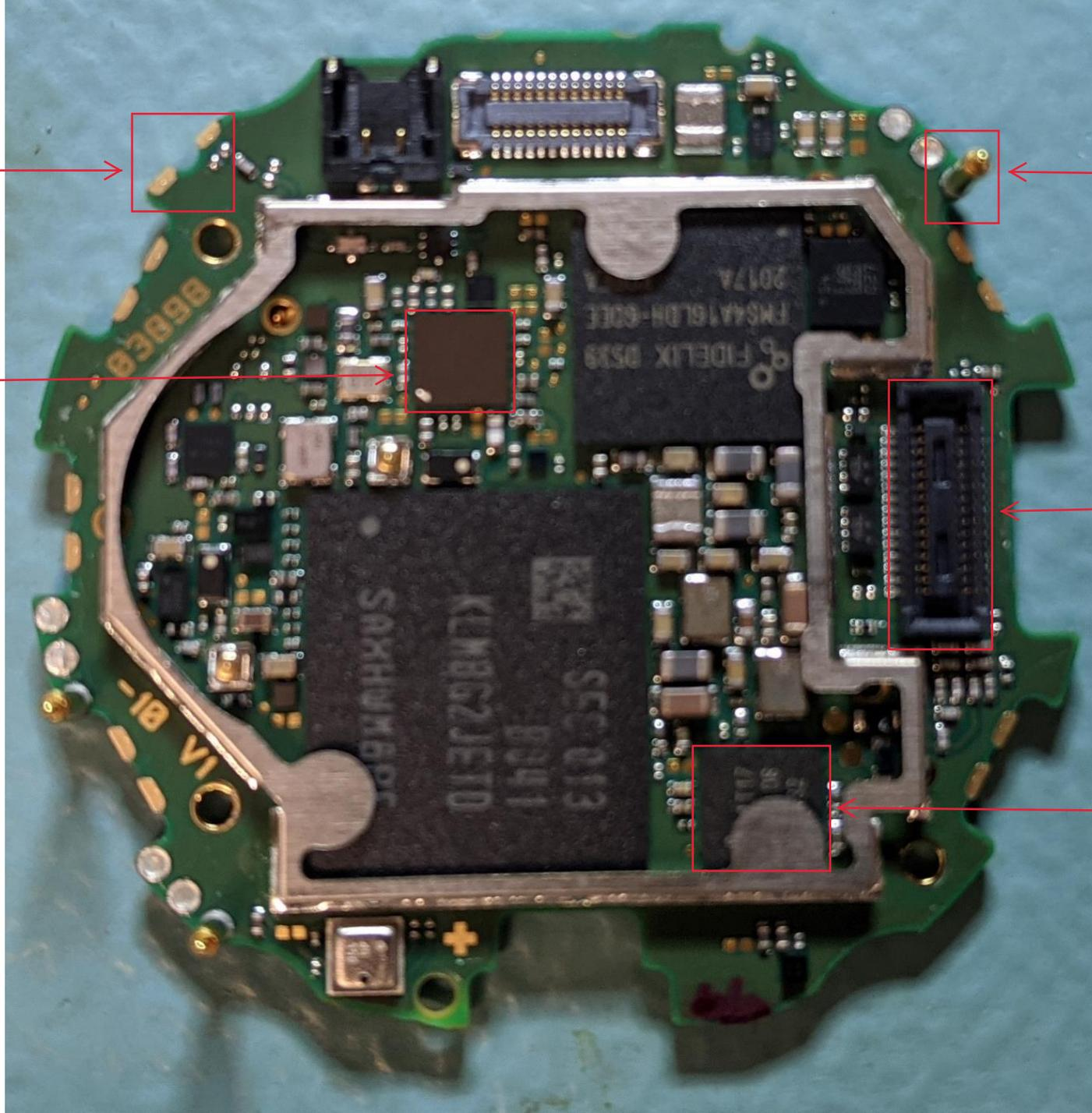
PCB bottom side shield removed
