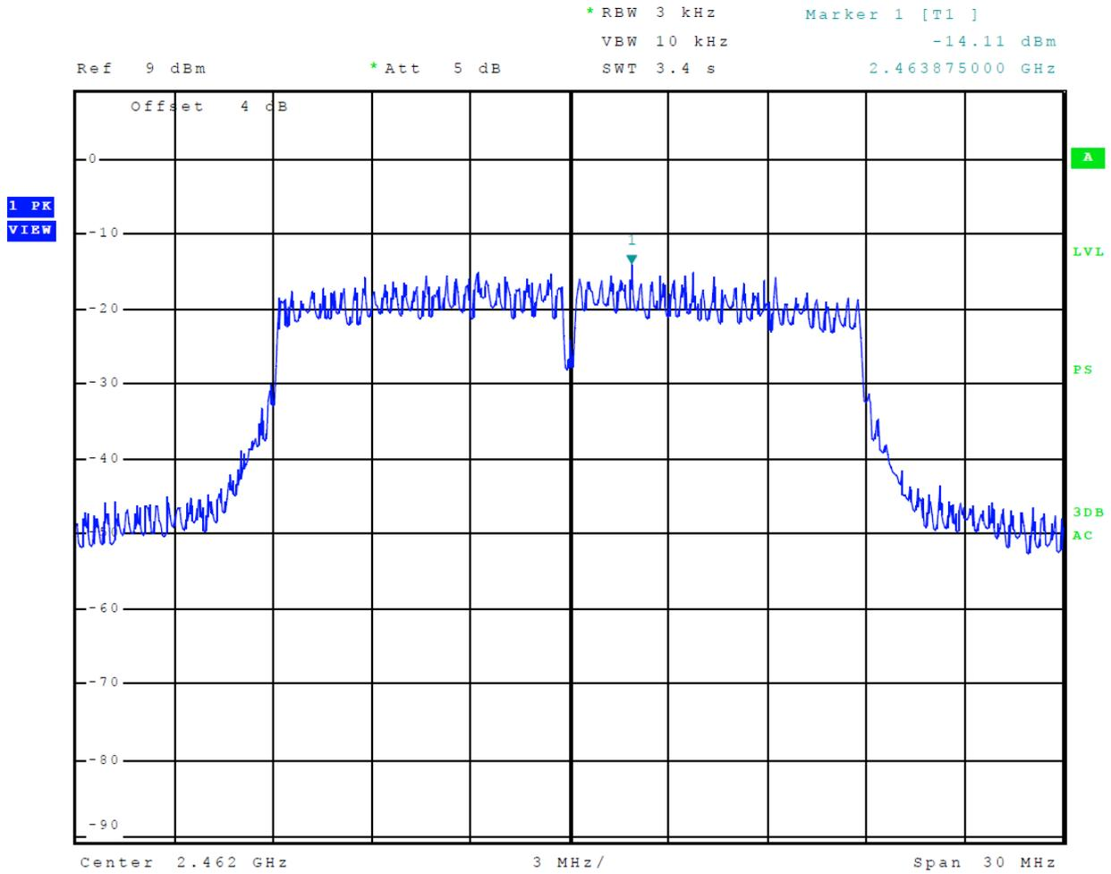
**Figure 22 Plot of Transmitter Power Spectral Density Mode 8 802.11n**
