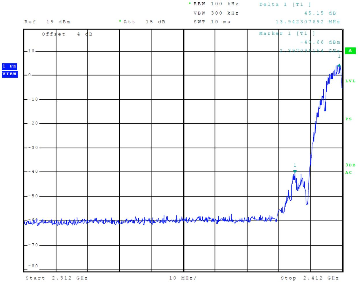
**Figure 8 Plot of Transmitter Emissions Low Band Edge Mode 6 802.11b**
