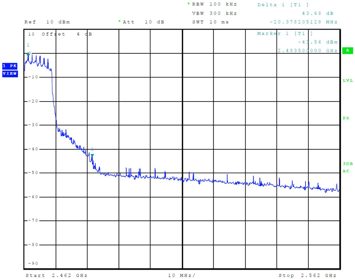
**Figure 13 Plot of Transmitter Emissions High Band Edge Mode 8 802.11n**
