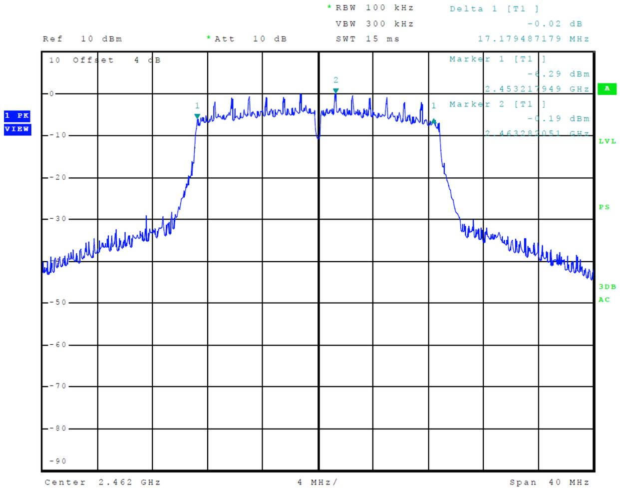
**Figure 18 Plot of 6-dB Occupied Bandwidth Mode 8 802.11n**
