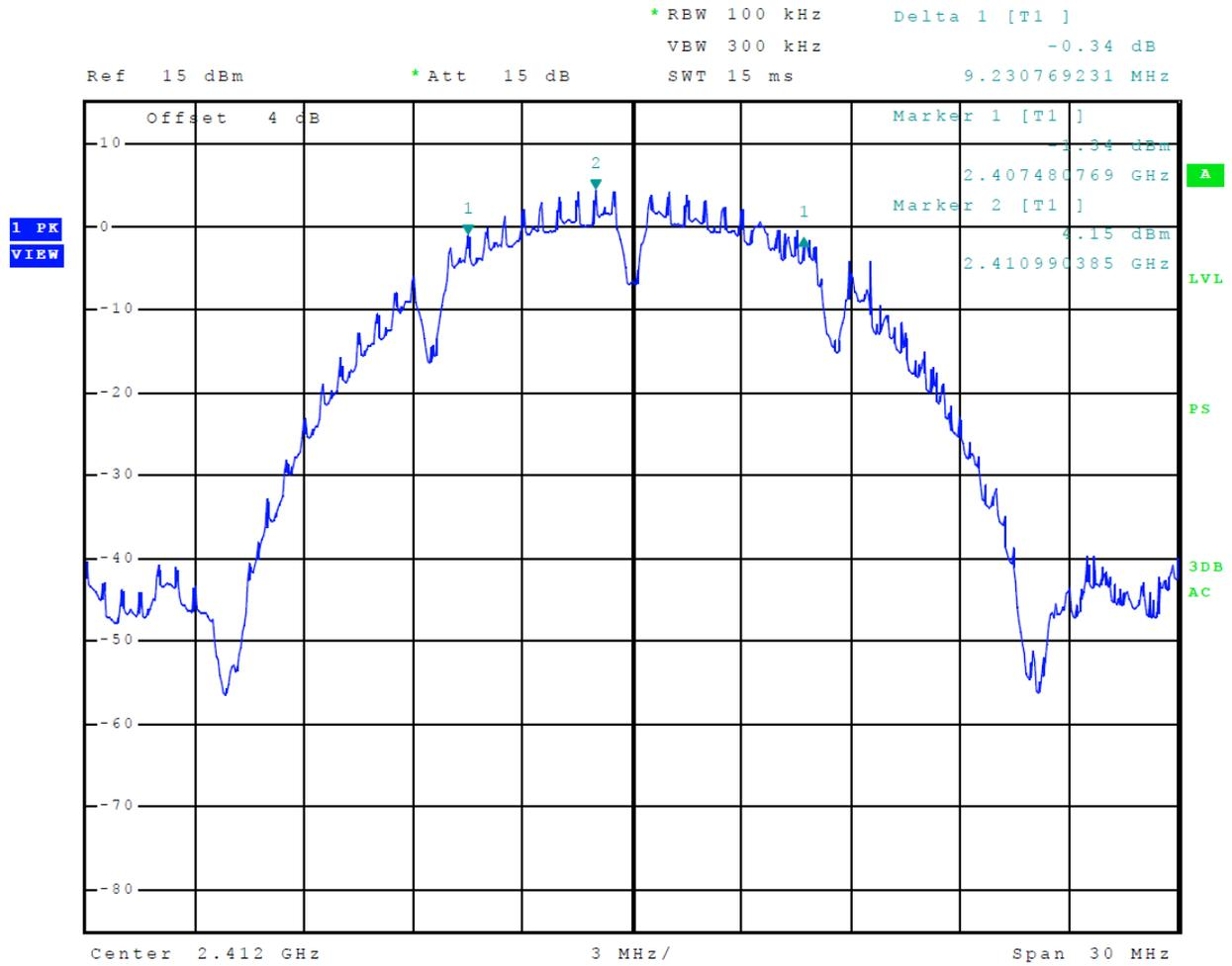
**Figure 14 Plot of 6-dB Occupied Bandwidth Mode 6 802.11b**
