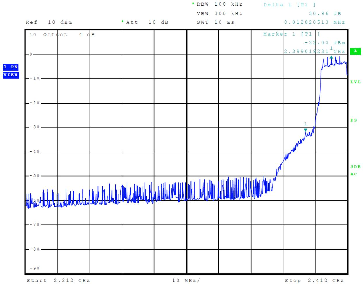
**Figure 9 Plot of Transmitter Emissions Low Band Edge Mode 7 802.11g**
