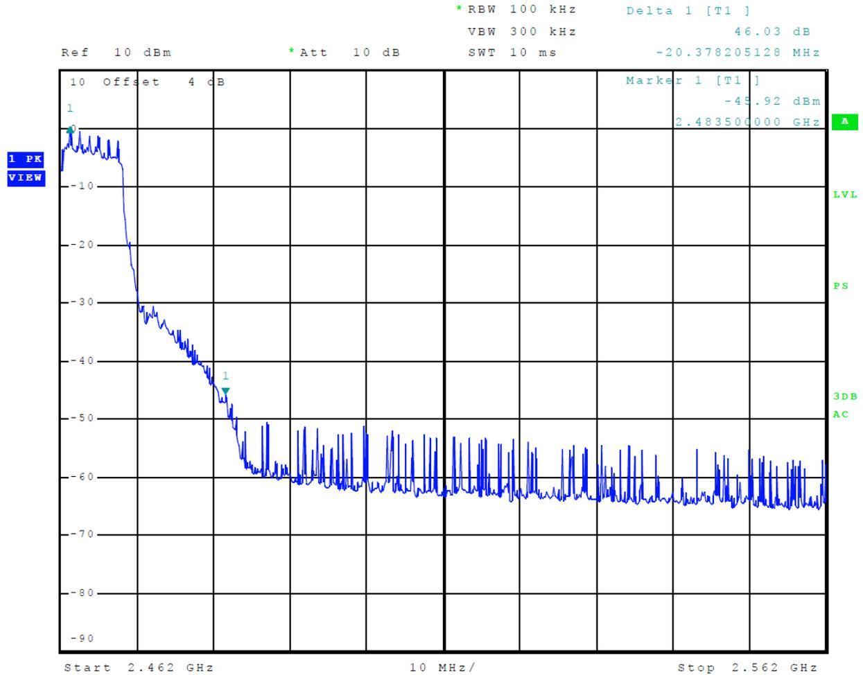
**Figure 12 Plot of Transmitter Emissions High Band Edge Mode 7 802.11g**
