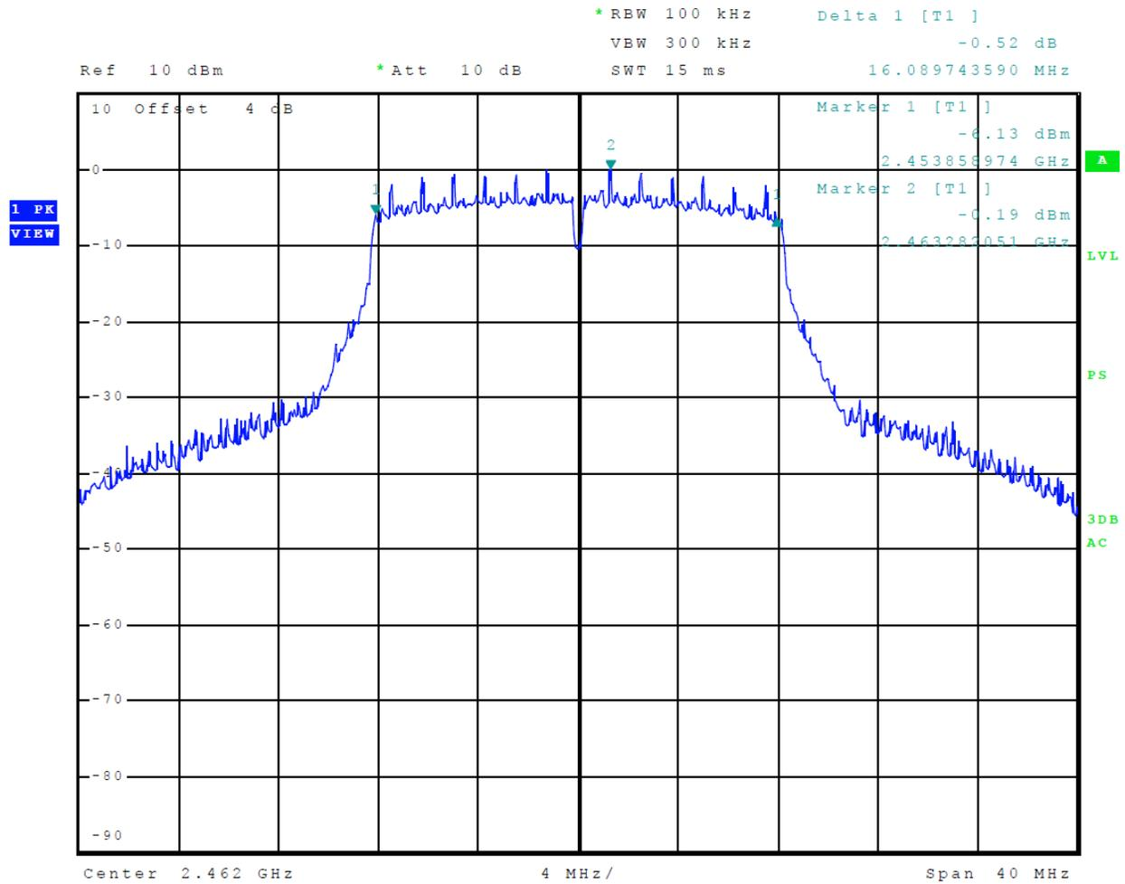
**Figure 16 Plot of 6-dB Occupied Bandwidth Mode 7 802.11g**
