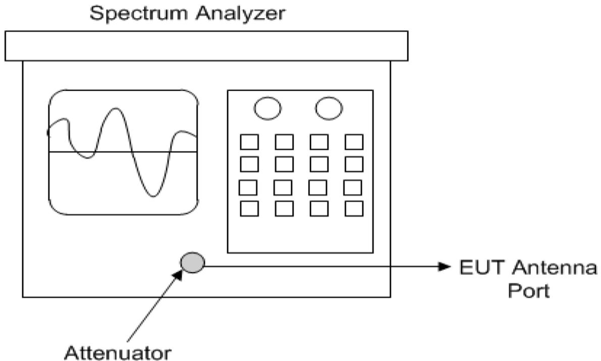
**Diagram 4 Test arrangement for Antenna Port Conducted emissions**
