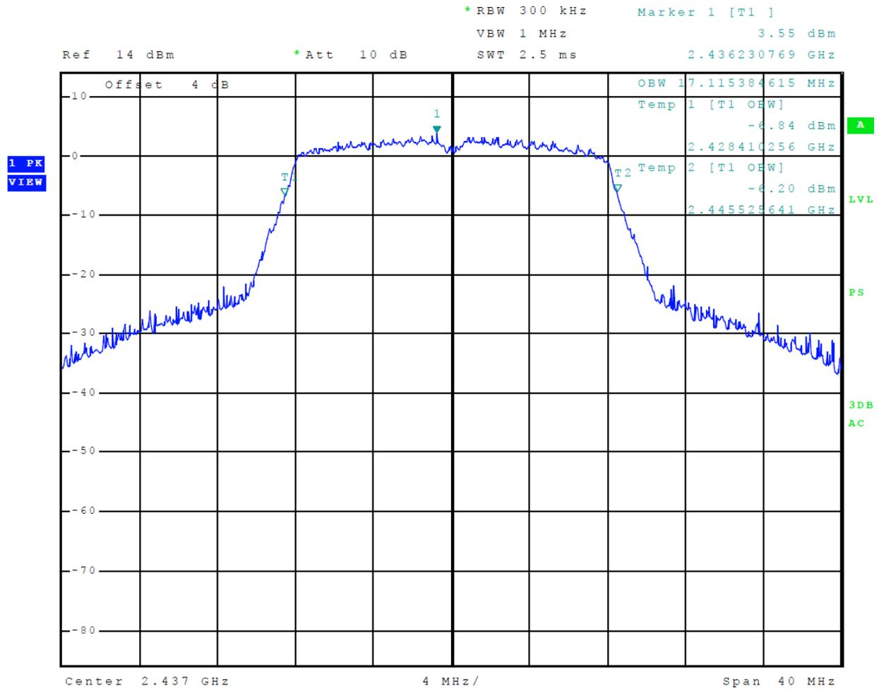
**Figure 17 Plot of 99% Occupied Bandwidth Mode 7 802.11g**
