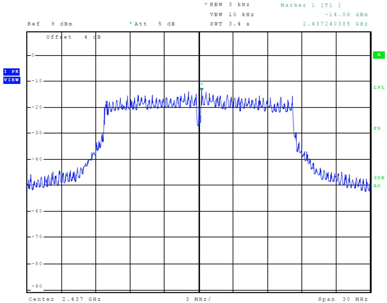
**Figure 21 Plot of Transmitter Power Spectral Density Mode 7 802.11g**
