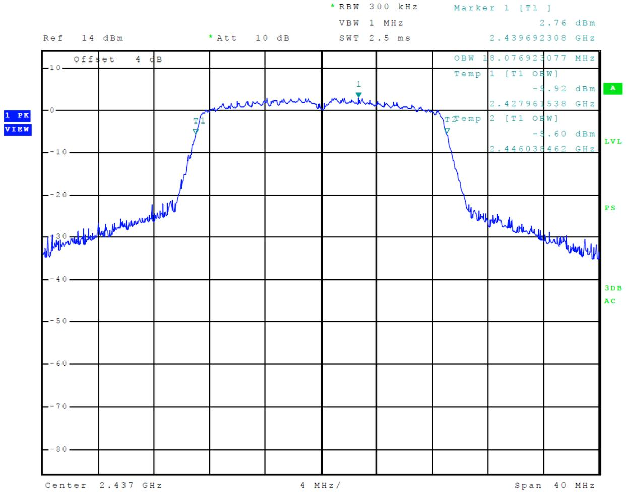
**Figure 19 Plot of 99% Occupied Bandwidth Mode 8 802.11n**
