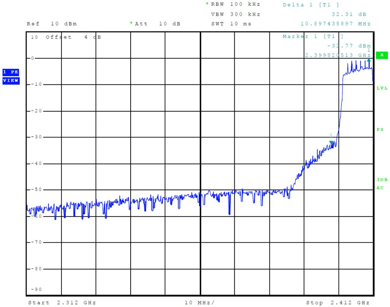
**Figure 10 Plot of Transmitter Emissions Low Band Edge Mode 8 802.11n**
