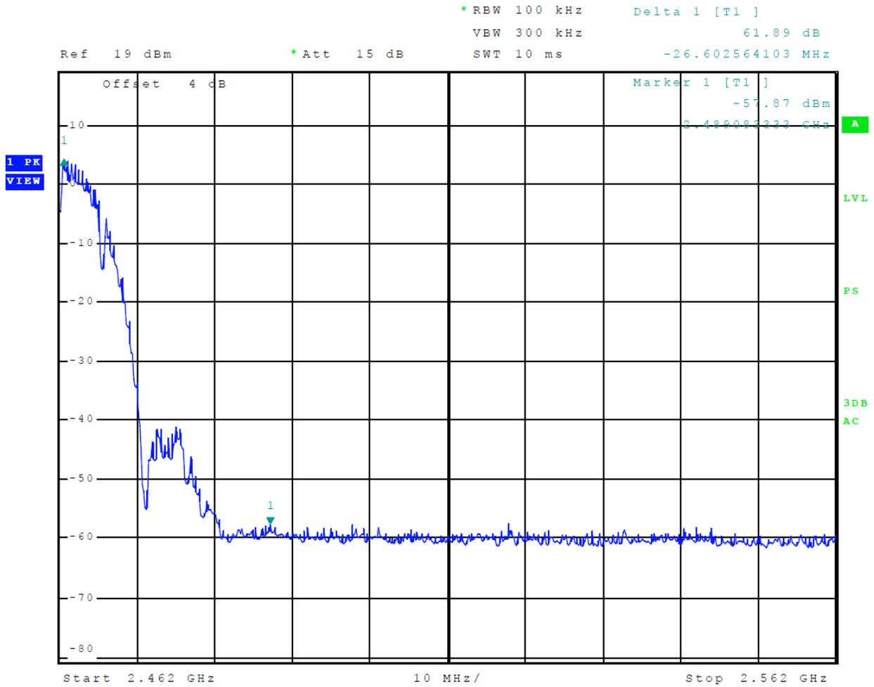
**Figure 11 Plot of Transmitter Emissions High Band Edge Mode 6 802.11b**
