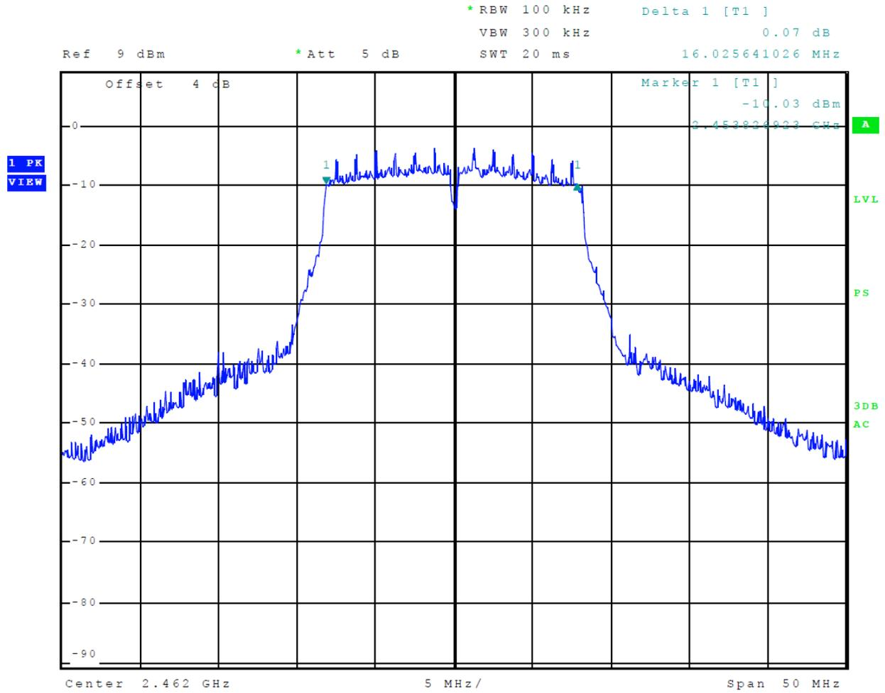
**Figure 17 Plot of 6-dB Occupied Bandwidth Mode 4 802.11g**
