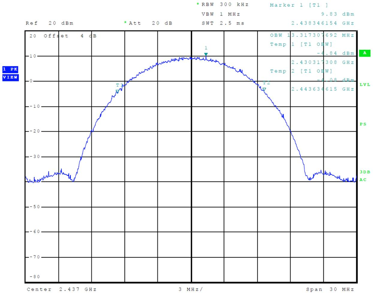
**Figure 16 Plot of 99% Occupied Bandwidth Mode 3 802.11b**
