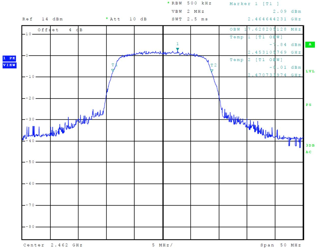
**Figure 18 Plot of 99% Occupied Bandwidth Mode 4 802.11g**
