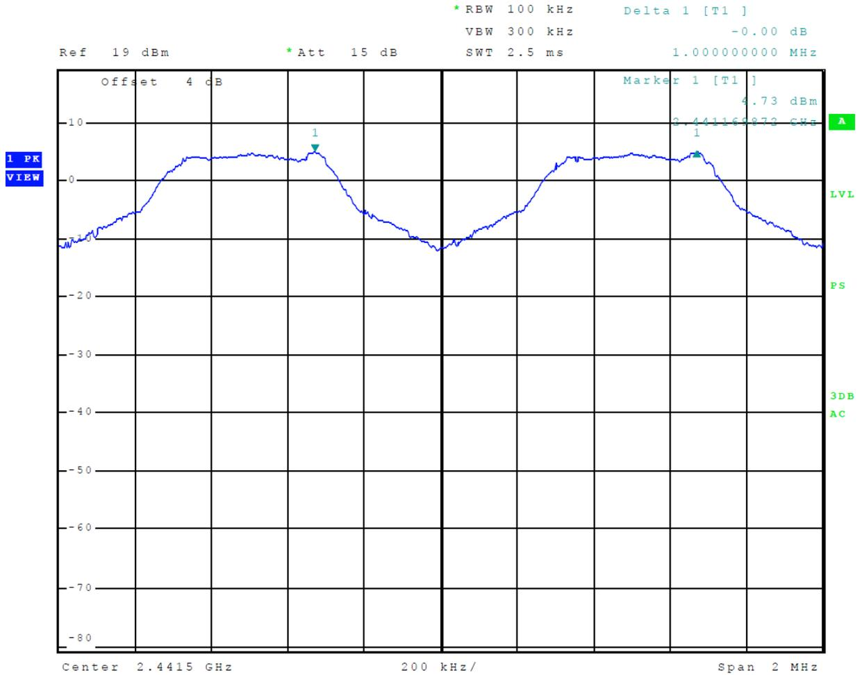
**Figure 12 Plot of Channel Separation BT BR (GMSK)**
