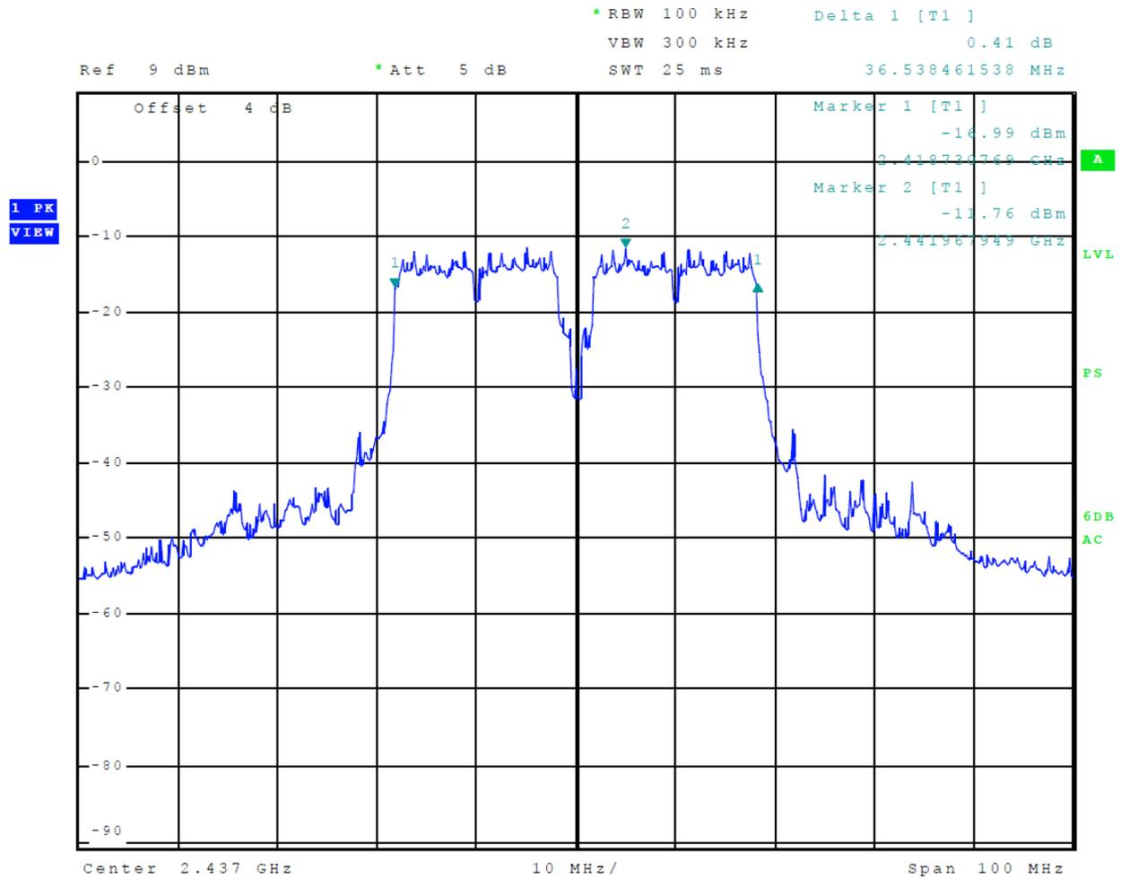
**Figure 38 Plot of 6-dB Occupied Bandwidth (Mode 8, 802.11n40)**
