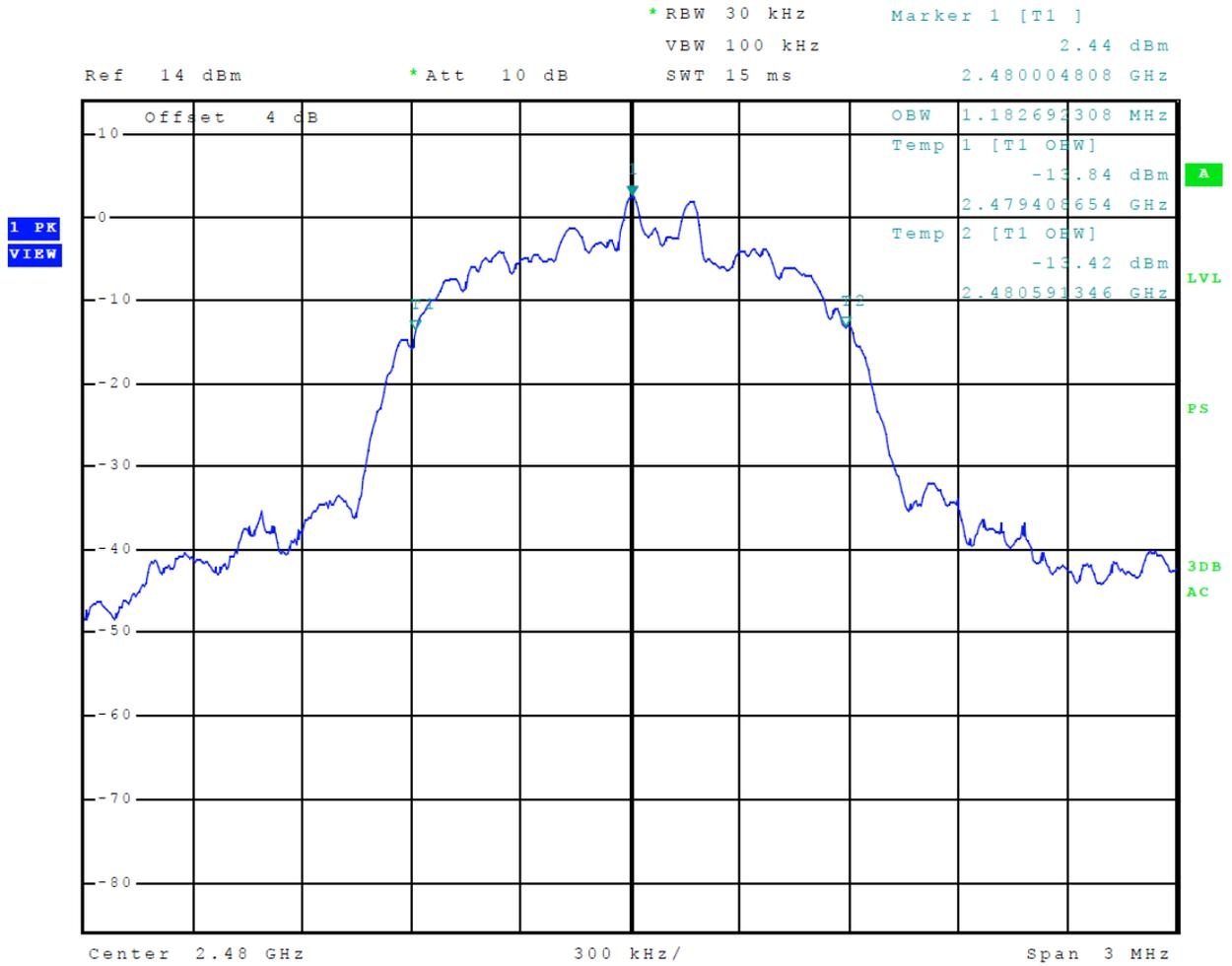
**Figure 29 Plot of 99% Occupied Bandwidth (Mode 3, 3EDR)**
