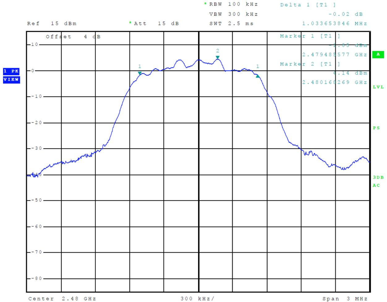
**Figure 28 Plot of 6-dB Occupied Bandwidth (Mode 3, 3EDR)**
