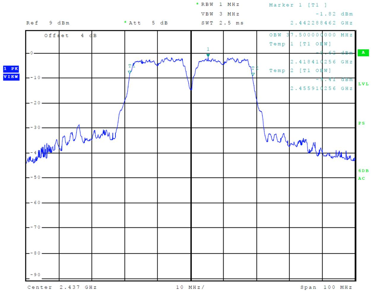
**Figure 39 Plot of 99% Occupied Bandwidth (Mode 8, 802.11n40)**
