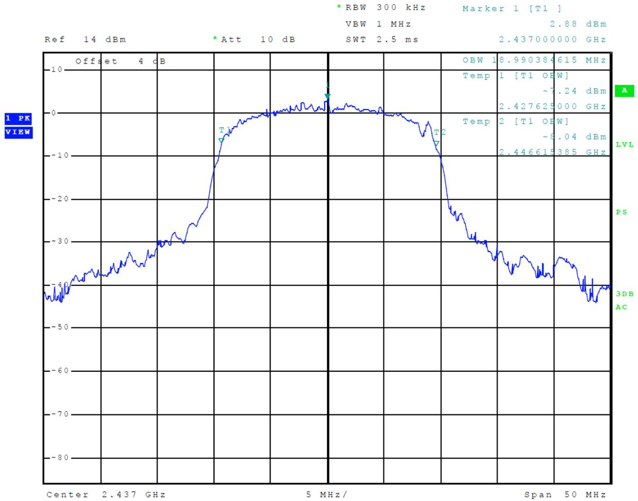
**Figure 35 Plot of 99% Occupied Bandwidth (Mode 6, 802.11g)**
