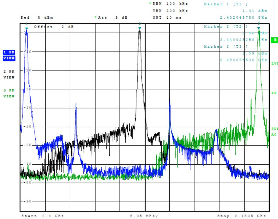
**Figure 17 Plot of Transmitter Emissions (Mode 2 Operation In 2402-2480 MHz)**
