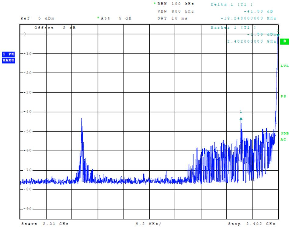
Figure 15 Plot of Transmitter Emissions (Mode 1 Low Band Edge)
