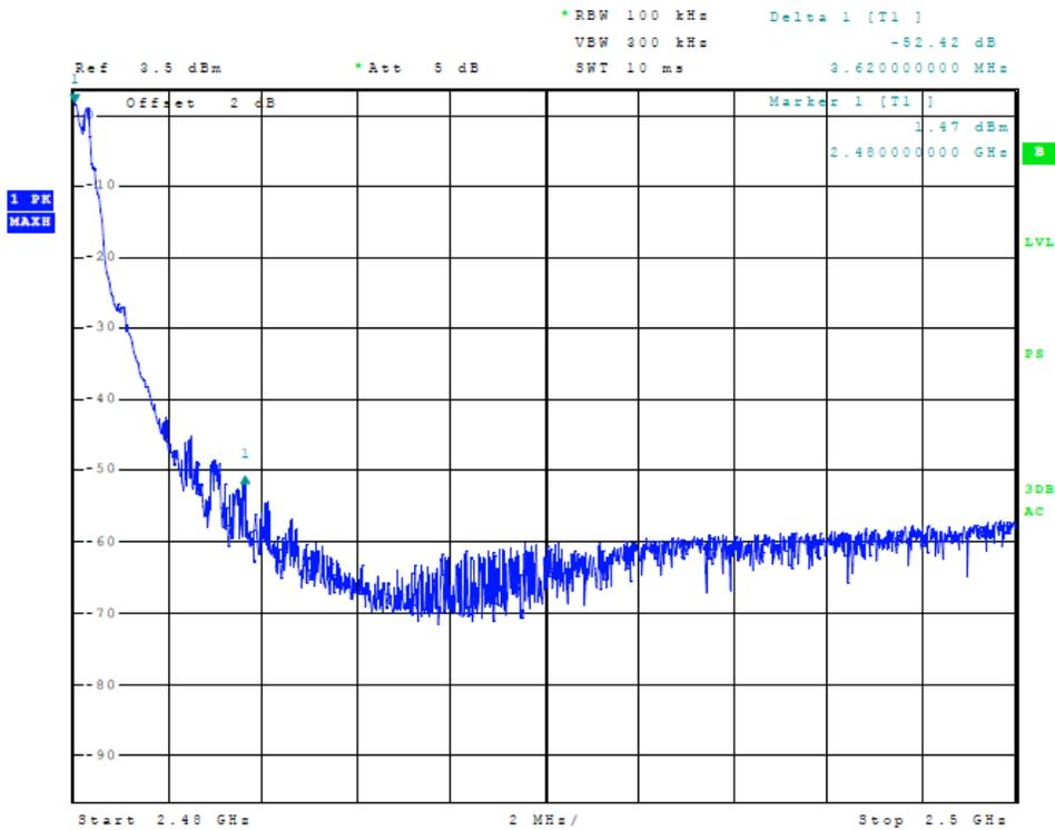
Figure 20 Plot of Transmitter Emissions (Mode 2 High Band Edge)
