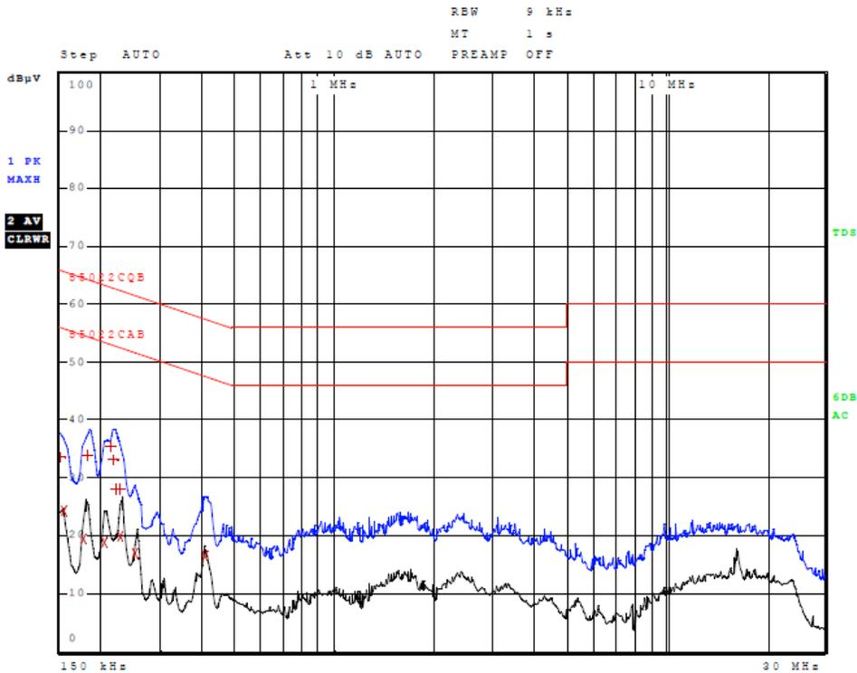
**Figure 7 AC Line Conducted emissions of EUT line 1 (EUT AC Adapter Configuration #5)**
