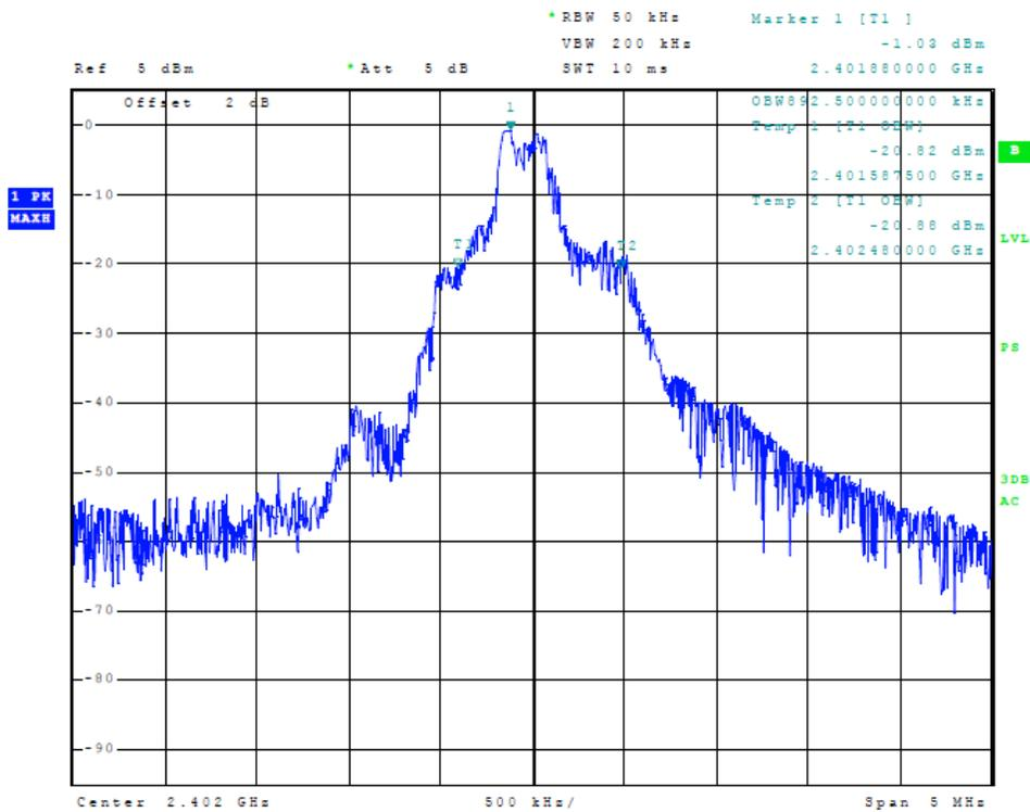
Figure 14 Plot of Transmitter Emissions (Mode 1 2402-2479 MHz, 99% Occupied Bandwidth)
