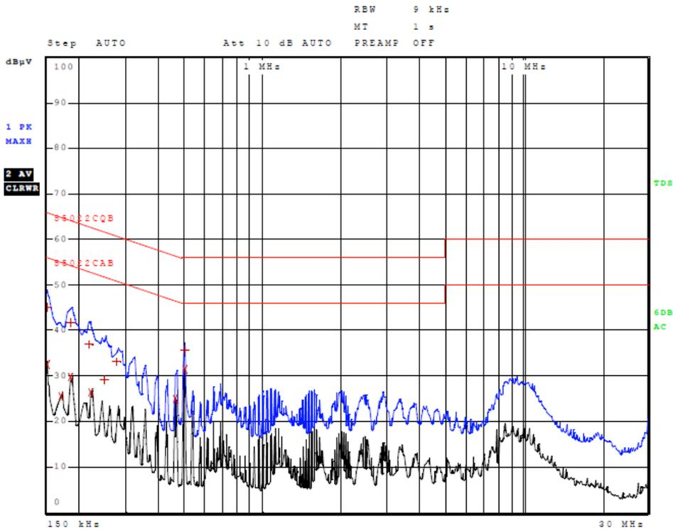
Figure 4 AC Line Conducted emissions of EUT line 2 (EUT AC Adapter Configuration #3)
