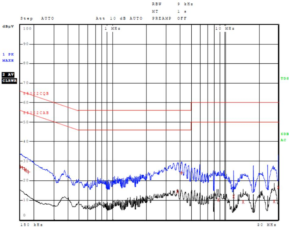
Figure 11 AC Line Conducted emissions of EUT line 1 (EUT AC Adapter Configuration #7)
