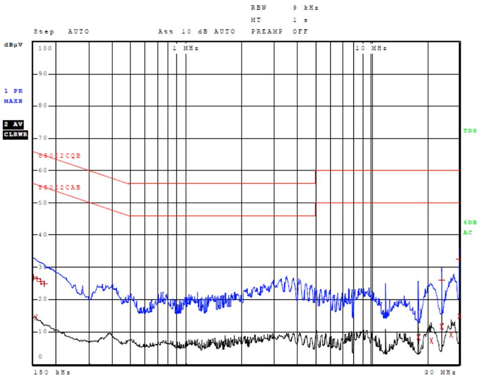
Figure 12 AC Line Conducted emissions of EUT line 2 (EUT AC Adapter Configuration #7)
