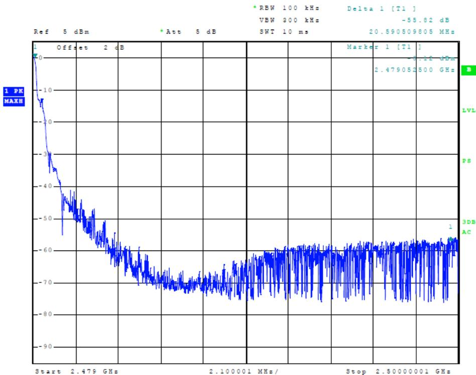
Figure 16 Plot of Transmitter Emissions (Mode 1 High Band Edge)
