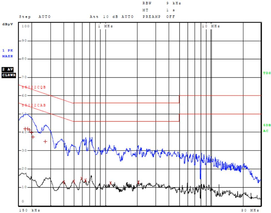
**Figure 9 AC Line Conducted emissions of EUT line 1 (EUT AC Adapter Configuration #6)**
