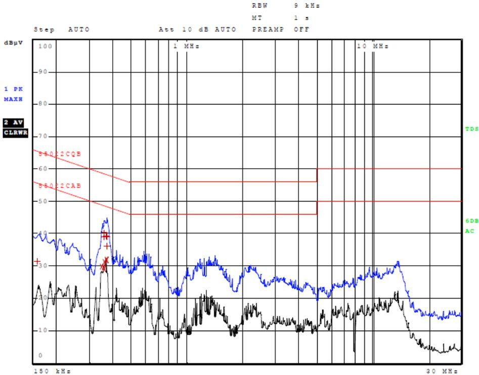
Figure 5 AC Line Conducted emissions of EUT line 1 (EUT AC Adapter Configuration #4)
