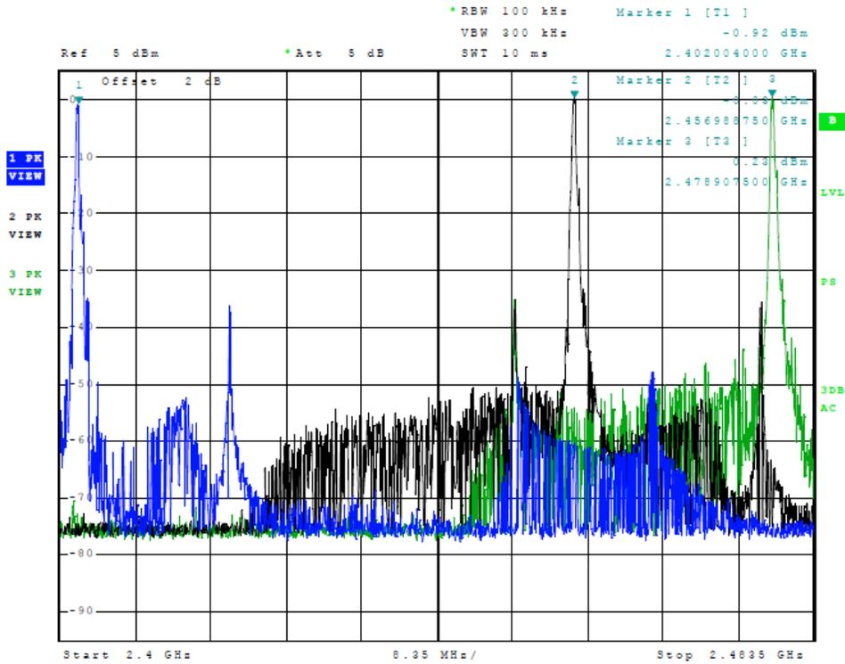
Figure 13 Plot of Transmitter Emissions (Mode 1 Operation In 2402-2479 MHz)
