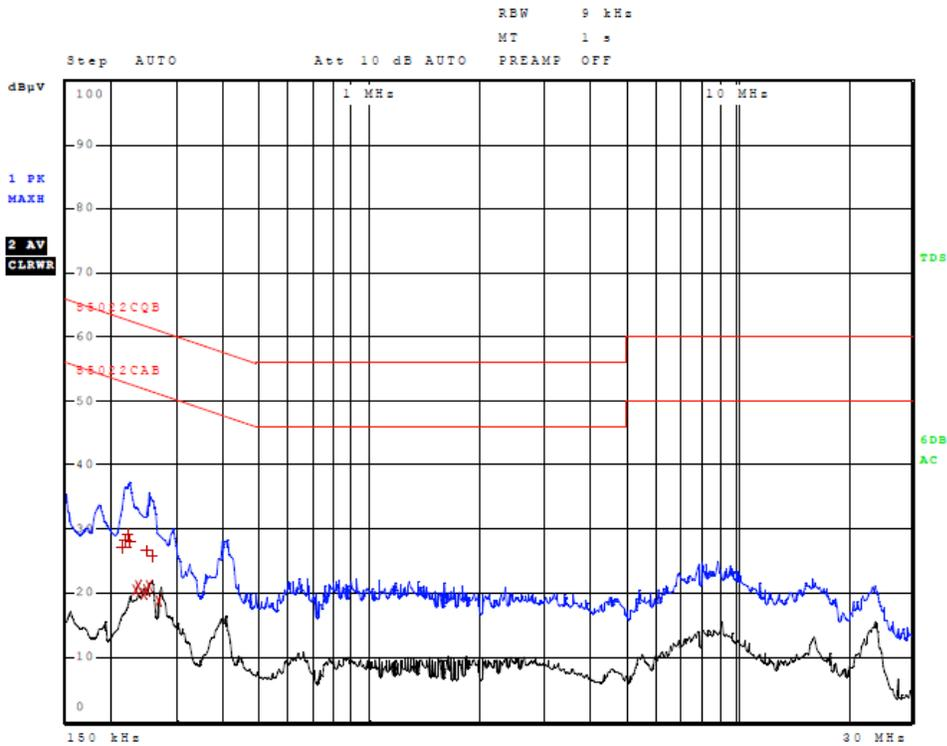
**Figure 8 AC Line Conducted emissions of EUT line 2 (EUT AC Adapter Configuration #5)**
