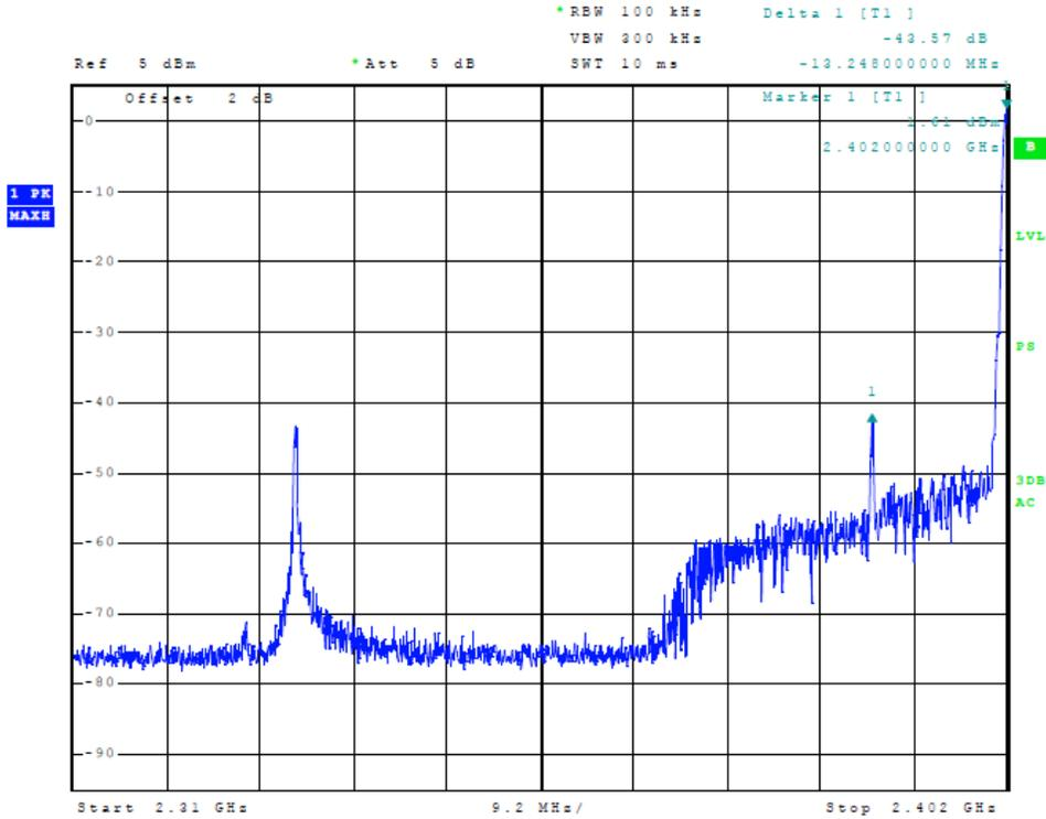
Figure 19 Plot of Transmitter Emissions (Mode 2 Low Band Edge)
