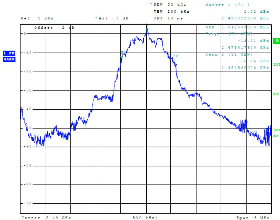
**Figure 18 Plot of Transmitter Emissions (Mode 2 2402-2480 MHz, 99% Occupied Bandwidth)**
