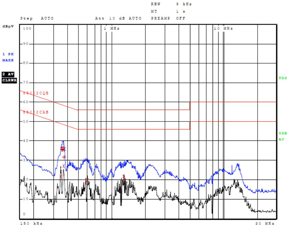
Figure 6 AC Line Conducted emissions of EUT line 2 (EUT AC Adapter Configuration #4)
