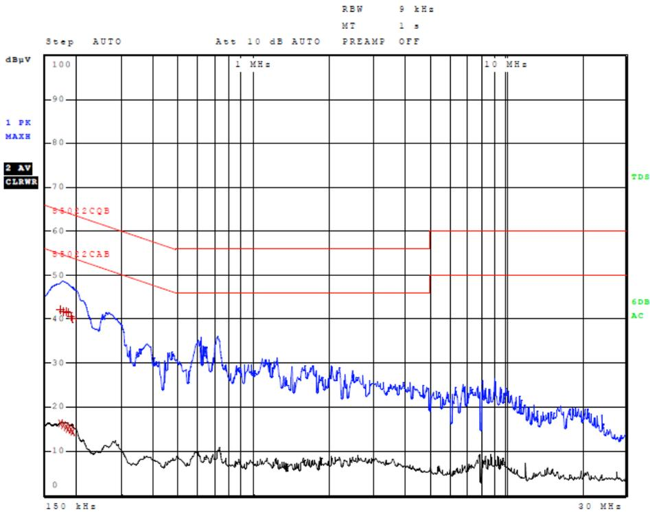
**Figure 10 AC Line Conducted emissions of EUT line 2 (EUT AC Adapter Configuration #6)**
