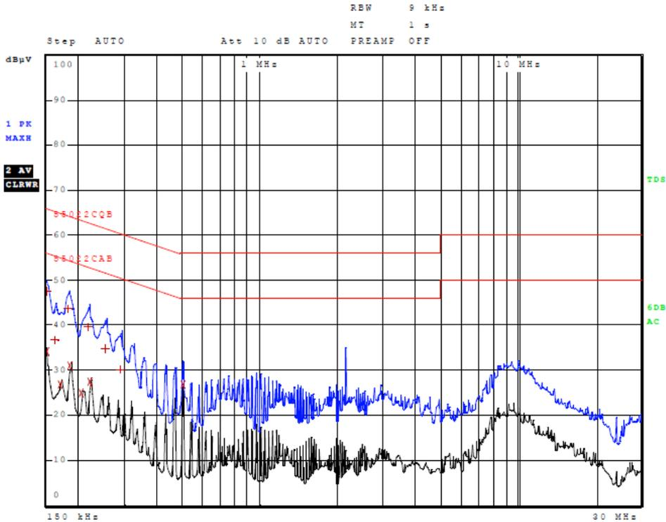
Figure 3 AC Line Conducted emissions of EUT line 1 (EUT AC Adapter Configuration #3)
