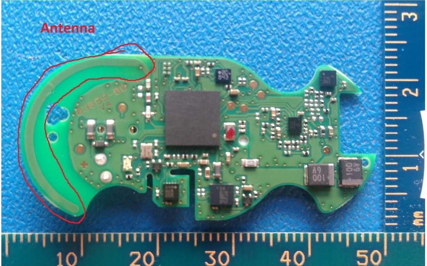
Figure E19.2 – Internal Photo – PCB Bottom
