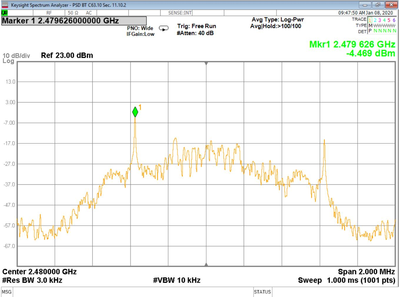
Figure 41 - Power Spectral Density, High Channel, BT EDR 2MB
