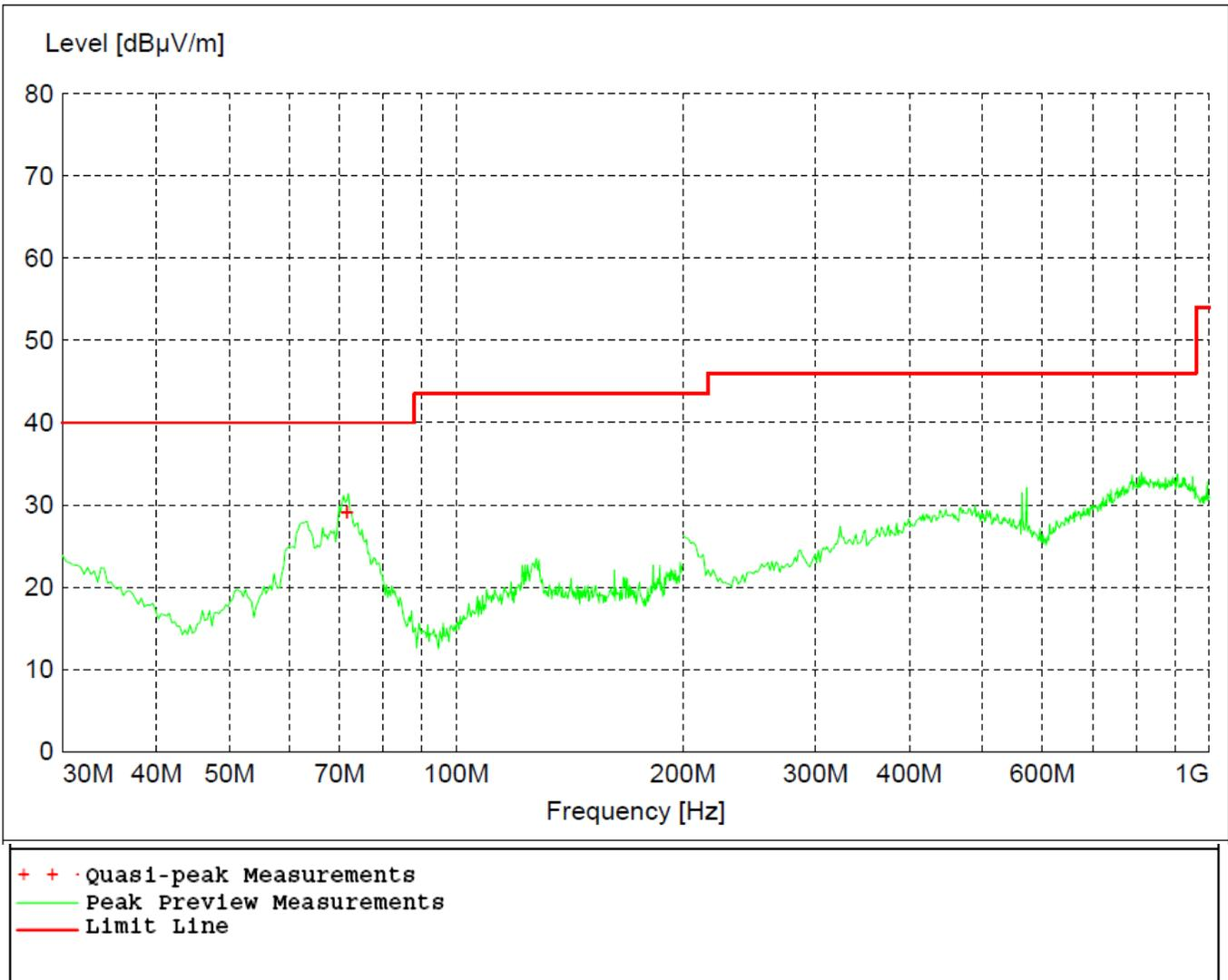
Figure 13 - Radiated Emissions Plot, GMSK
