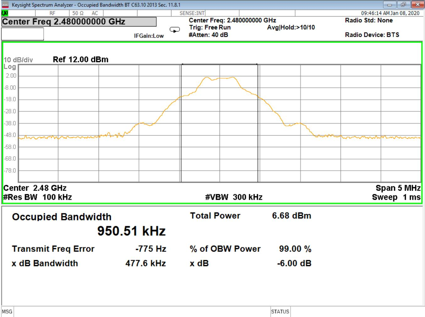
Figure 10 - Bandwidth, High Channel, BT BR (GFSK)
