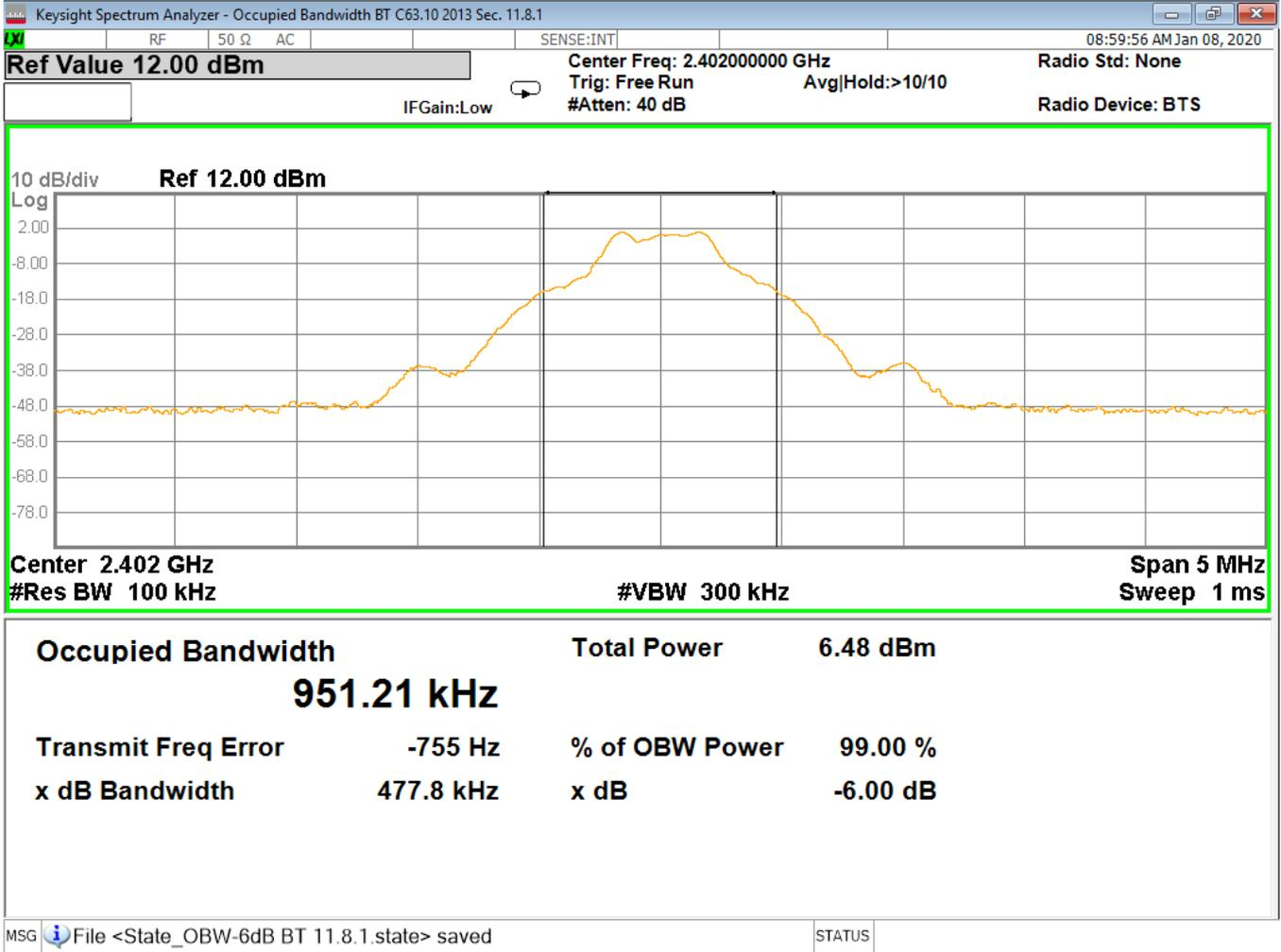
Figure 8 –Bandwidth, Low Channel, BT BR (GFSK)
