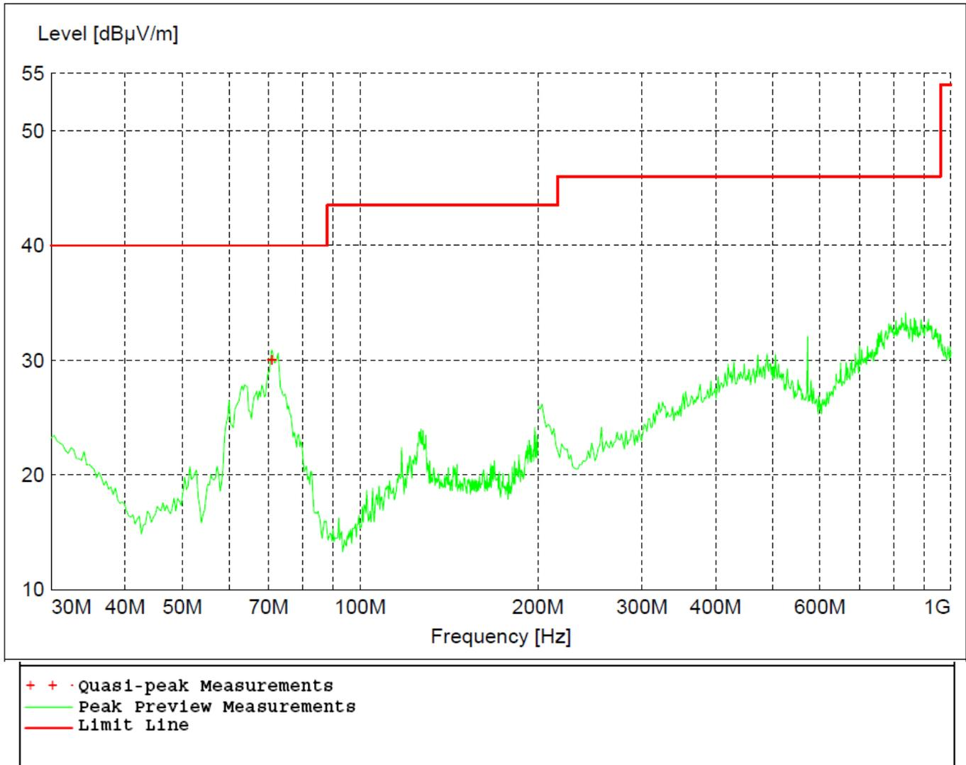
Figure 14 - Radiated Emissions Plot, GFSK
