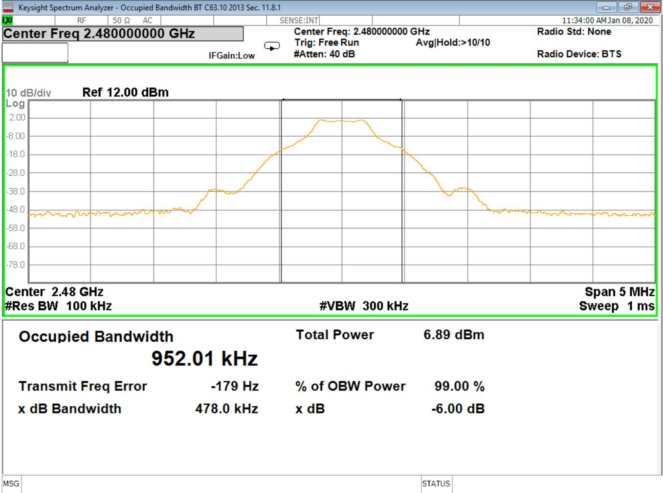
Figure 7 – Occupied Bandwidth, High Channel, GFSK
