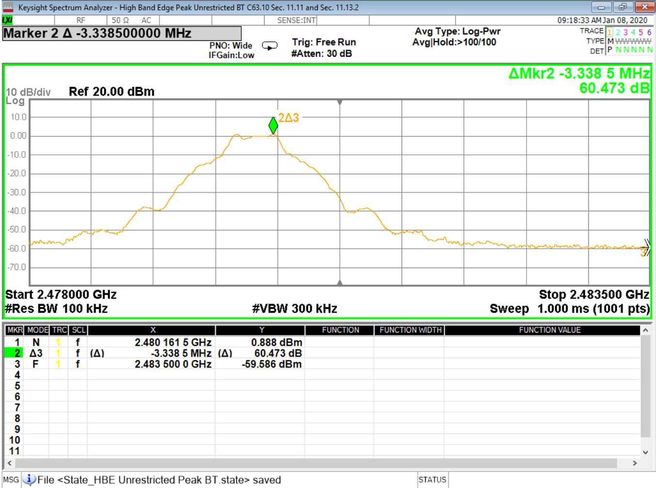
Figure 21 – Band Edge Measurement, High Channel, BTBR
