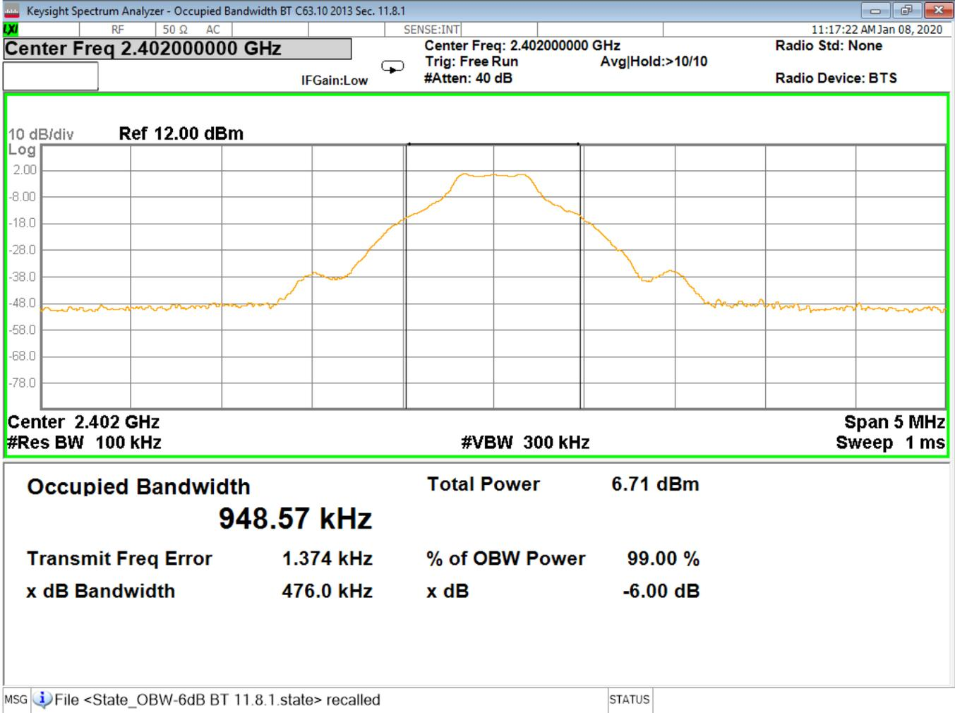
Figure 5 - Occupied Bandwidth, Low Channel, GFSK
