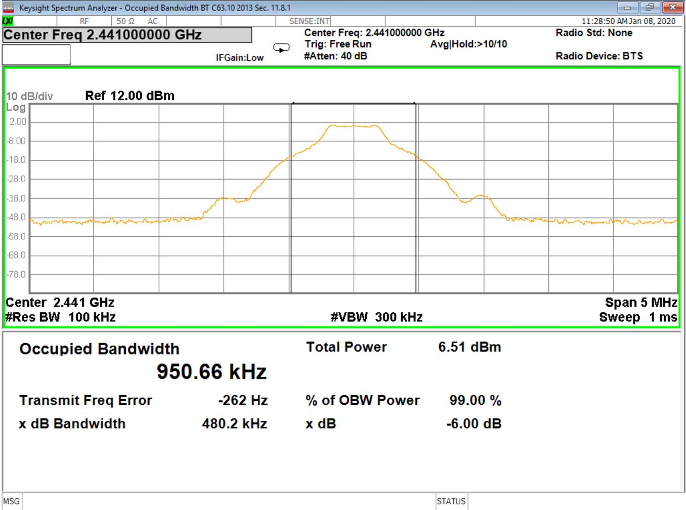
Figure 6 - Occupied Bandwidth, Mid Channel, GFSK
