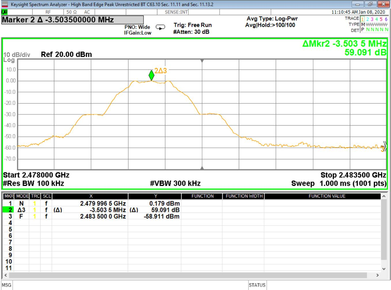
Figure 19 – Band Edge Measurement, High Channel, GMSK
