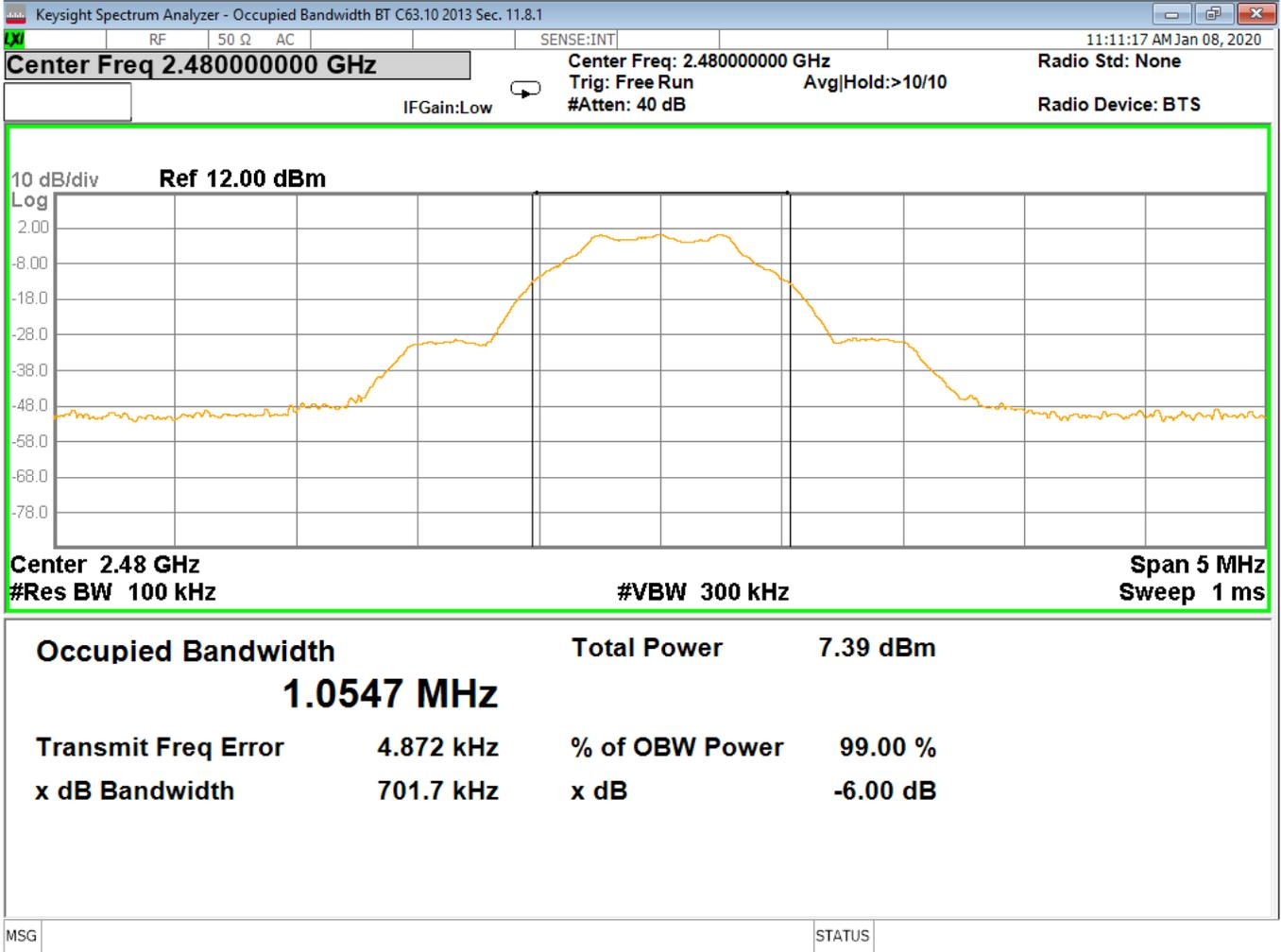
Figure 4 – Occupied Bandwidth, High Channel, GMSK
