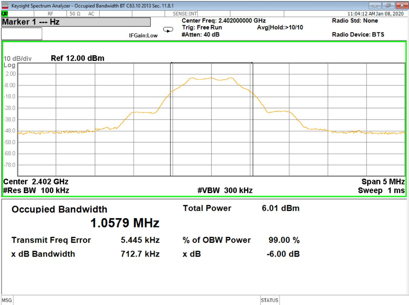
Figure 2 – Occupied Bandwidth, Low Channel, GMSK
