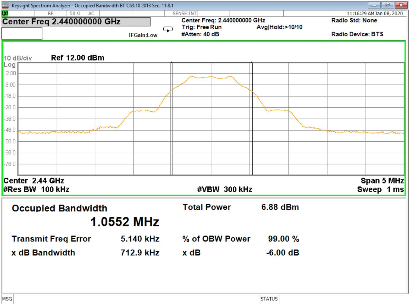
Figure 3 - Occupied Bandwidth, Mid Channel, GMSK
