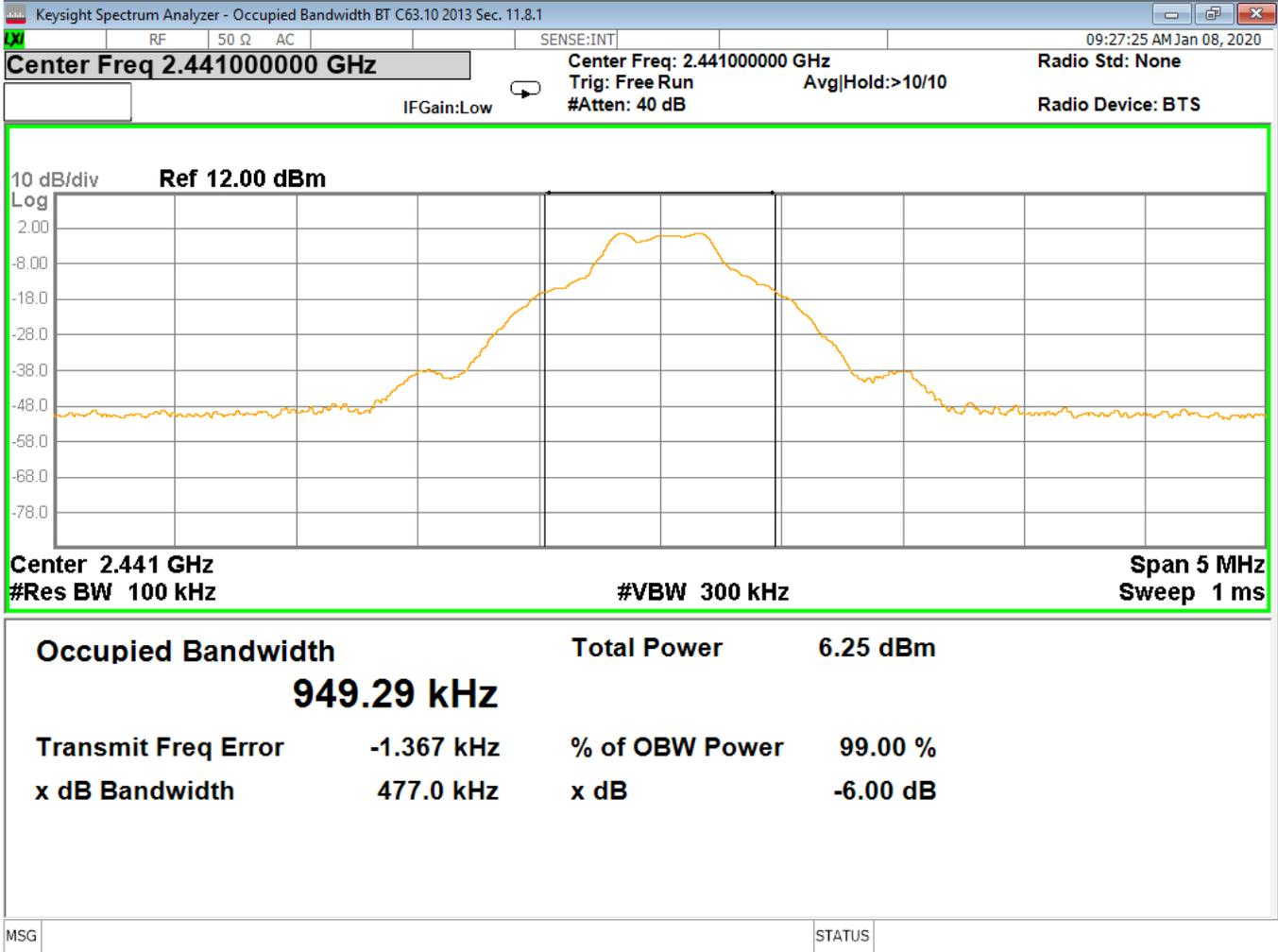
Figure 9 - Bandwidth, Mid Channel, BT BR (GFSK)
