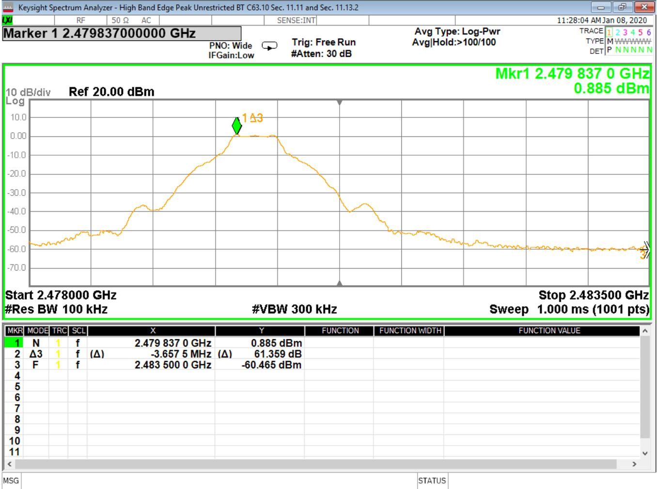
Figure 17 –Band Edge Measurement, High Channel, GFSK
