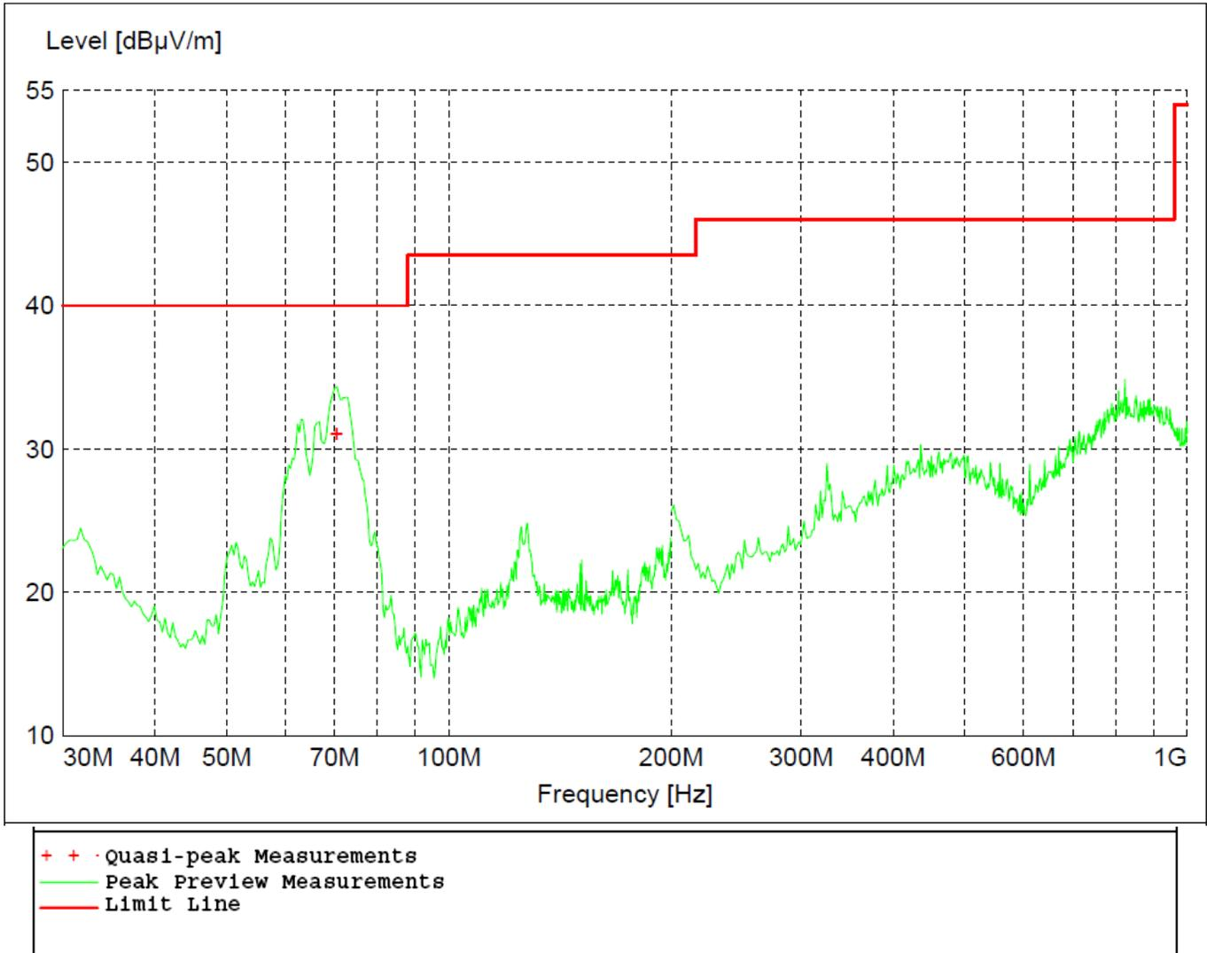
Figure 15 - Radiated Emissions Plot, BTBR
