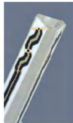
Figure 2.3 Probe Thick-Film Technique
