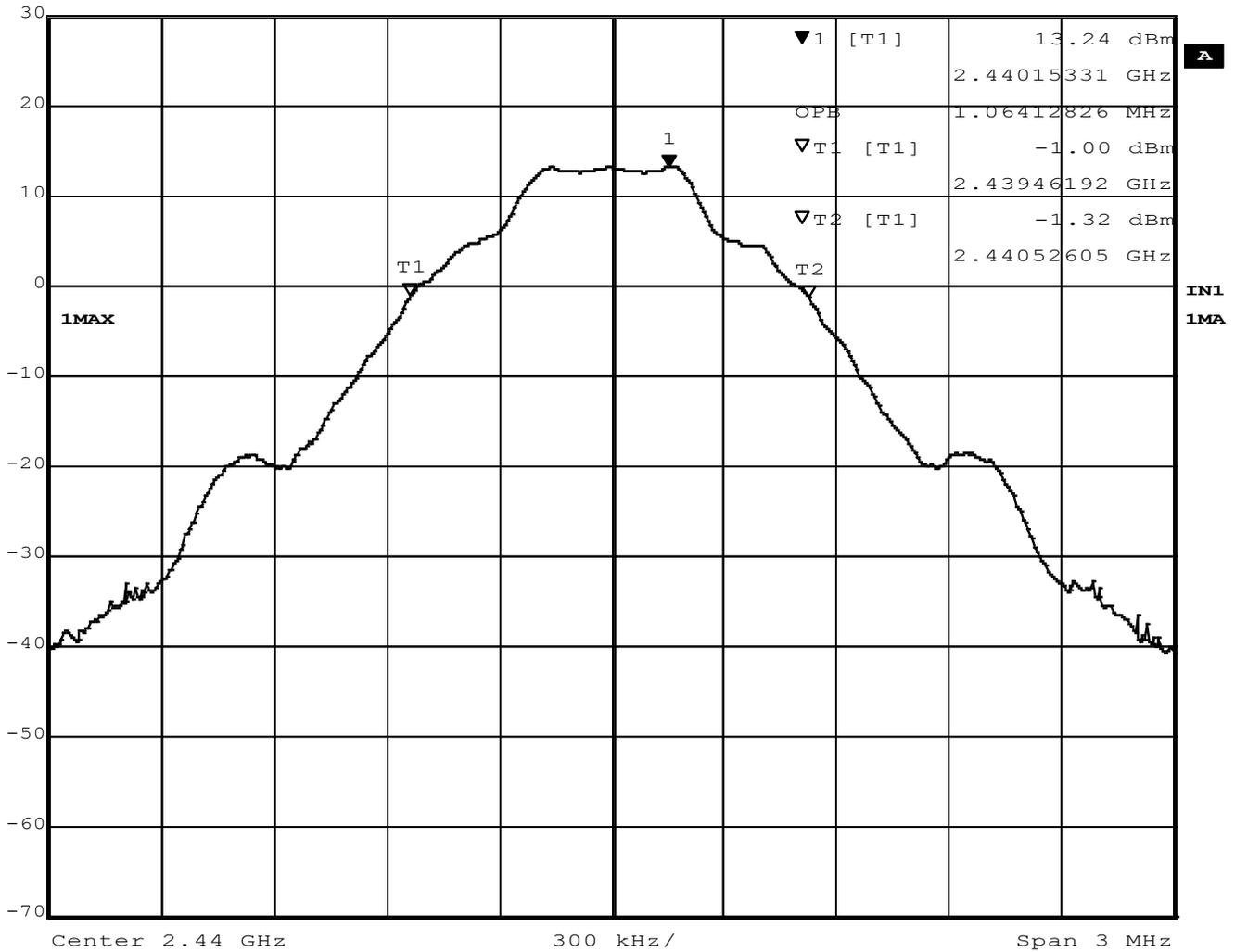
Figure 13 - Occupied Bandwidth, Mid Channel, BT BR (GFSK)
