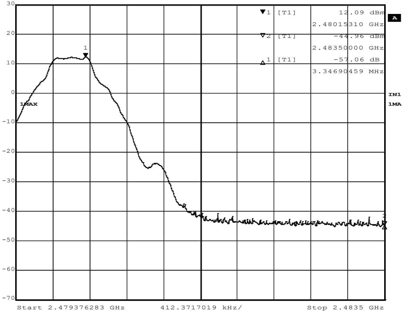
Figure 47 - Band-edge Measurement, High Channel, Fundamental, Peak
