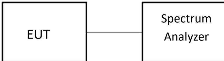
**Figure 11 – Peak Output Power Measurements Test Setup**
