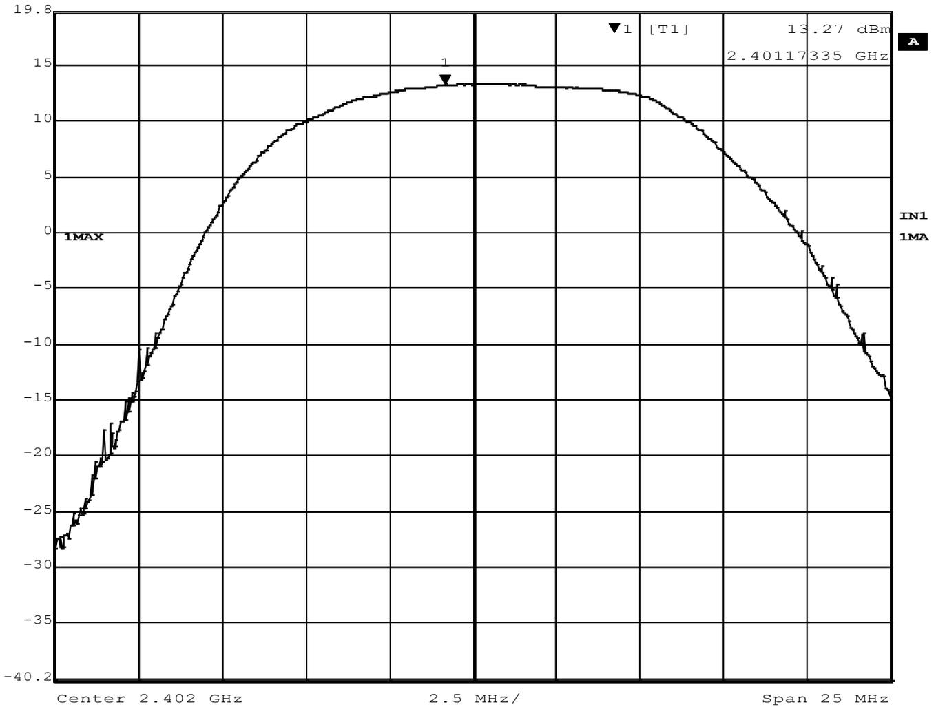
**Figure 5 – Output Power, Low Channel, BT EDR 2MB**
