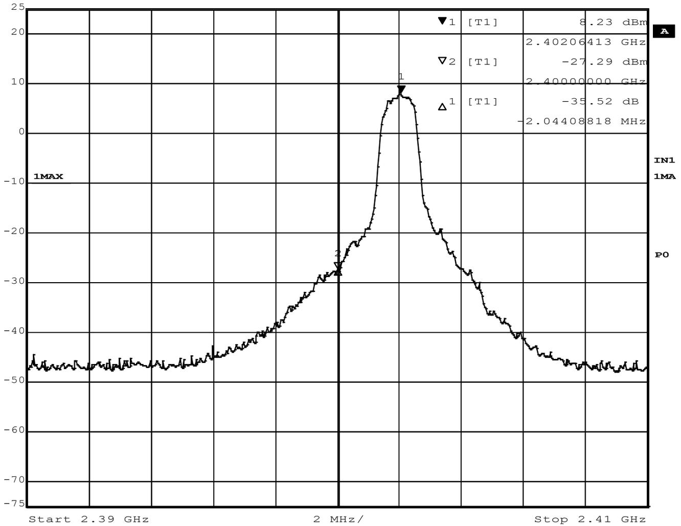
Figure 49 - Band-edge Measurement, Low Channel, Fundamental, Peak
