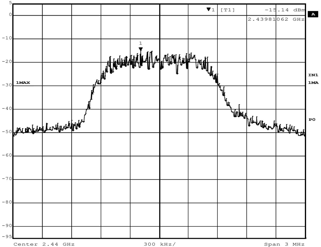
Figure 42 - Power Spectral Density, Mid Channel, BT EDR 3MB
