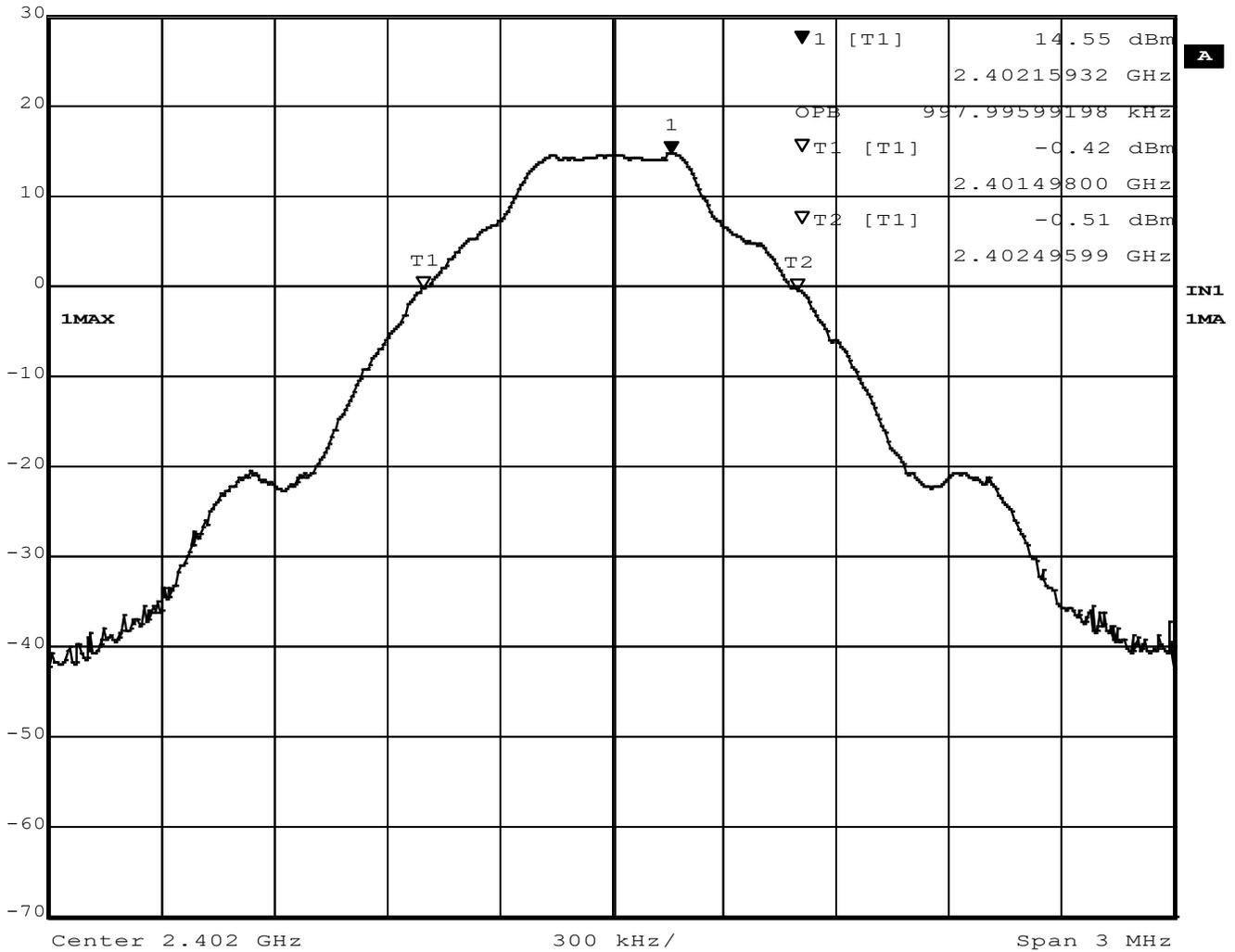
Figure 12 – Occupied Bandwidth, Low Channel, BT BR (GFSK)
