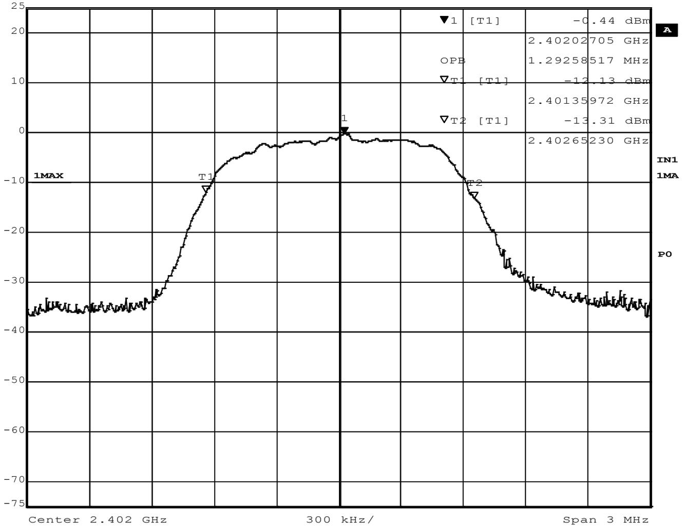
Figure 15 – Occupied Bandwidth, Low Channel, BT EDR 2MB
