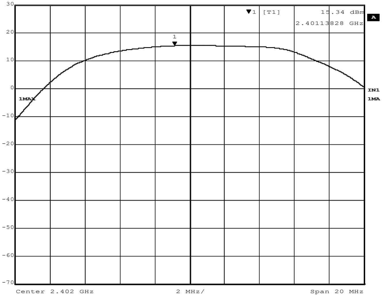
**Figure 2 – Output Power, Low Channel, BT BR (GFSK)**
