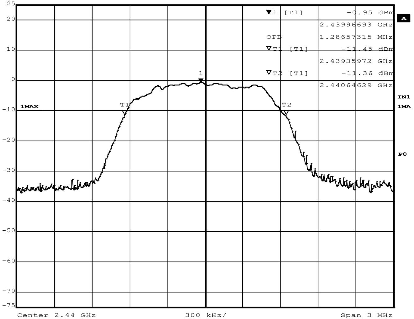
Figure 19 - Occupied Bandwidth, Mid Channel, BT EDR 3MB
