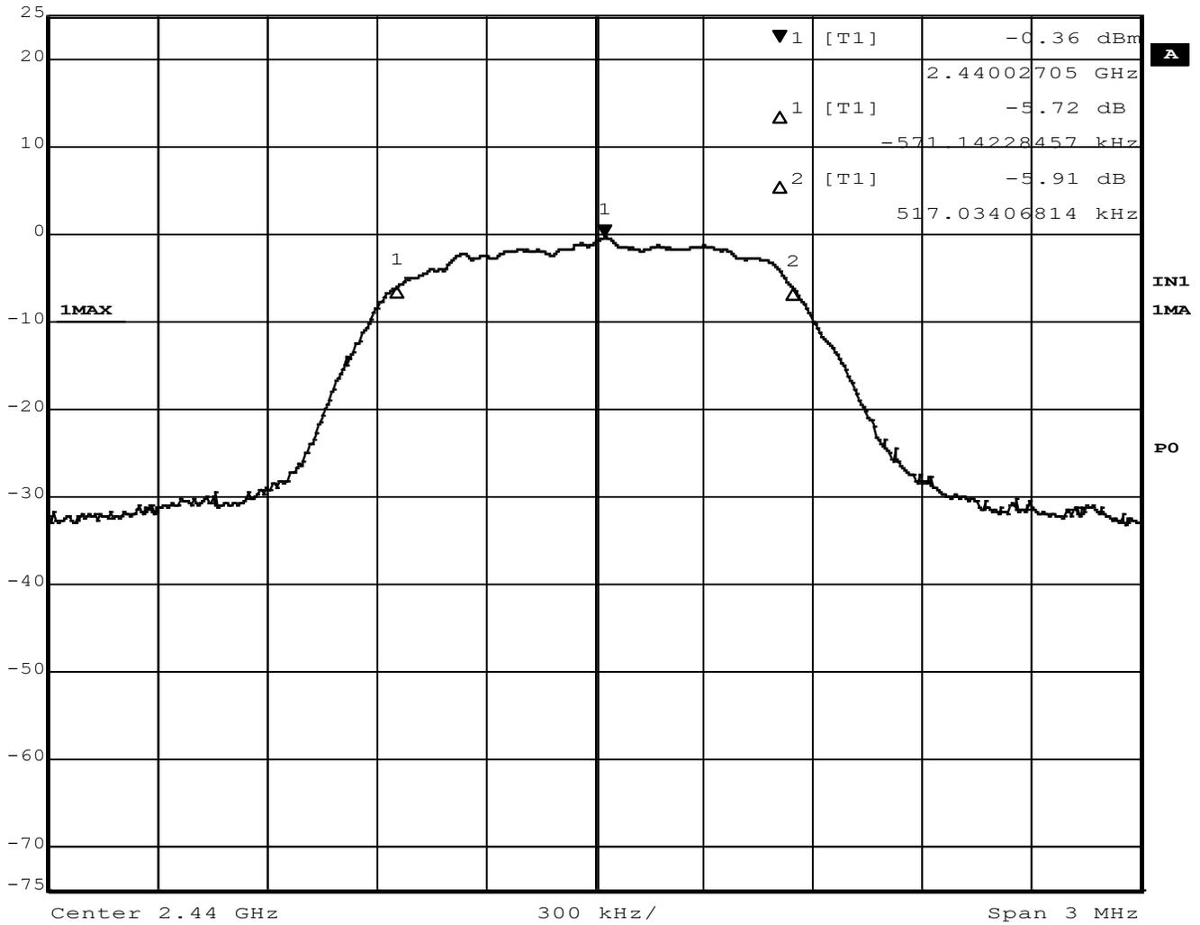
Figure 25 – 6dB Bandwidth, Mid Channel, BT EDR 2MB
