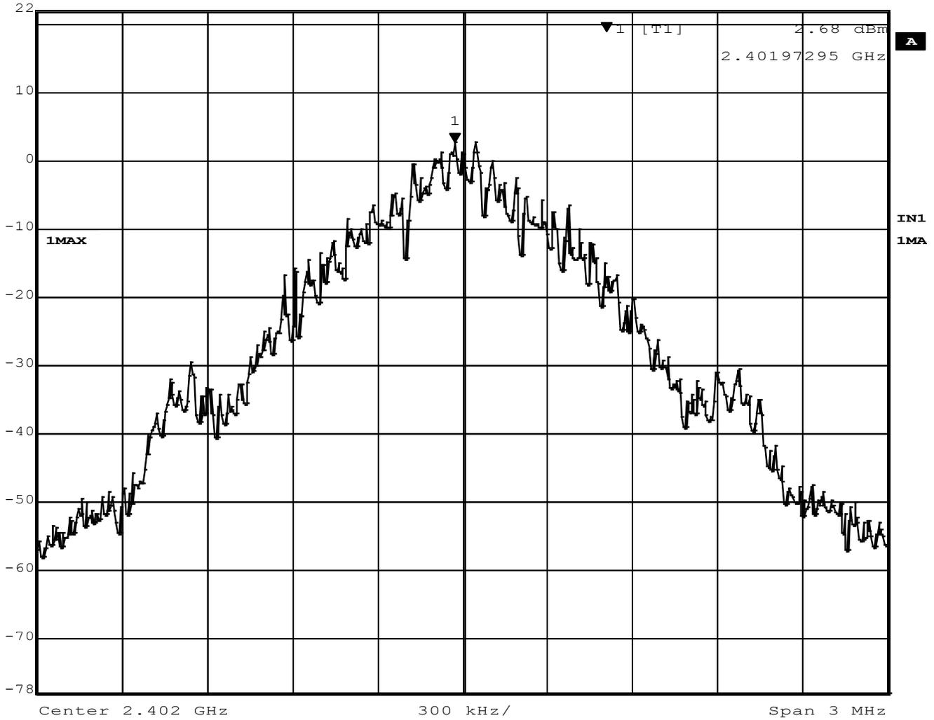
Figure 35 - Power Spectral Density, Low Channel, BT BR (GFSK)
