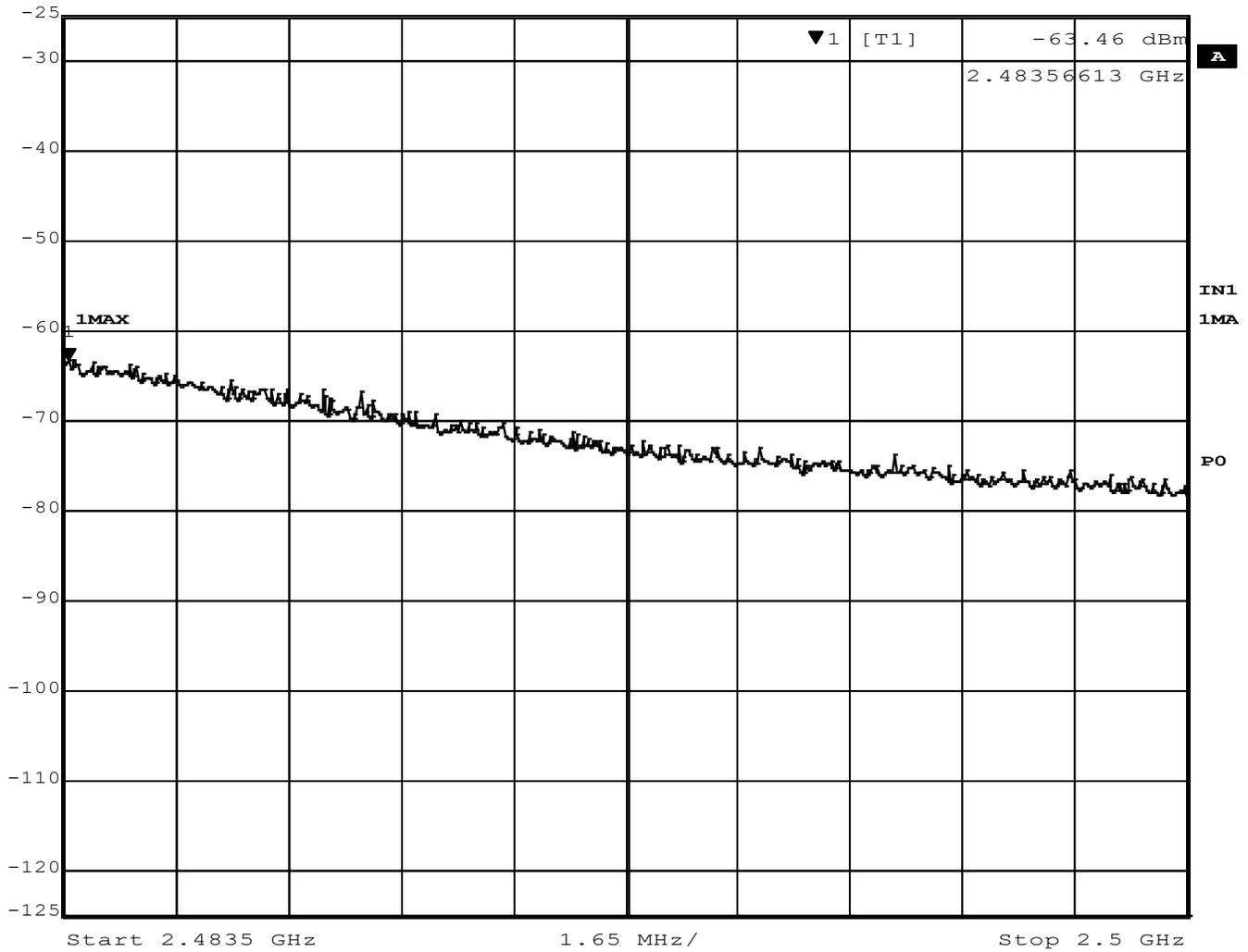
**Figure 46 - Band-edge Measurement, High Channel, Restricted Frequency, Peak**
