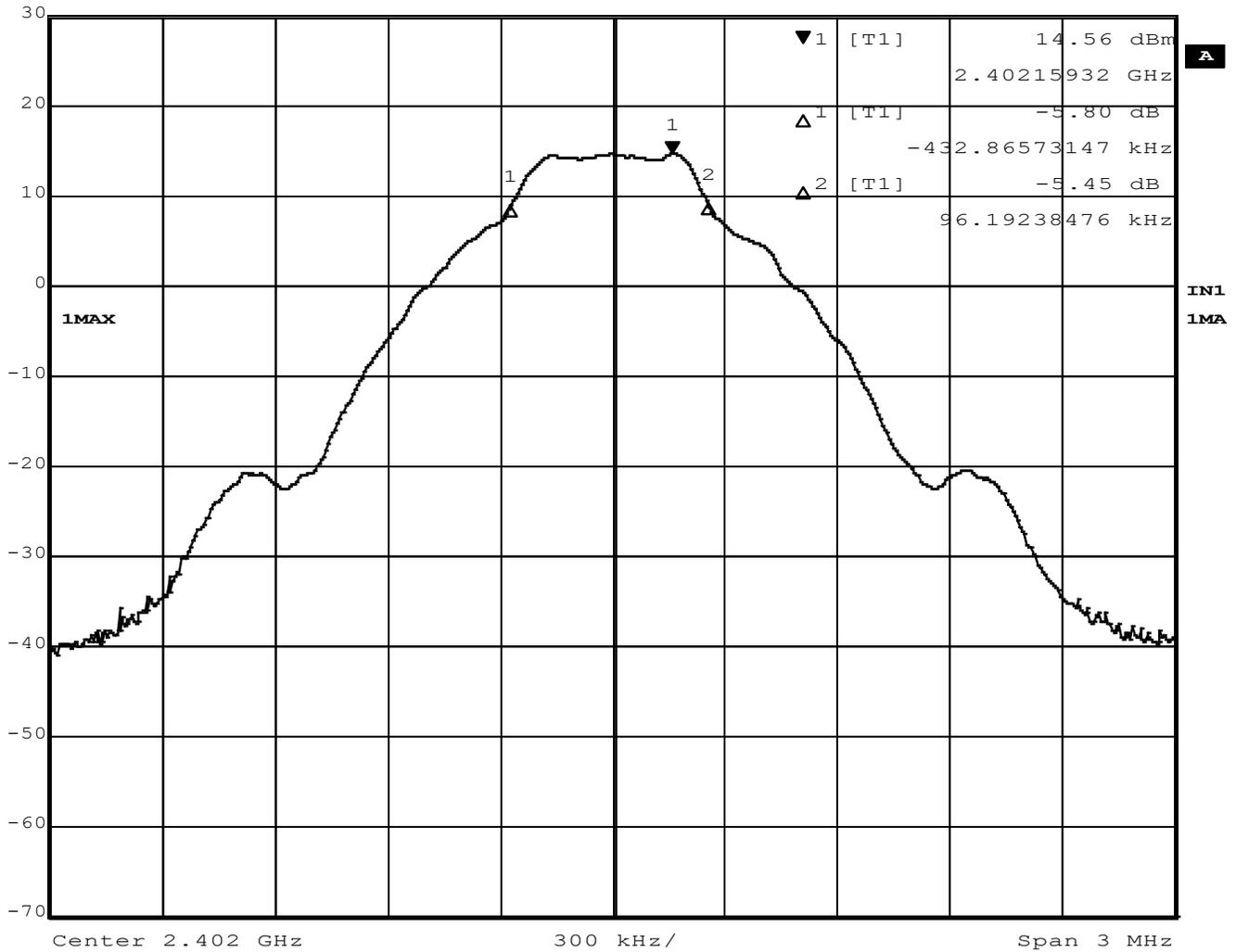
Figure 21 – 6dB Bandwidth, Low Channel, BT BR (GFSK)
