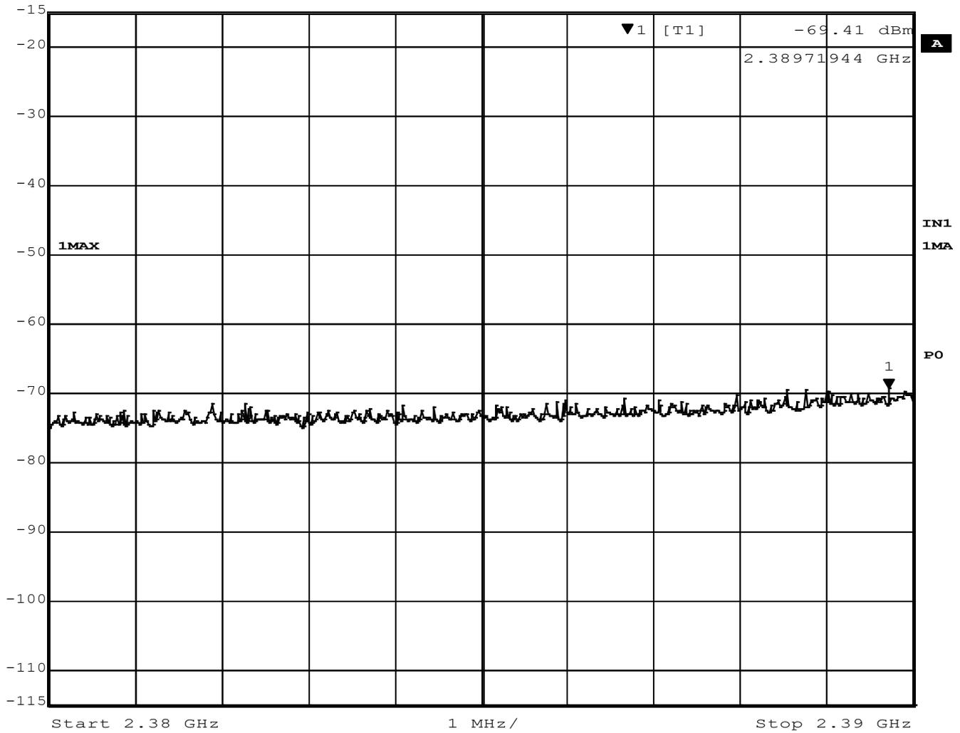
Figure 48 - Band-edge Measurement, Low Channel, Restricted Frequency, Peak
