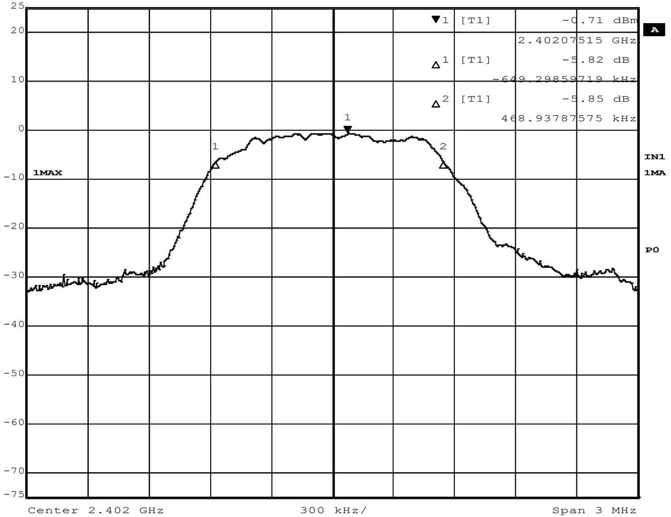
Figure 27 – 6dB Bandwidth, Low Channel, BT EDR 3MB
