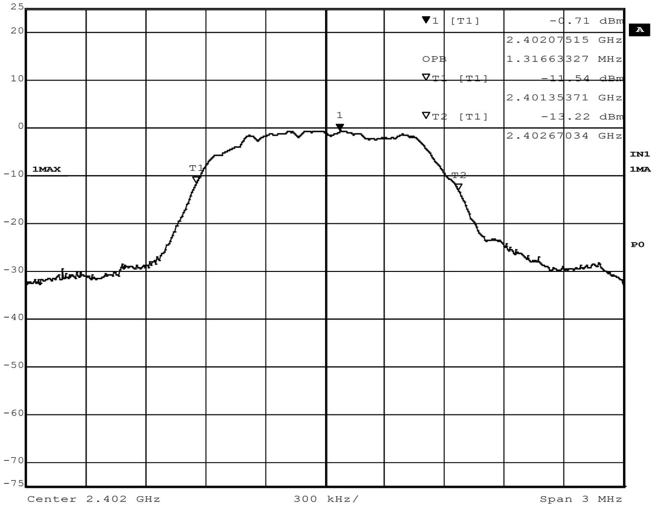
Figure 18 – Occupied Bandwidth, Low Channel, BT EDR 3MB
