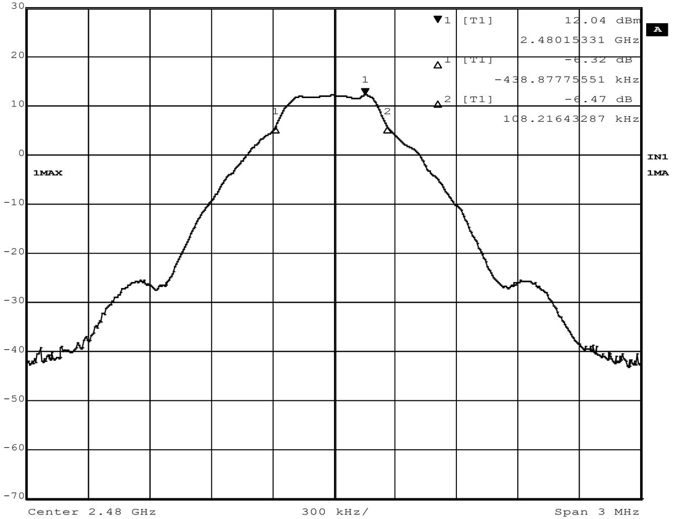
Figure 23 – 6dB Bandwidth, High Channel, BT BR (GFSK)
