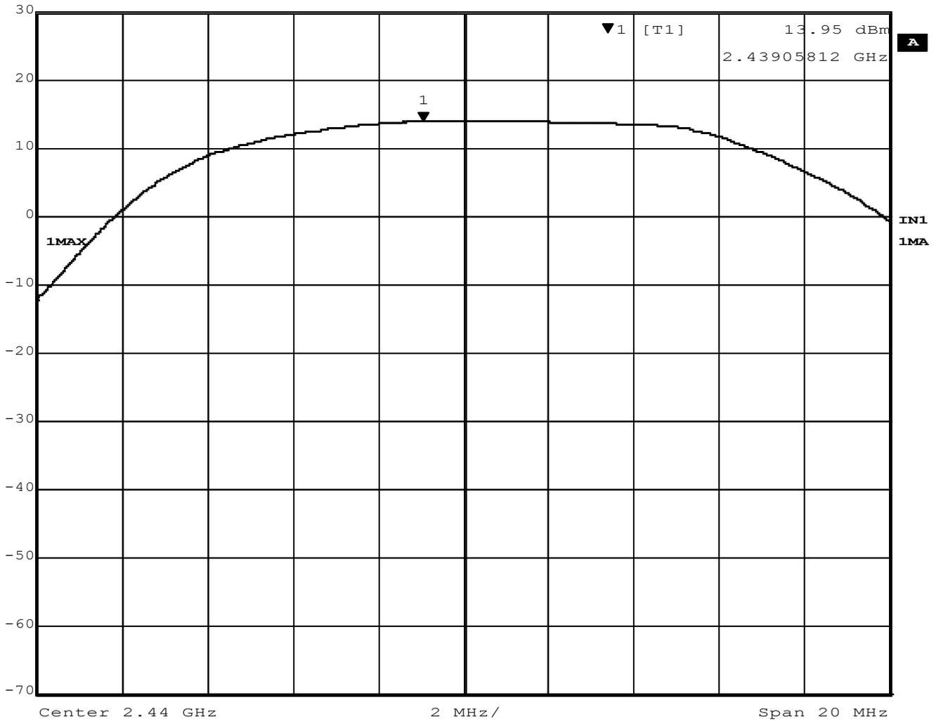
**Figure 3 – Output Power, Mid Channel, BT BR (GFSK)**
