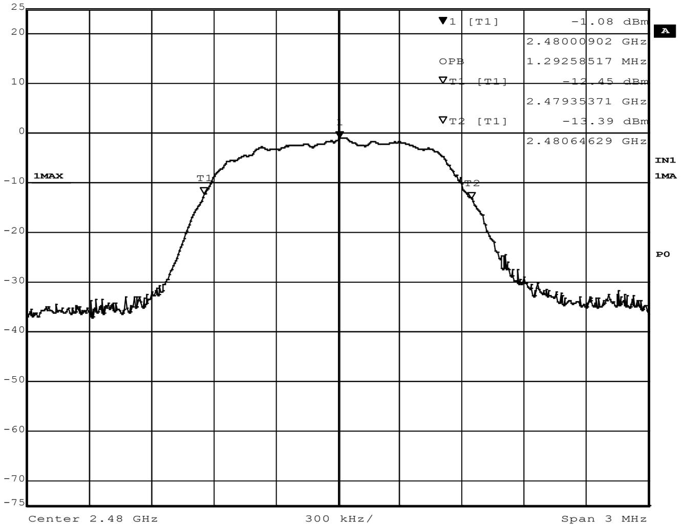
Figure 17 - Occupied Bandwidth, High Channel, BT EDR 2MB
