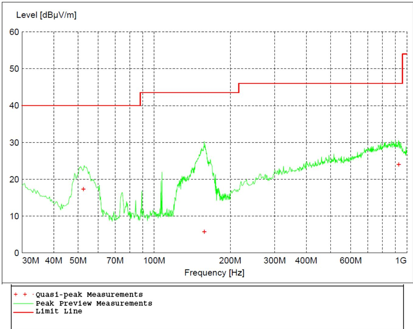
Figure 34 - Radiated Emissions Plot, BT EDR 3MB
