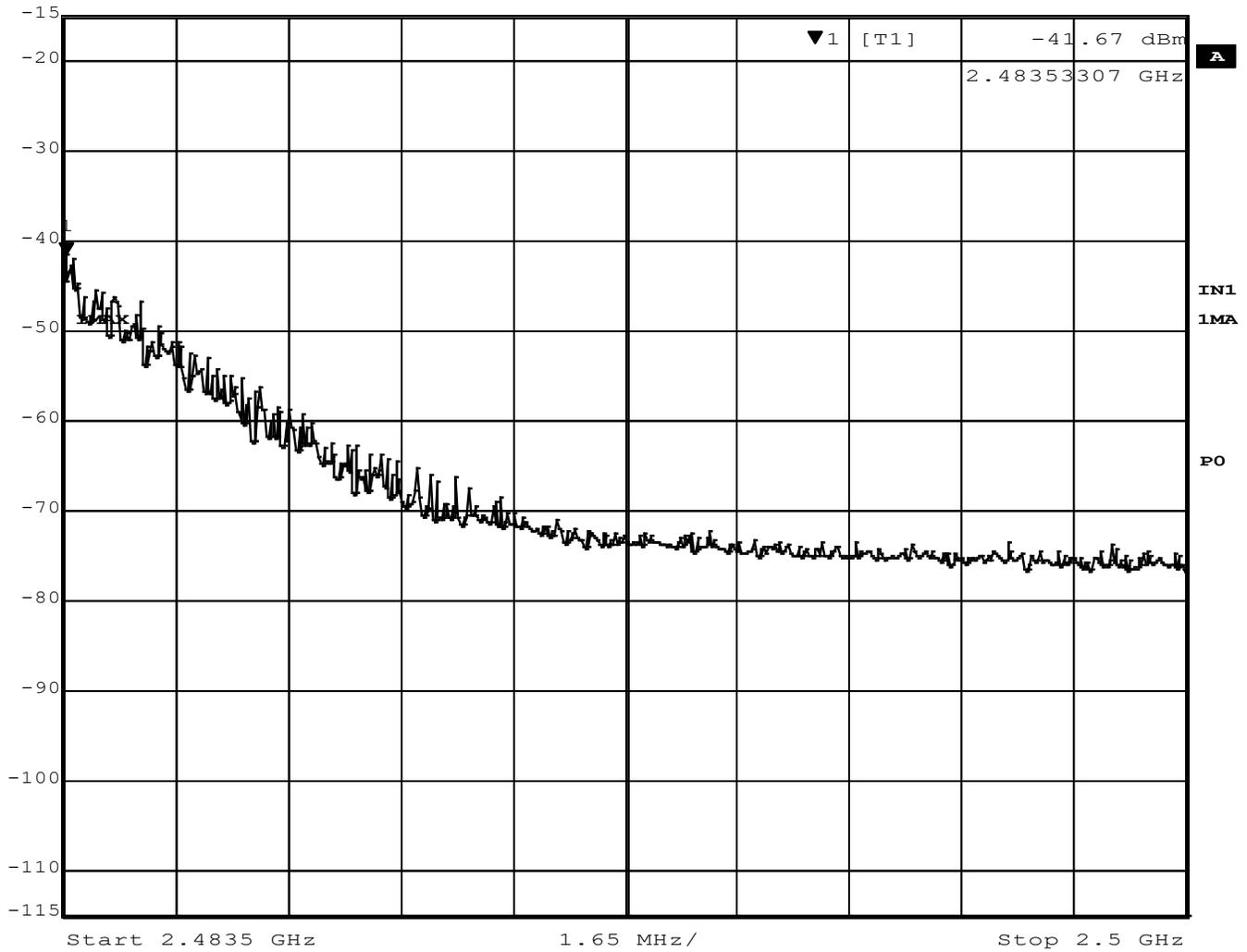
**Figure 50 - Band-edge Measurement, High Channel, Restricted Frequency, Peak**
