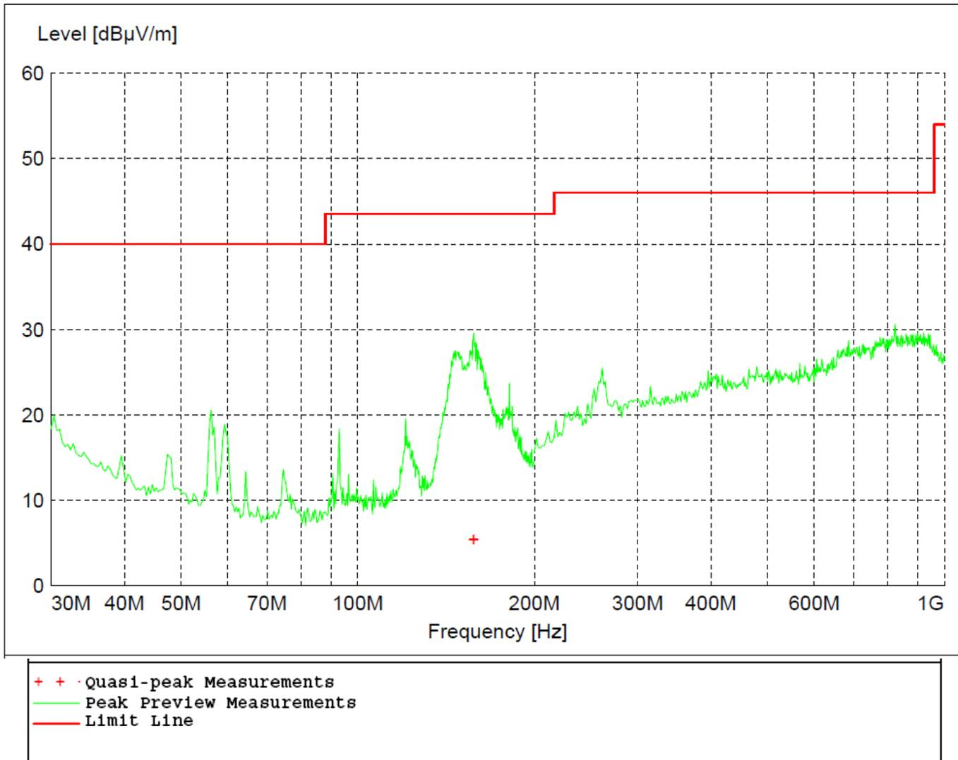
**Figure 31 - Radiated Emissions Plot, Receive**
