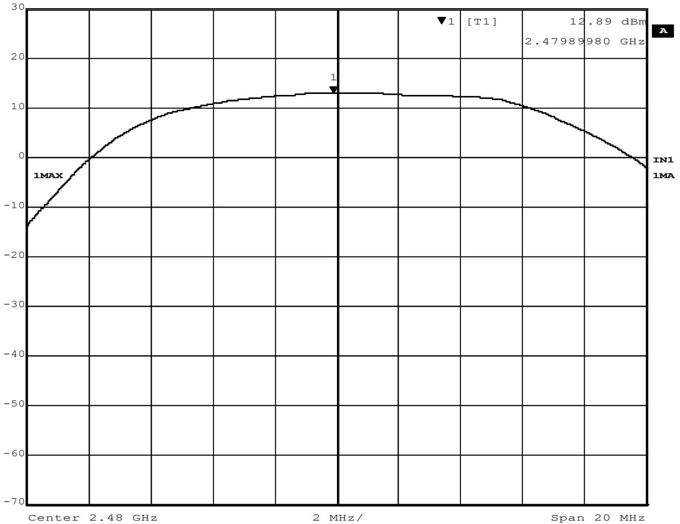
**Figure 4 – Output Power, High Channel, BT BR (GFSK)**
