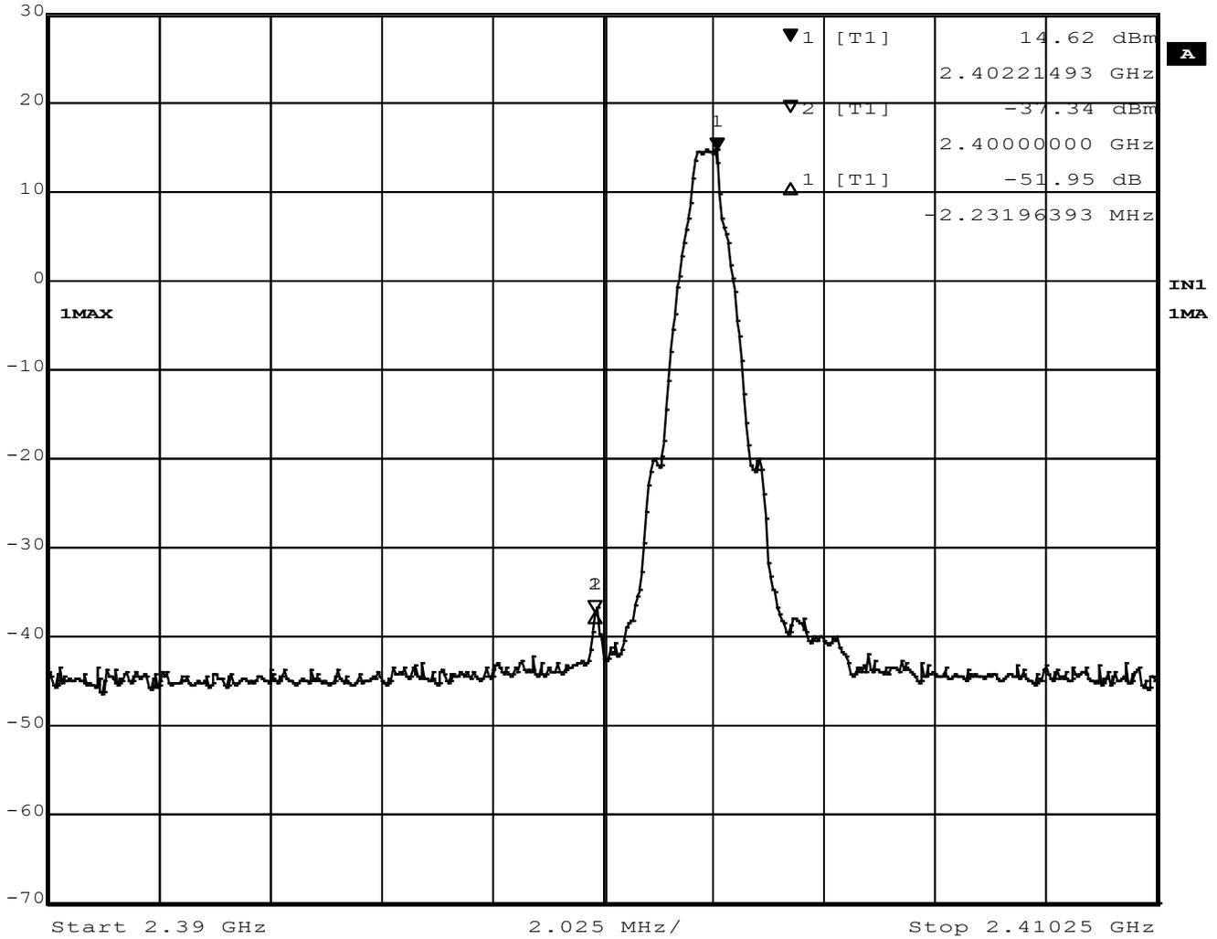
Figure 45 - Band-edge Measurement, Low Channel, Fundamental, Peak
