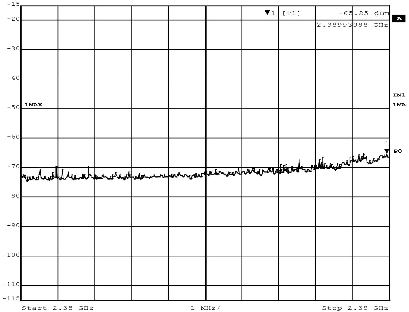
Figure 52 - Band-edge Measurement, Low Channel, Restricted Frequency, Peak
