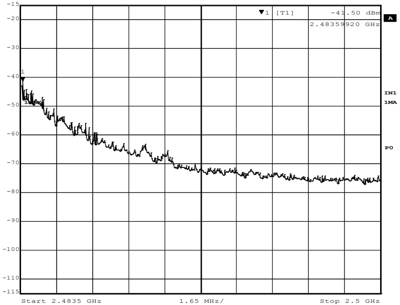
**Figure 54 - Band-edge Measurement, High Channel, Restricted Frequency, Peak**
