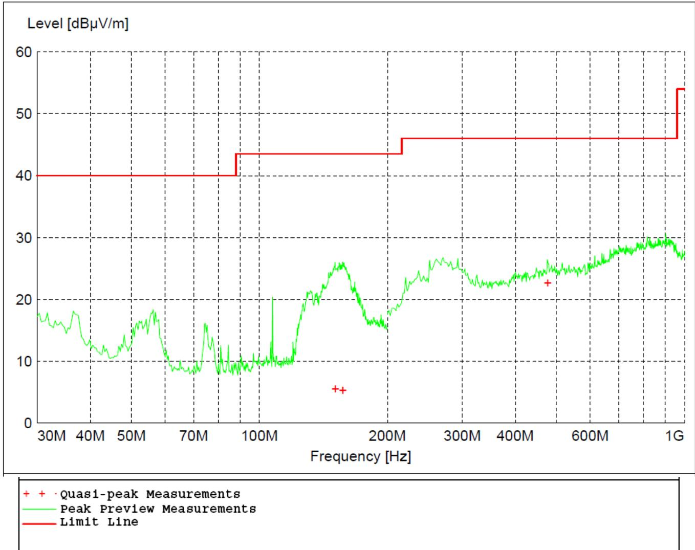
Figure 32 - Radiated Emissions Plot, BT BR (GFSK)
