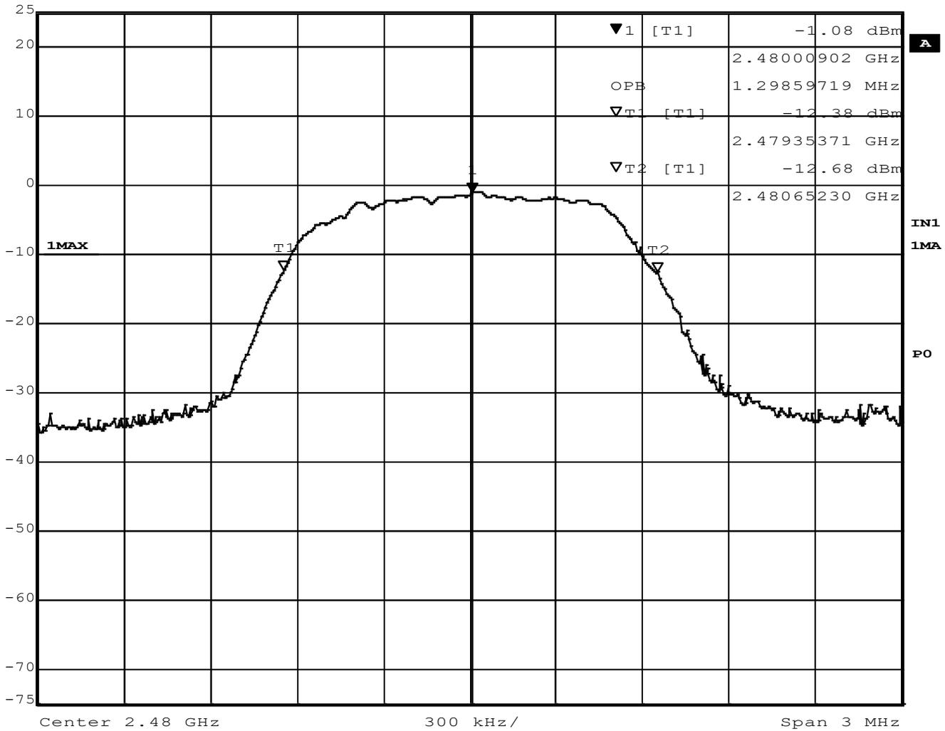
Figure 20 - Occupied Bandwidth, High Channel, BT EDR 3MB
