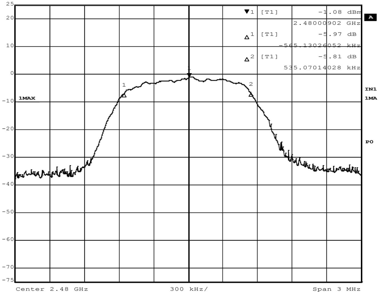
Figure 26 – 6dB Bandwidth, High Channel, BT EDR 2MB
