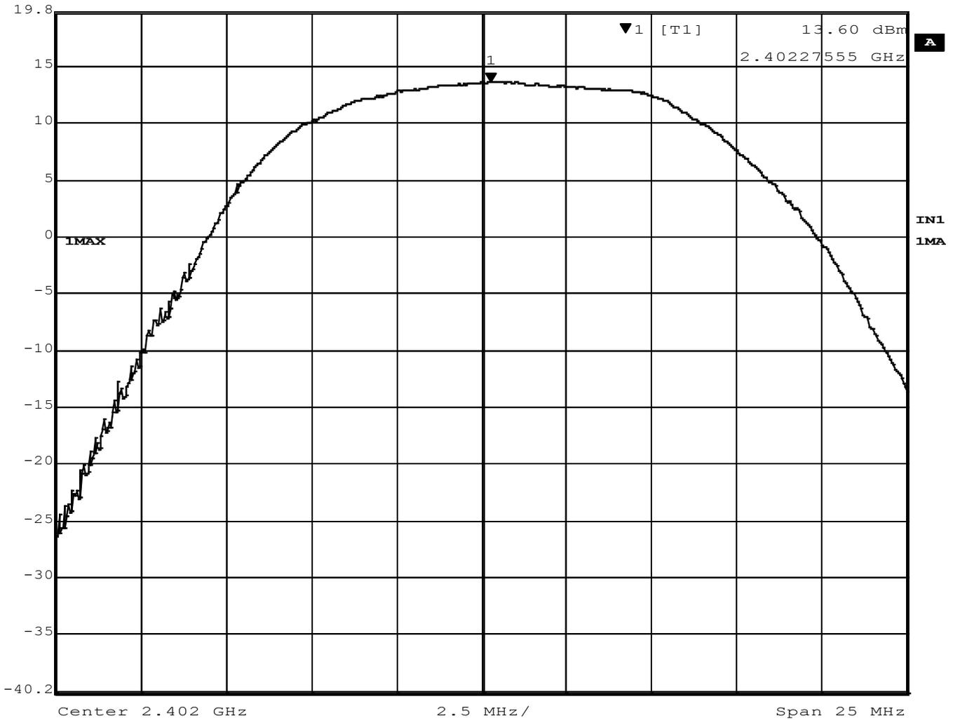
**Figure 8 – Output Power, Low Channel, BT EDR 3MB**
