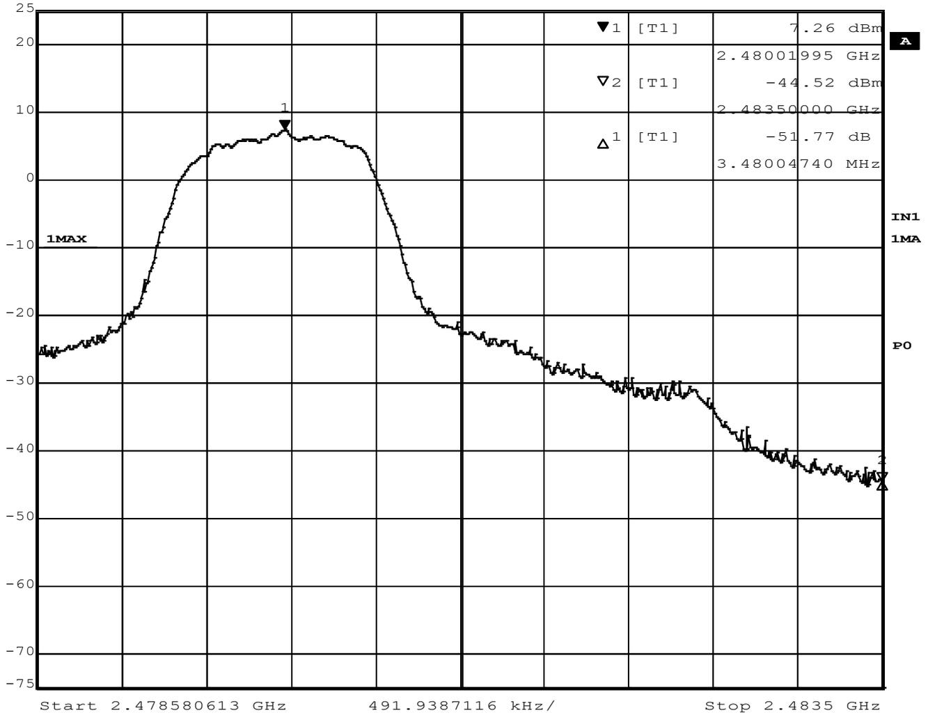
Figure 51 - Band-edge Measurement, High Channel, Fundamental, Peak
