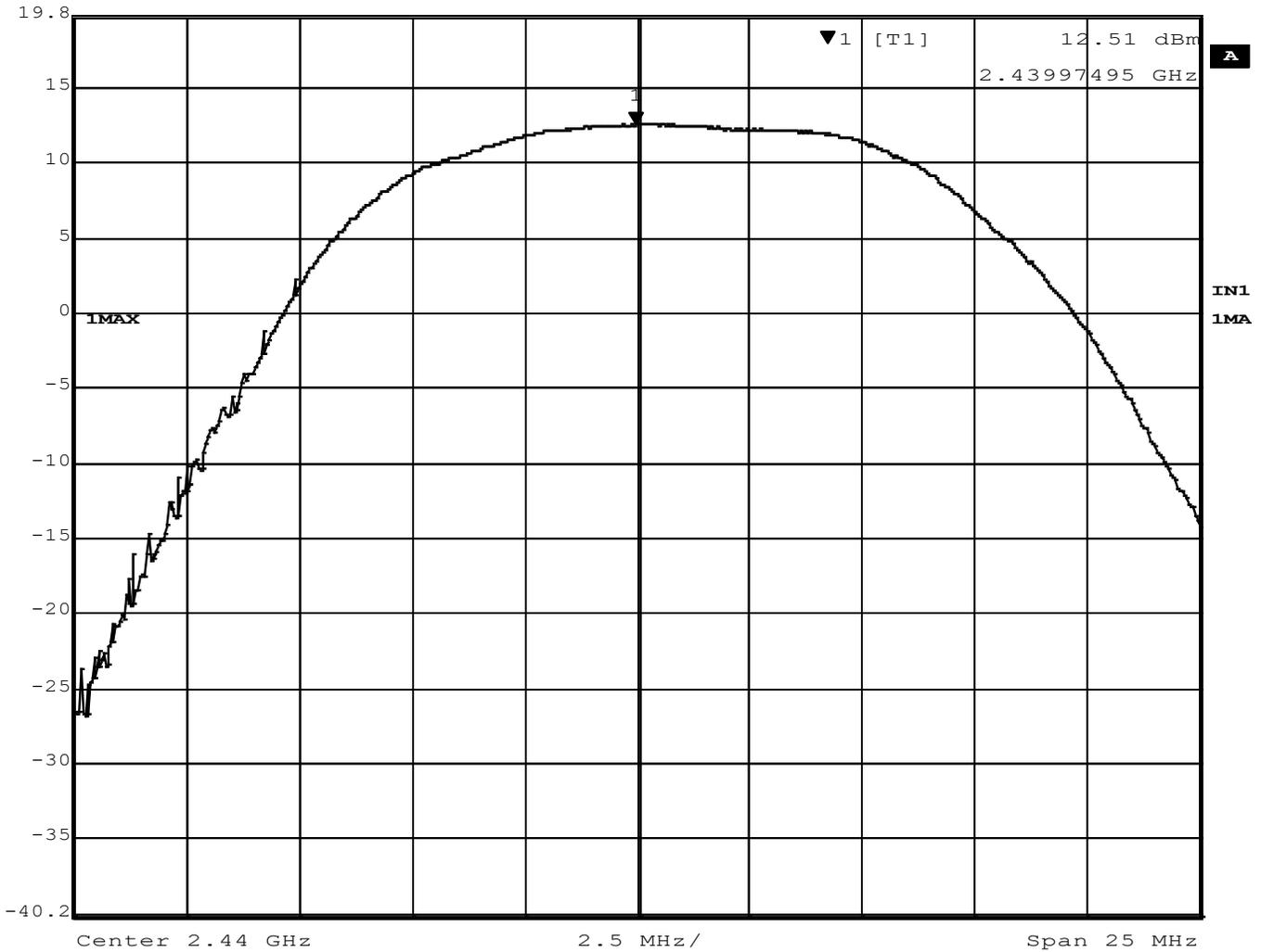
**Figure 6 – Output Power, Mid Channel, BT EDR 2MB**
