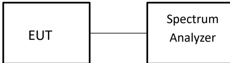
**Figure 1 – Peak Output Power Measurements Test Setup**
