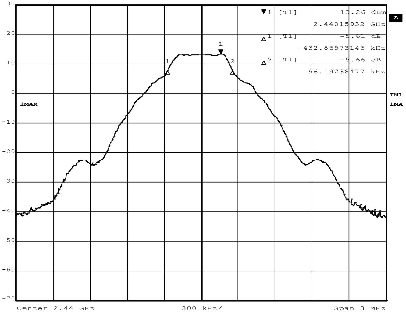
Figure 22 – 6dB Bandwidth, Mid Channel, BT BR (GFSK)
