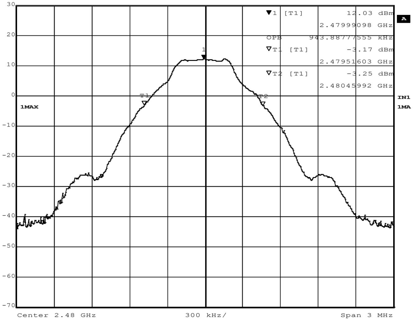
Figure 14 - Occupied Bandwidth, High Channel, BT BR (GFSK)
