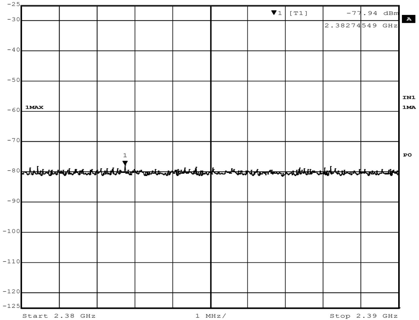
**Figure 44 - Band-edge Measurement, Low Channel, Restricted Frequency, Peak**
