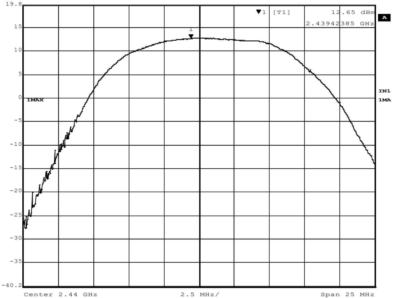
**Figure 9 – Output Power, Mid Channel, BT EDR 3MB**
