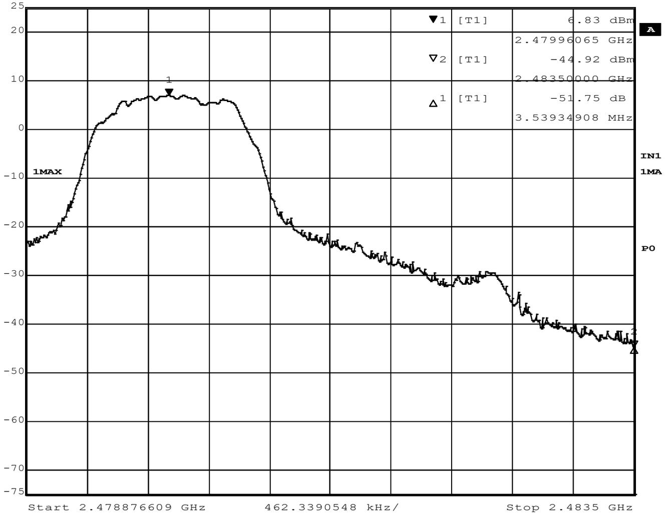
Figure 55 - Band-edge Measurement, High Channel, Fundamental, Peak
