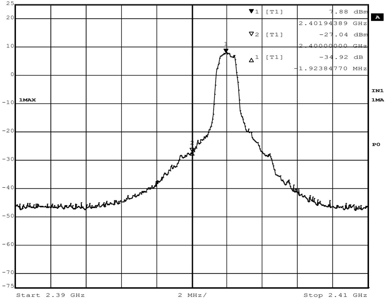
Figure 53 - Band-edge Measurement, Low Channel, Fundamental, Peak
