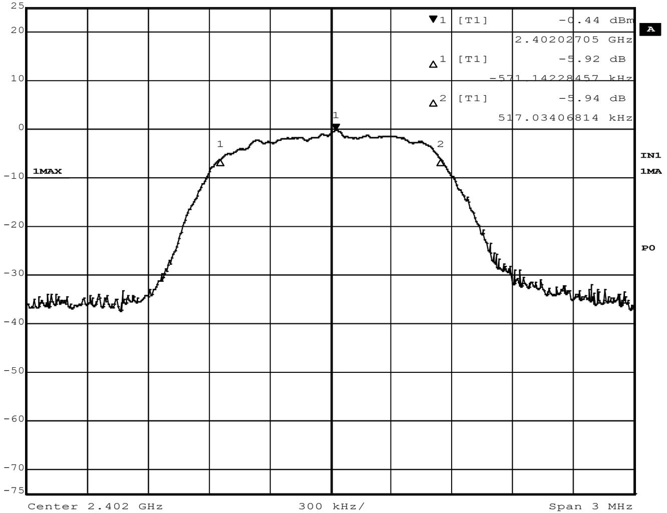
Figure 24 – 6dB Bandwidth, Low Channel, BT EDR 2MB
