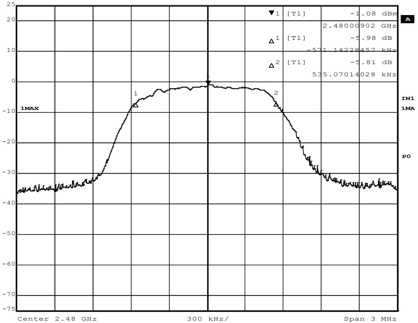
Figure 29 – 6dB Bandwidth, High Channel, BT EDR 3MB
