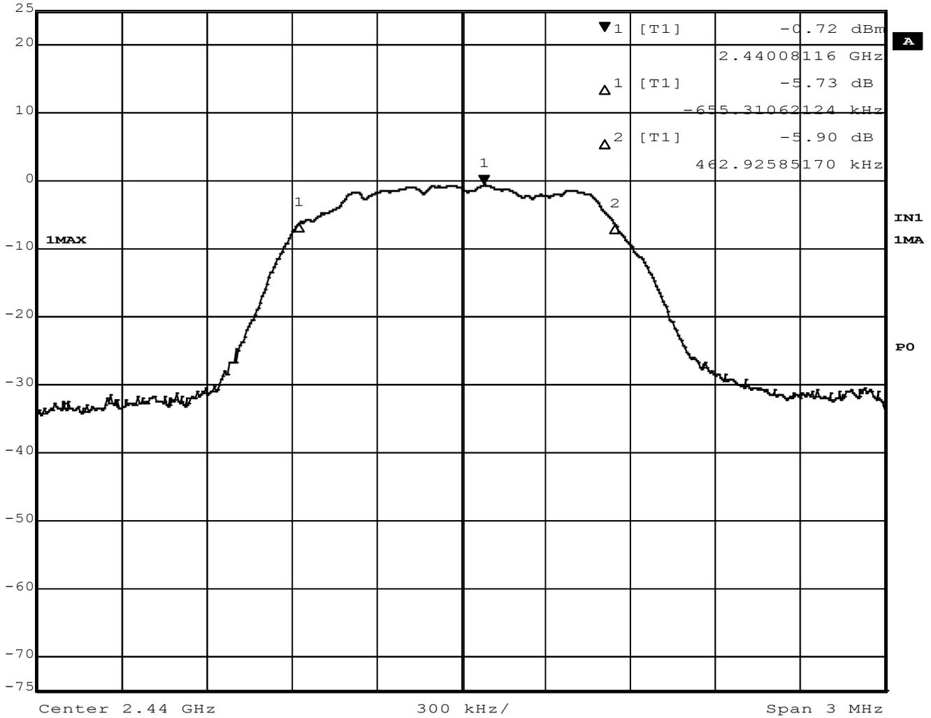
Figure 28 – 6dB Bandwidth, Mid Channel, BT EDR 3MB
