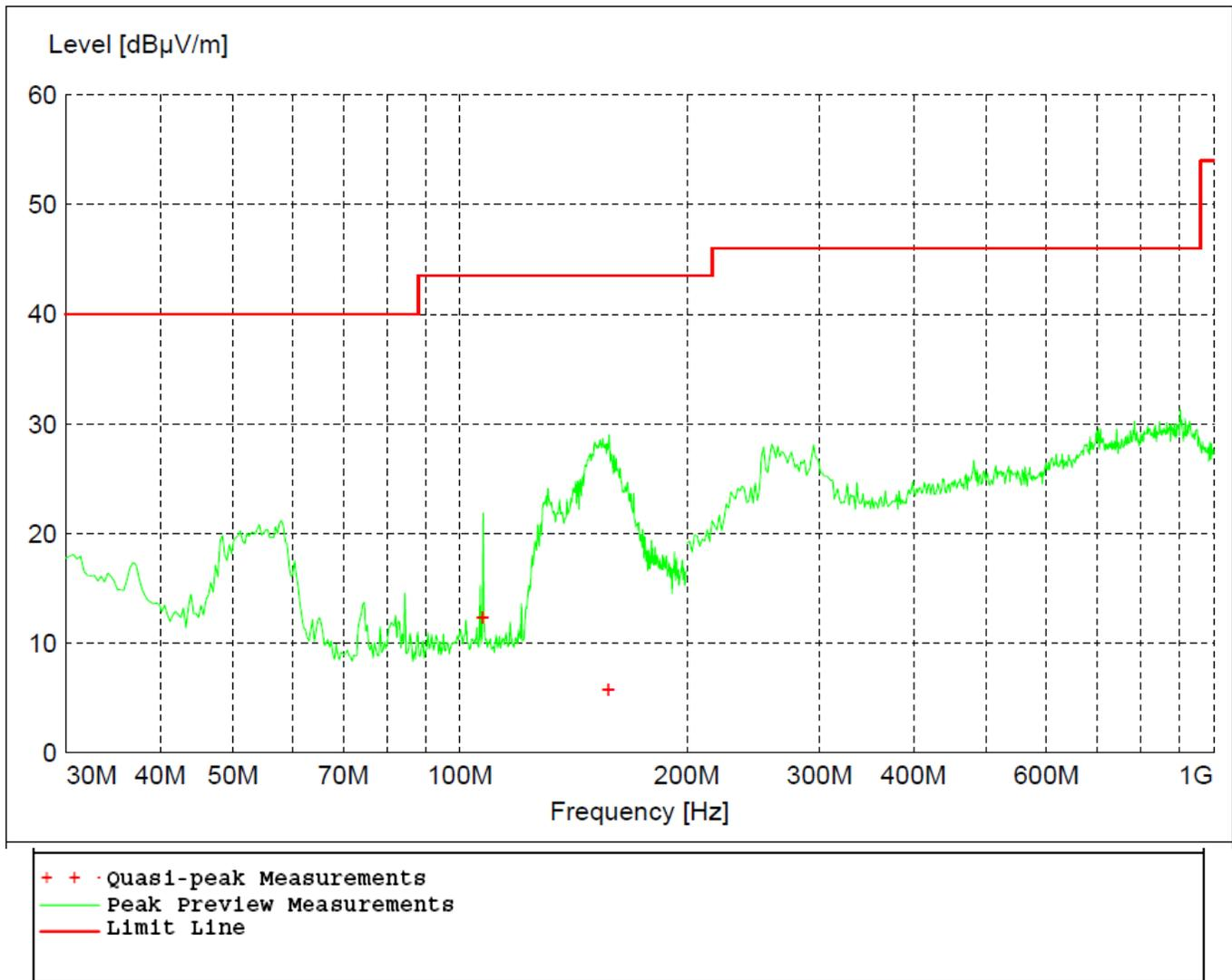
Figure 33 - Radiated Emissions Plot, BT EDR 2MB
