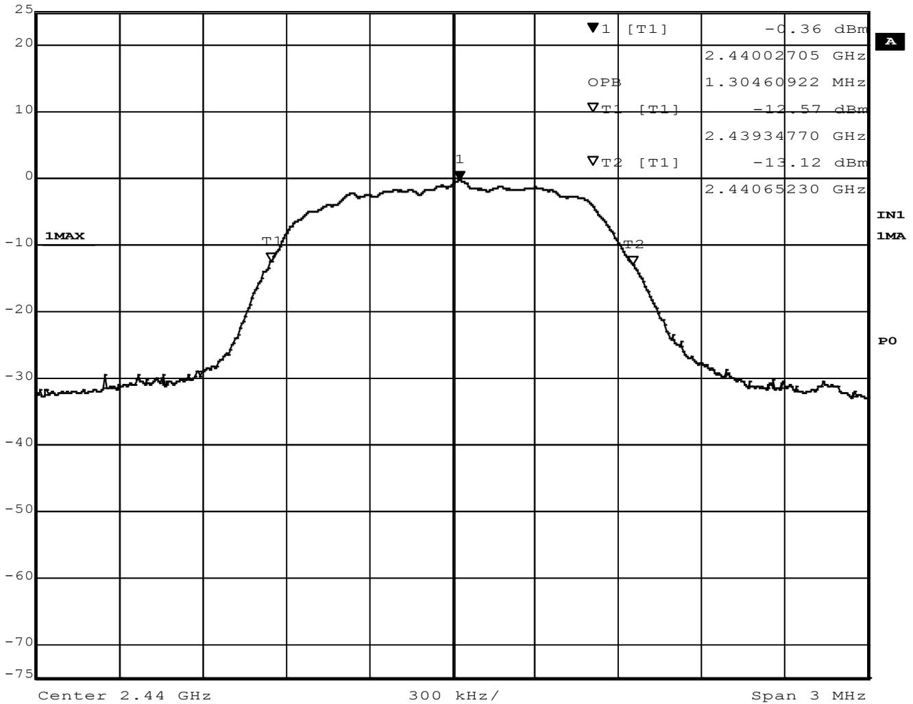
Figure 16 - Occupied Bandwidth, Mid Channel, BT EDR 2MB
