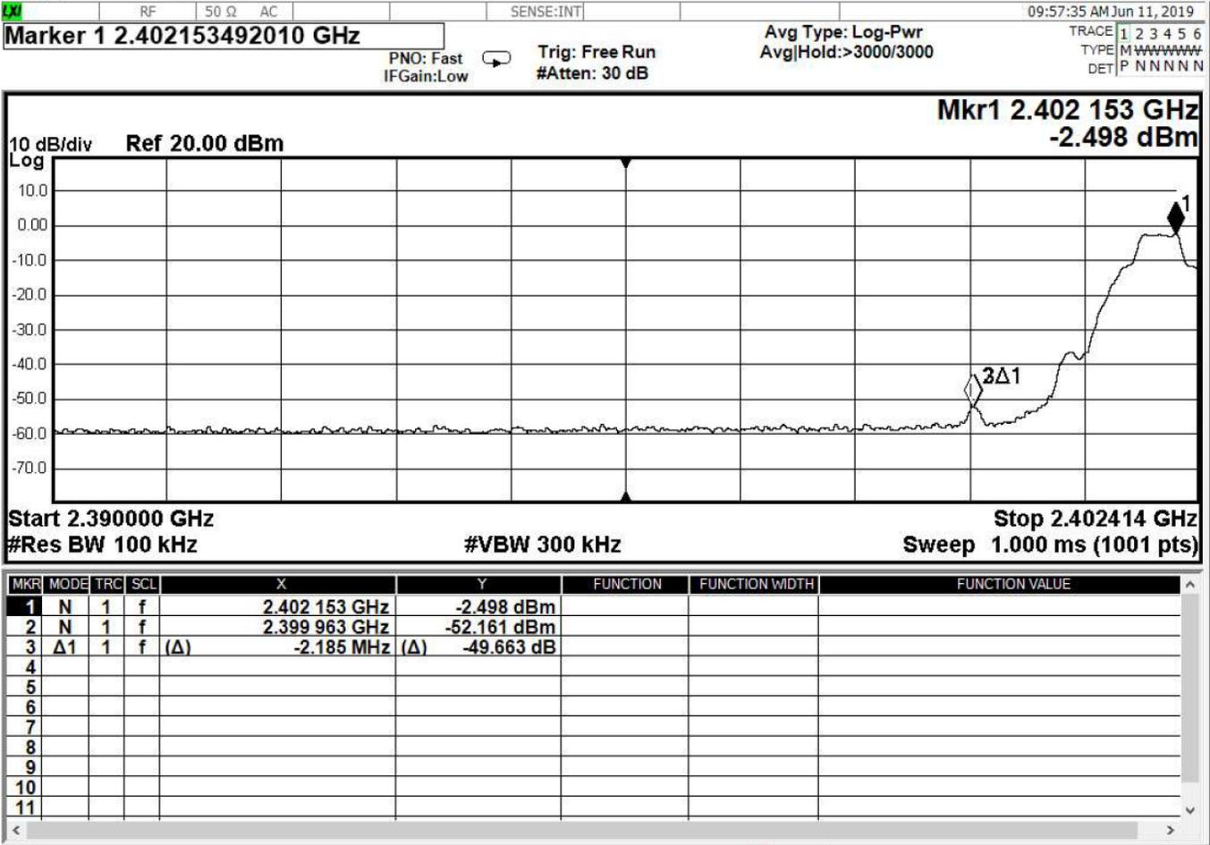
Figure 20 – Band Edge Measurement, Low Channel, GFSK
