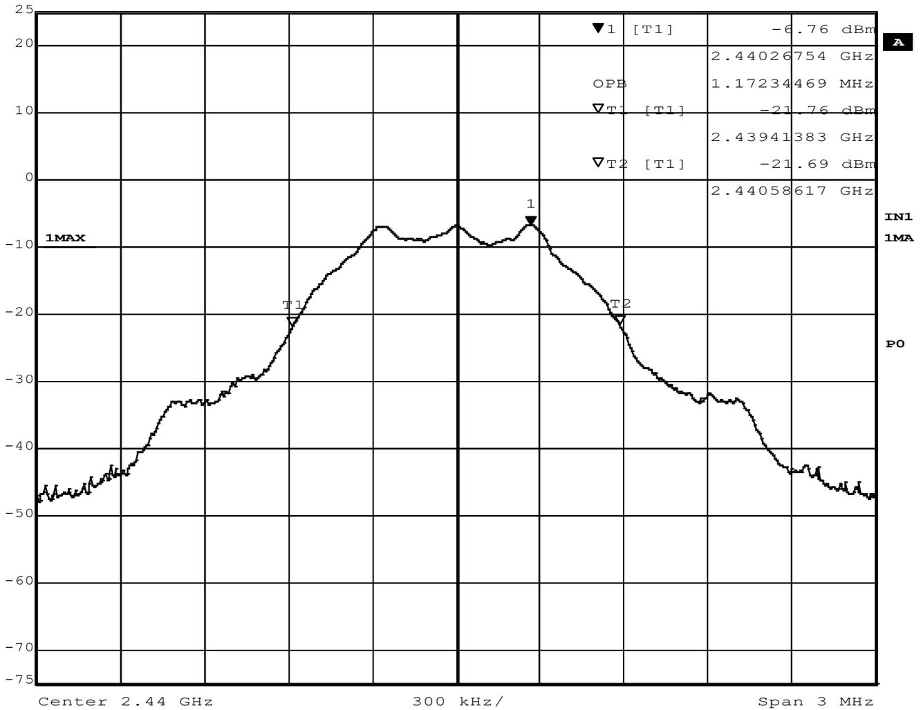
Figure 9 - Occupied Bandwidth, Mid Channel, GMSK
