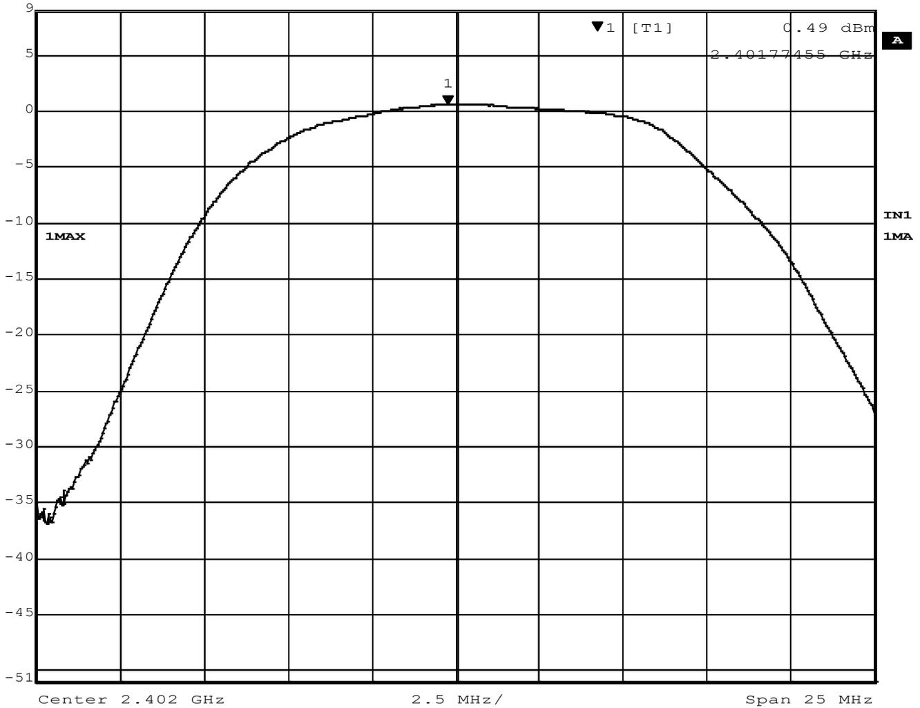
**Figure 1 – Output Power, Low Channel, GMSK**
