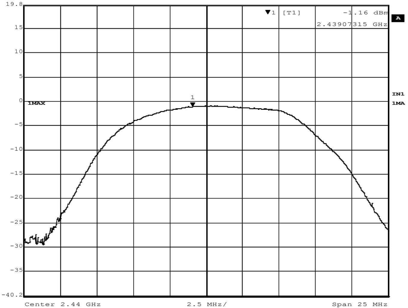
**Figure 2 – Output Power, Mid Channel, GMSK**
