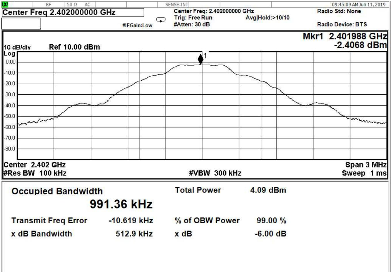
Figure 11 – Occupied Bandwidth, Low Channel, GFSK
