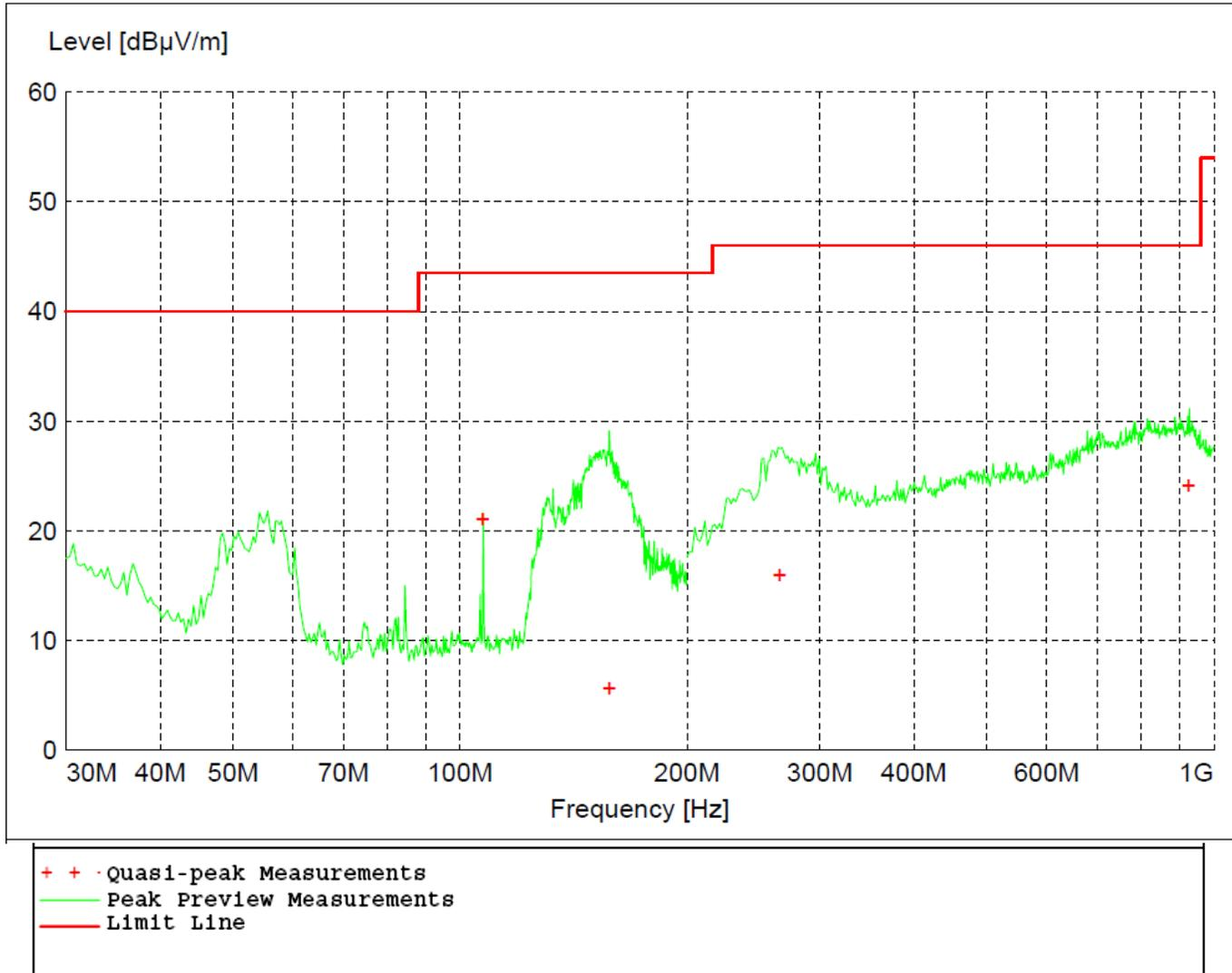
Figure 16 - Radiated Emissions Plot, GMSK
