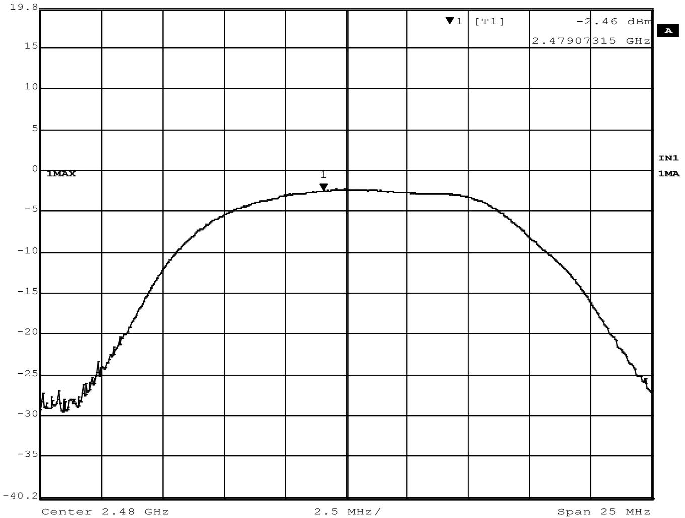
**Figure 3 – Output Power, High Channel, GMSK**
