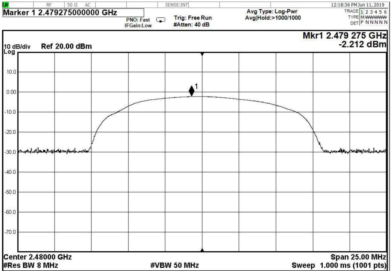
Figure 6 – Output Power, High Channel, GFSK
