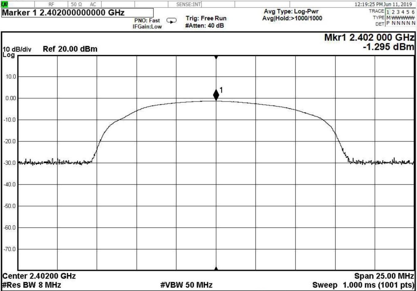
Figure 4 – Output Power, Low Channel, GFSK
