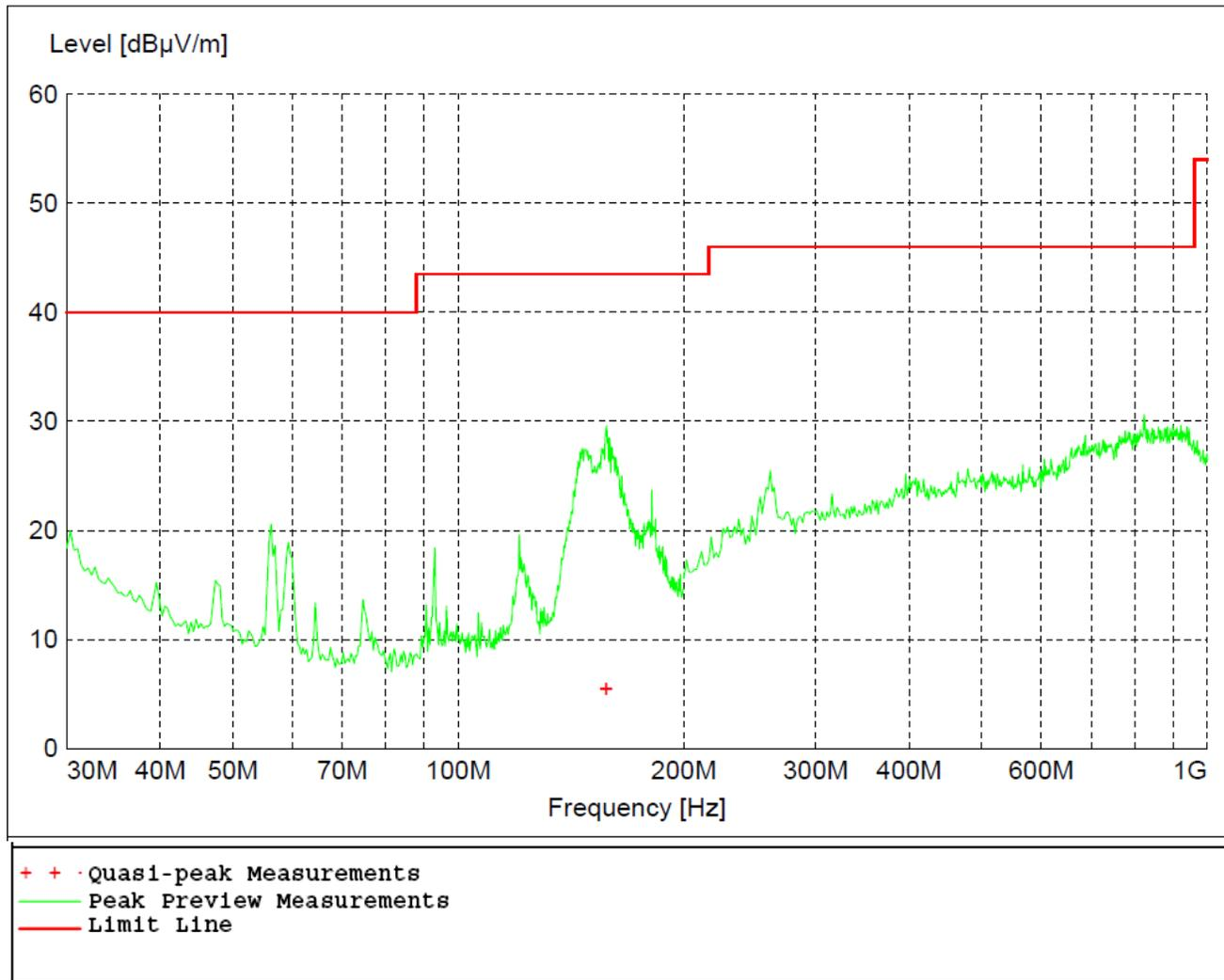
**Figure 15 - Radiated Emissions Plot, Receive**
