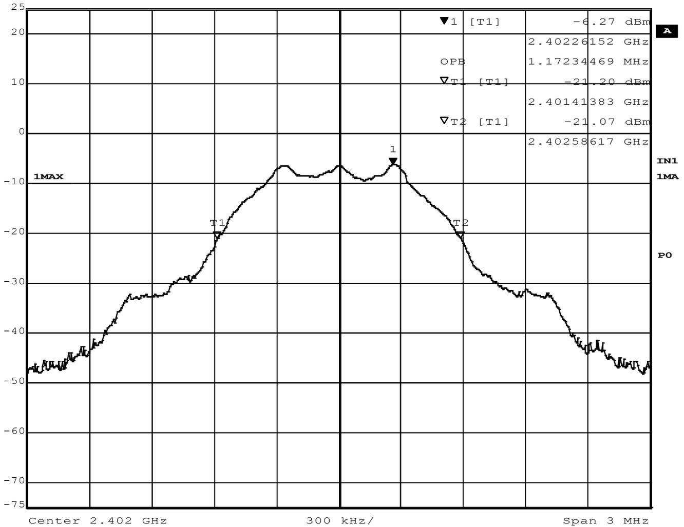
Figure 8 – Occupied Bandwidth, Low Channel, GMSK
