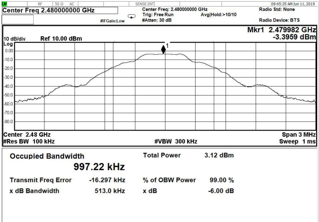
Figure 13 – Occupied Bandwidth, High Channel, GFSK
