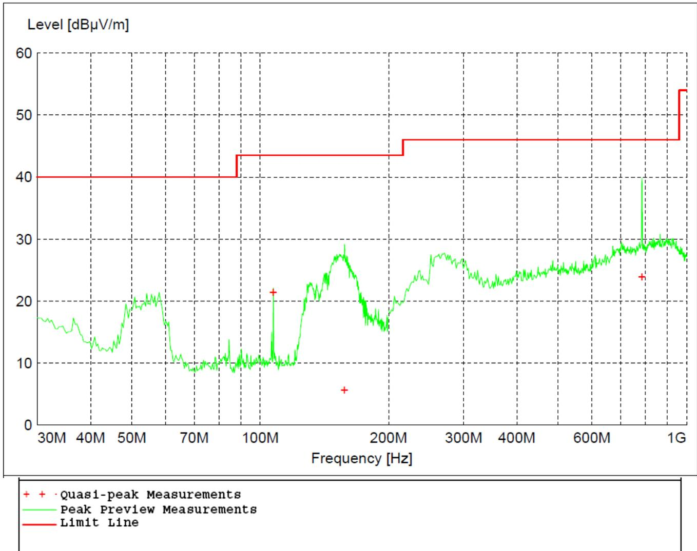
Figure 17 - Radiated Emissions Plot, GFSK
