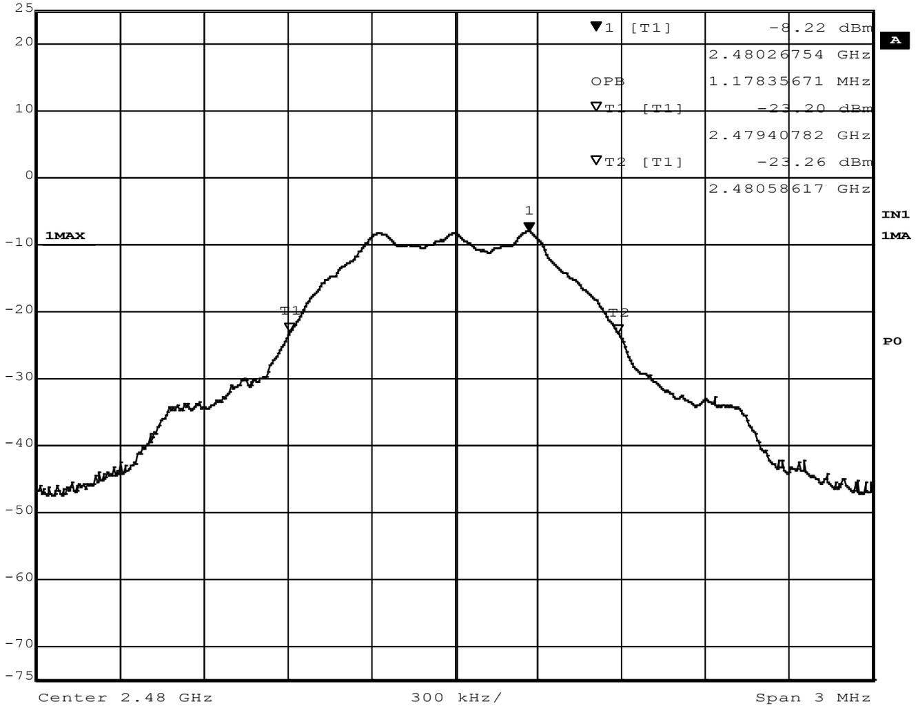
Figure 10 – Occupied Bandwidth, High Channel, GMSK
