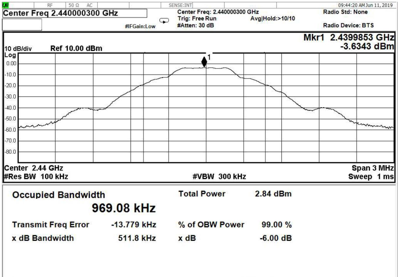
Figure 12 – Occupied Bandwidth, Mid Channel, GFSK
