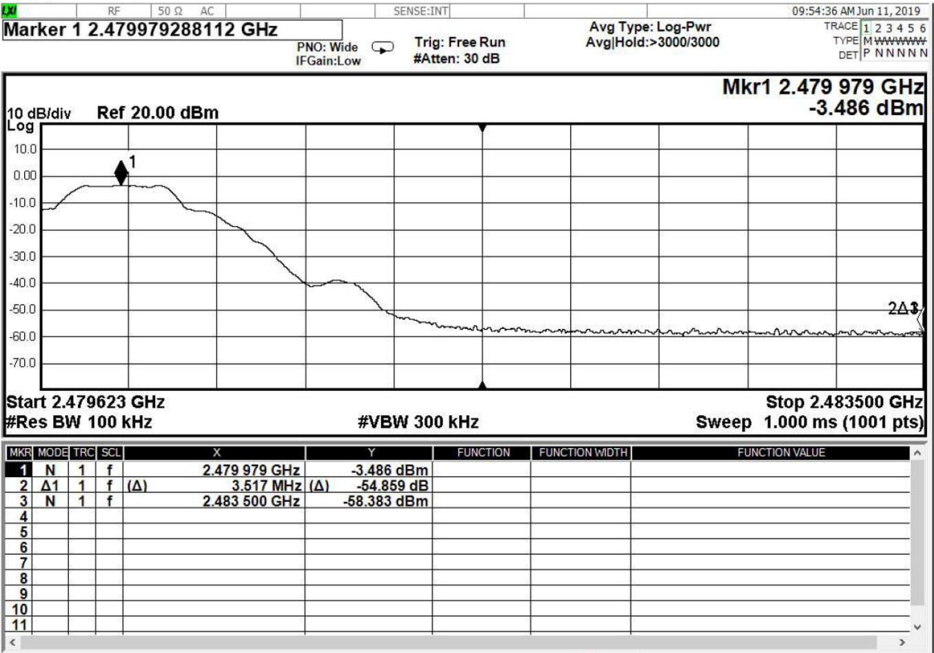
Figure 21 – Band Edge Measurement, High Channel, GFSK
