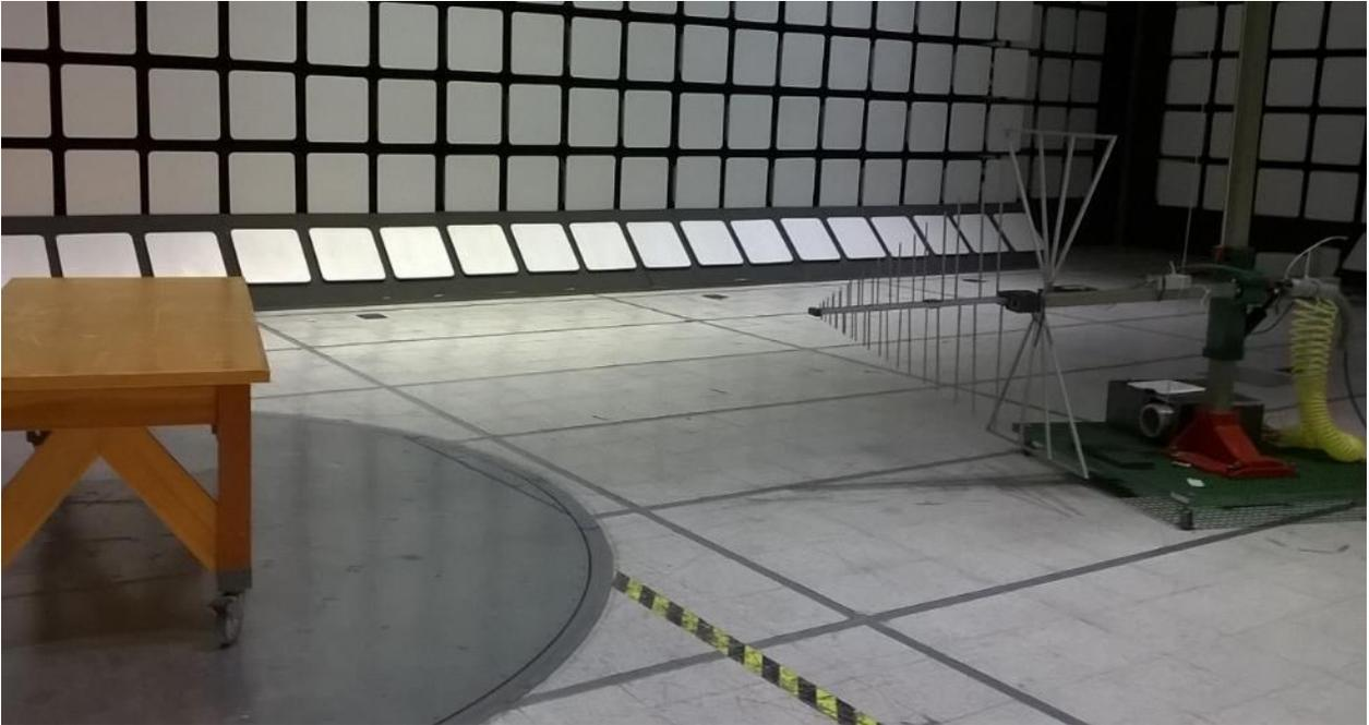
EUT not shown. Photo is intended to show test setup only. 3m, 30 MHz – 1 GHz
