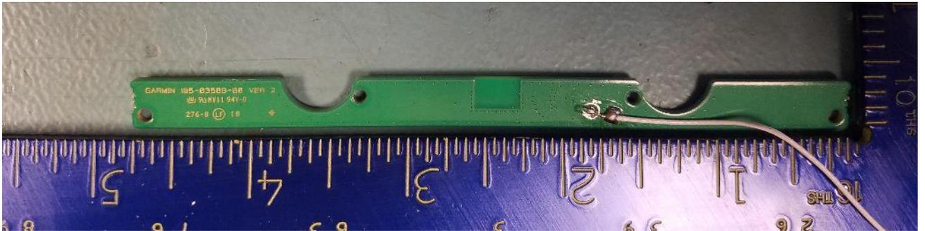
GPS PCB rear, receive antenna
