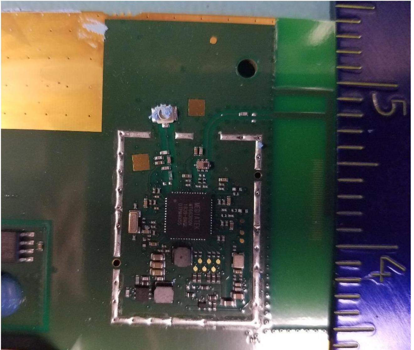
RF Section detail, no shield, A03587 and B03587
