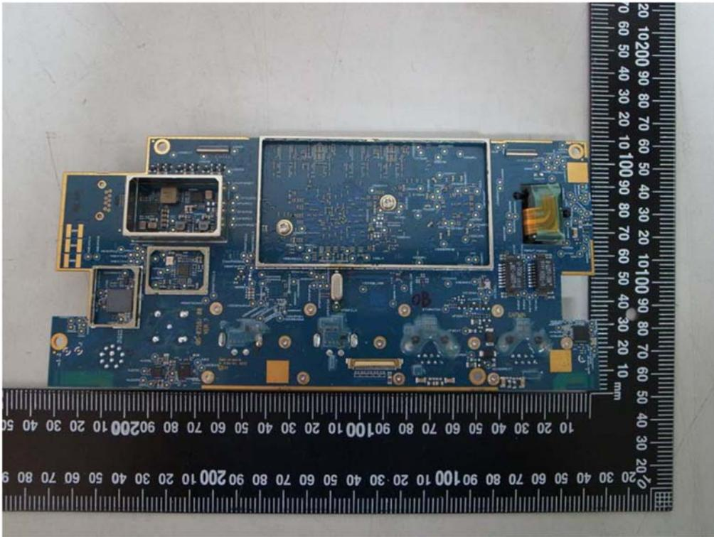
Figure 3 – PCB 1 RF CIRCUITRY (un-Shielded)
