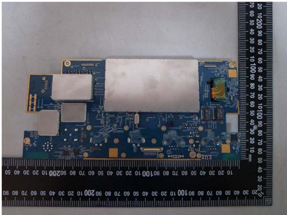
Figure 2 - PCB 1 RF CIRCUITRY (Shielded)
