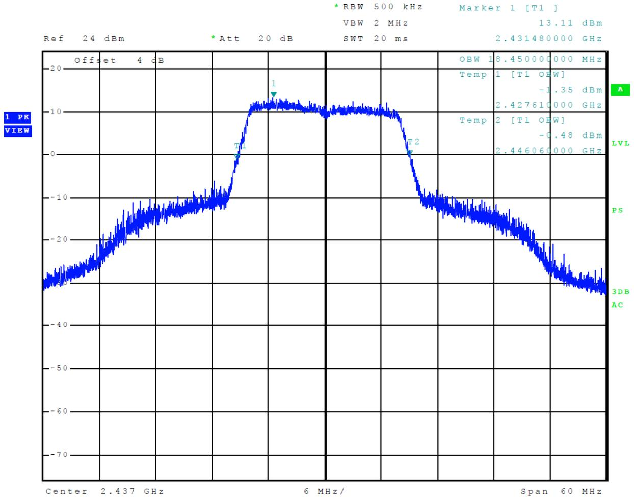
**Figure 27 Plot of 99% Occupied Bandwidth (Mode 5 802.11g)**
