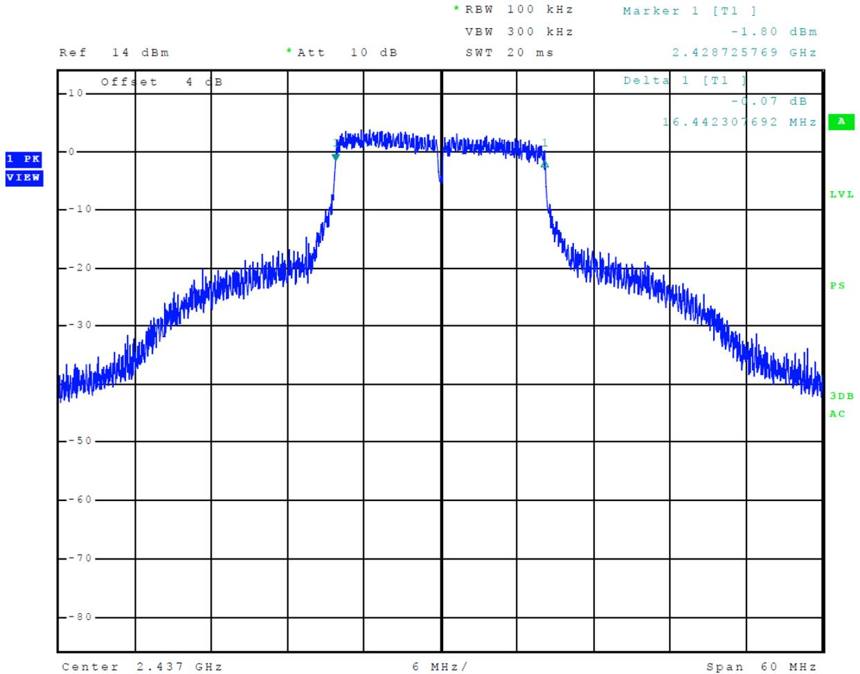
**Figure 26 Plot of 6-dB% Occupied Bandwidth (Mode 5 802.11g)**
