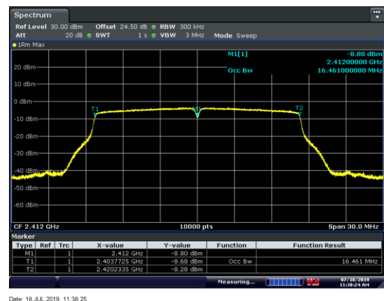
Figure 8.1-10: 99% bandwidth, 2112MHz, 802.11g @ 6Mbps
