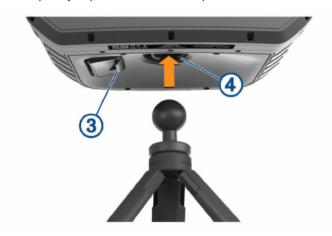
3 While depressing the tripod release lever, insert the tripod ball mount into the socket 4.
