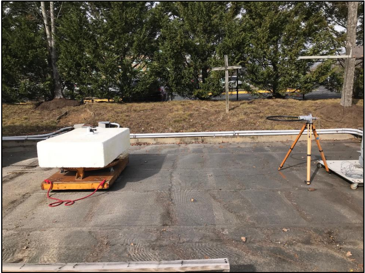
Photograph 3: Radiated Emissions Testing – Side View (Below 1 GHz)
