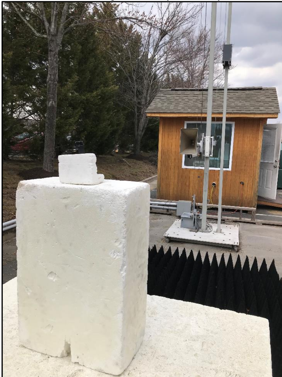
Photograph 2: Radiated Emissions Testing – Back View (Above 1 GHz)
