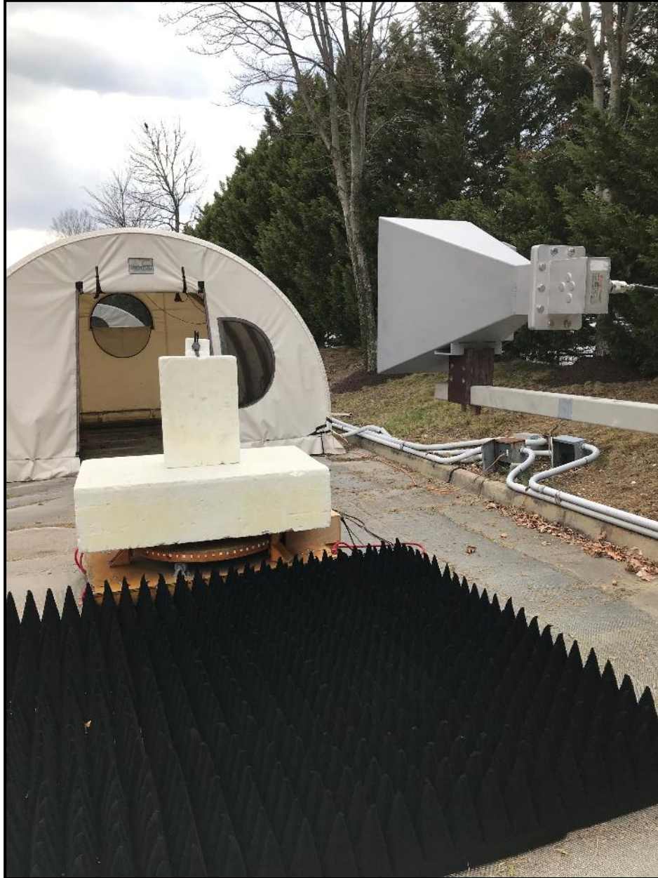
Photograph 1: Radiated Emissions Testing – Front View (Above 1 GHz)
