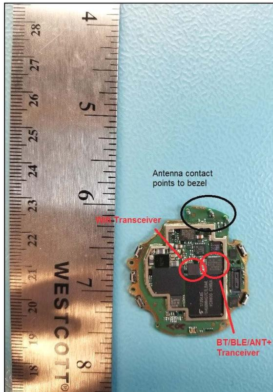
Main Board without Shield – Top View
