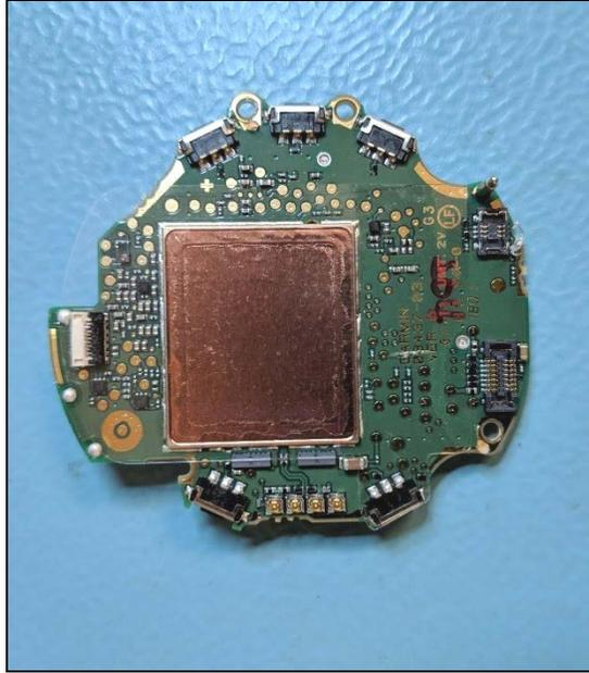
**Main Board with Shield – Bottom View**
