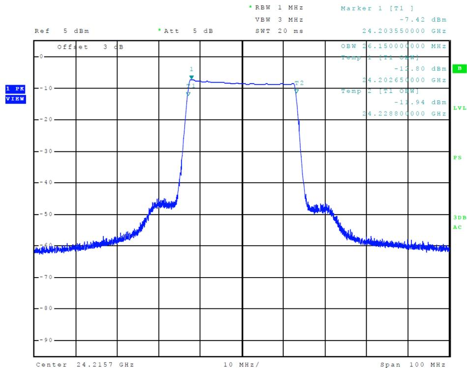
Figure 12 Plot of Transmitter Emissions (99% Occupied Bandwidth, 25 MHz Chnl, 24 GHz)
