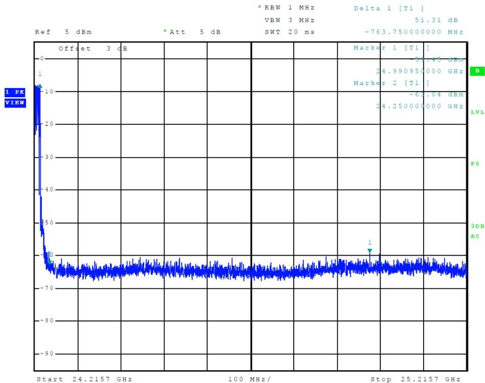
Figure 14 Plot of Transmitter Emissions (High Band Edge, 25 MHz Chnl, 24 GHz)
