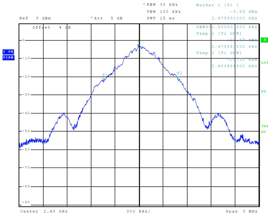
**Figure 8 Plot of Transmitter Emissions (99% Occupied Bandwidth, 2400 MHz Band)**
