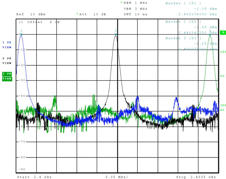
**Figure 7 Plot of Transmitter Emissions (Operation in 2402-2480 MHz)**
