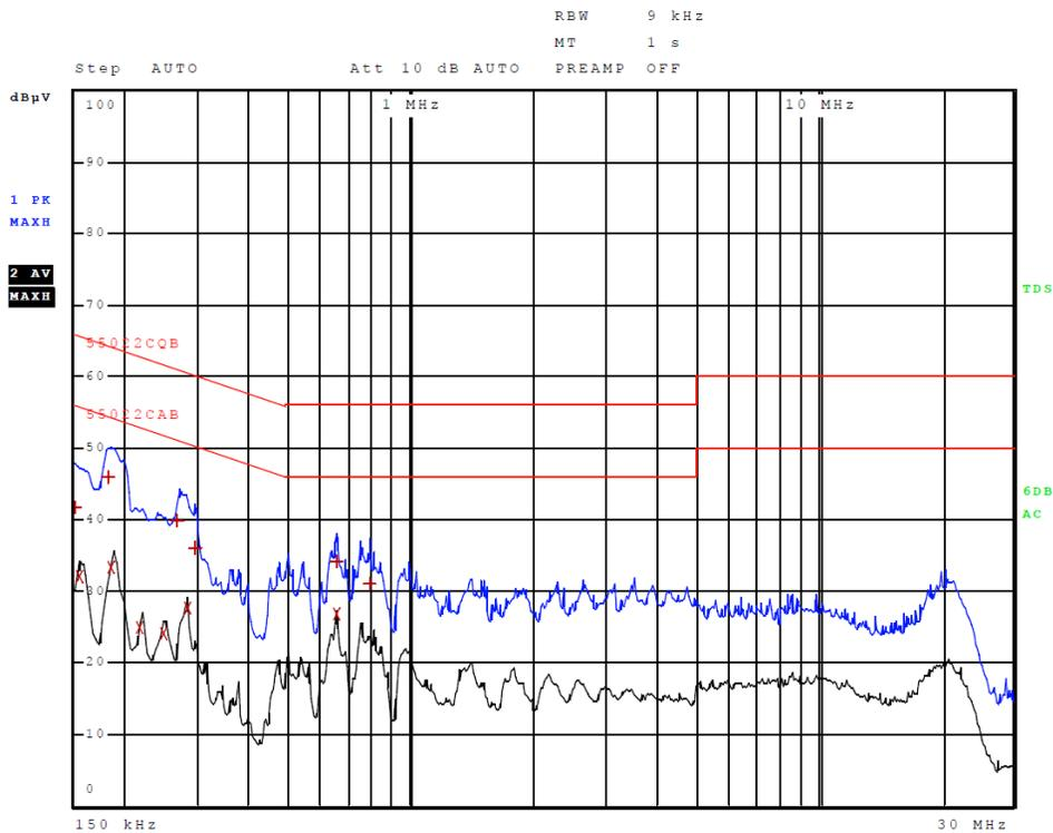
Figure 4 AC Line Conducted emissions of EUT line 2 (EUT – 362-00087-00)
