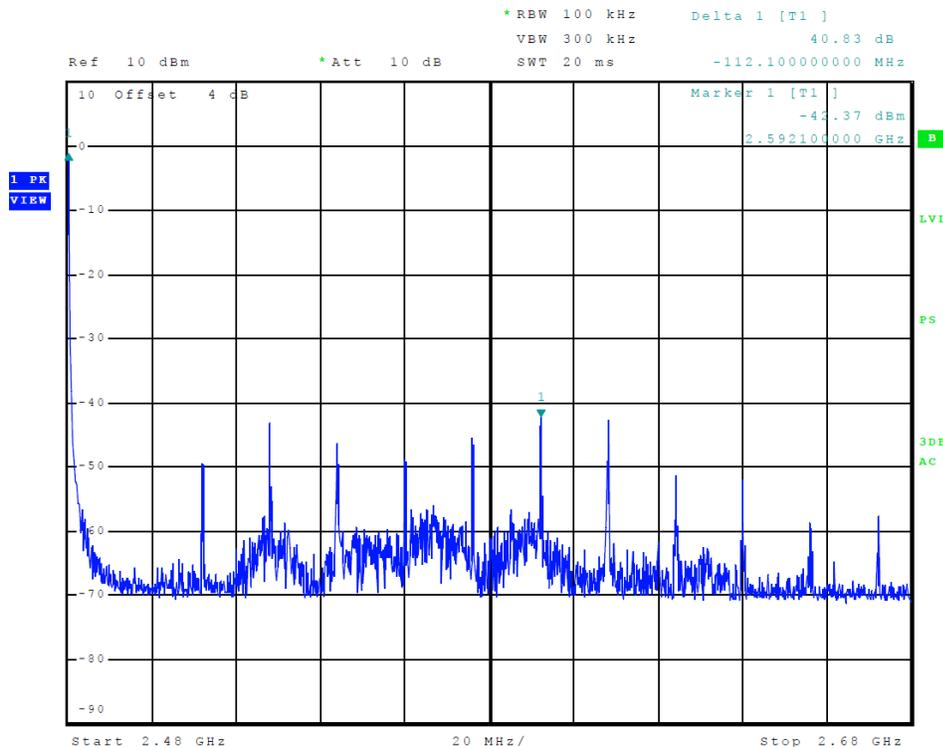
**Figure 10 Plot of Transmitter Emissions (High Band Edge, 2400 MHz Band)**
