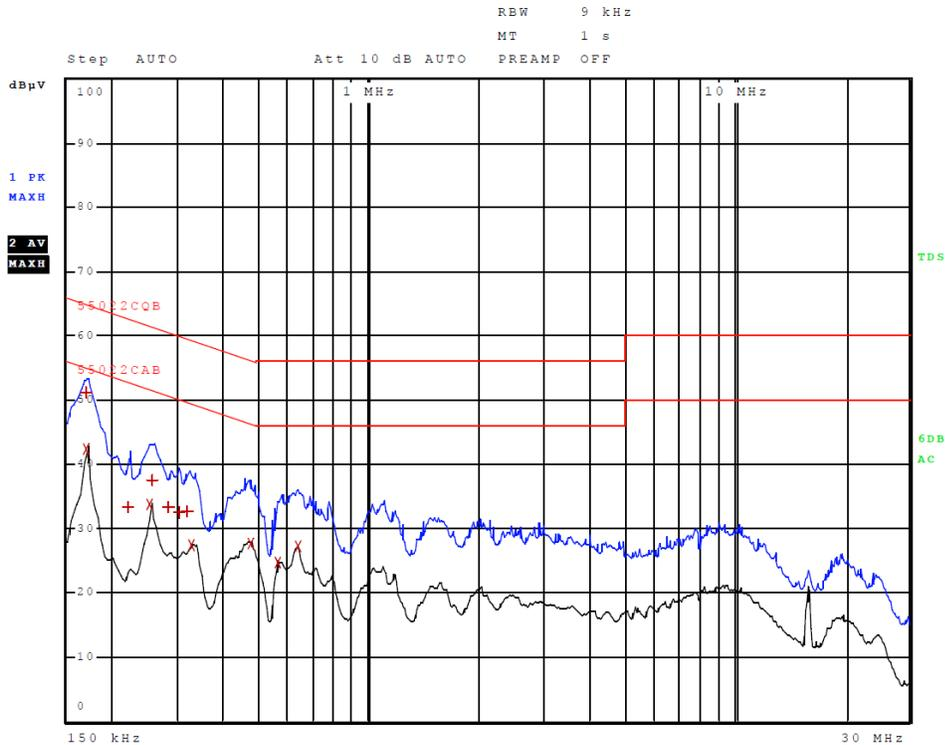
Figure 1 AC Line Conducted emissions of EUT line 1 (EUT – 362-00086-01)
