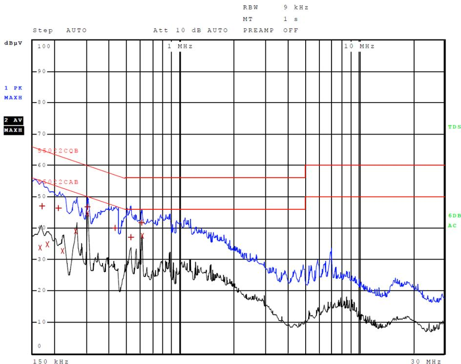
Figure 6 AC Line Conducted emissions of EUT line 2 (#4, EUT – Computer)
