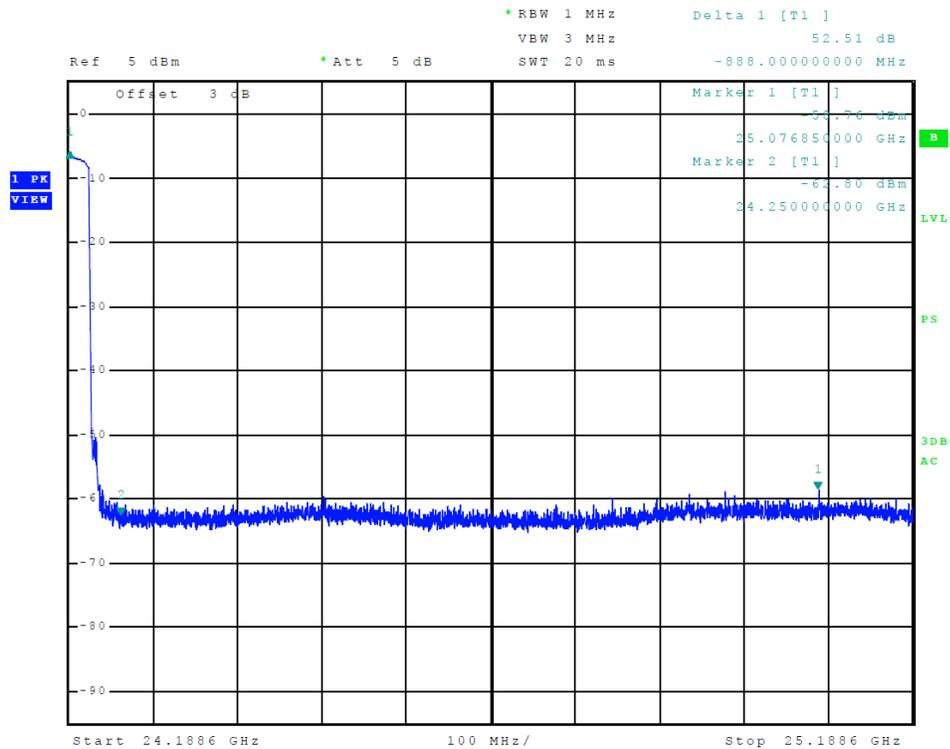
**Figure 18 Plot of Transmitter Emissions (High Band Edge, 50 MHz Chnl, 24 GHz)**
