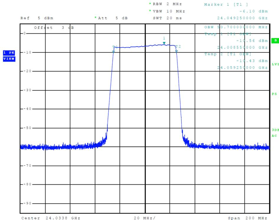
Figure 16 Plot of Transmitter Emissions (99% Occupied Bandwidth, 50 MHz Chnl, 24 GHz)
