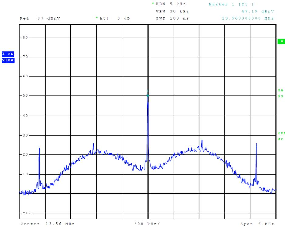
**Figure 5 Plot of NFC Operation Across Frequency Spectrum**
