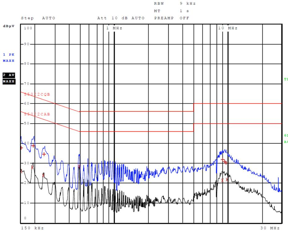
**Figure 1 AC Line Conducted emissions of EUT line 1 (#2, EUT – 362-00091-00)**
