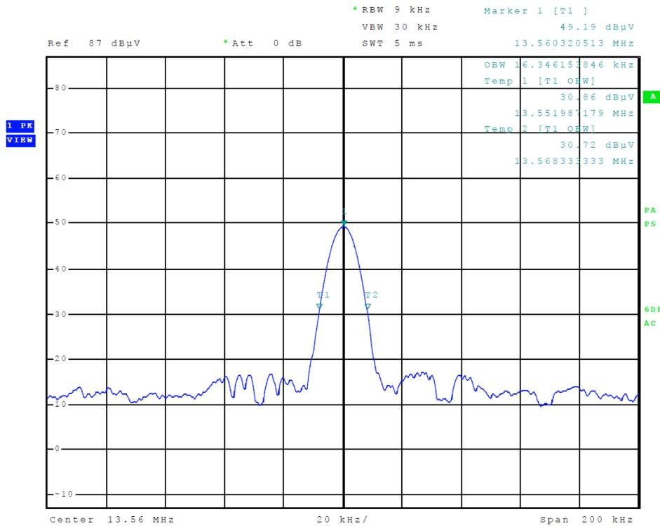
**Figure 7 Plot of NFC 99 percent Occupied Bandwidth**
