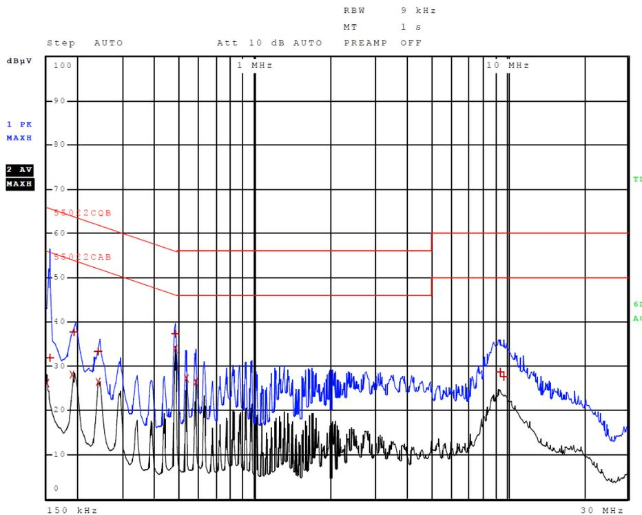
**Figure 2 AC Line Conducted emissions of EUT line 2 (#2, EUT – 362-00091-00)**
