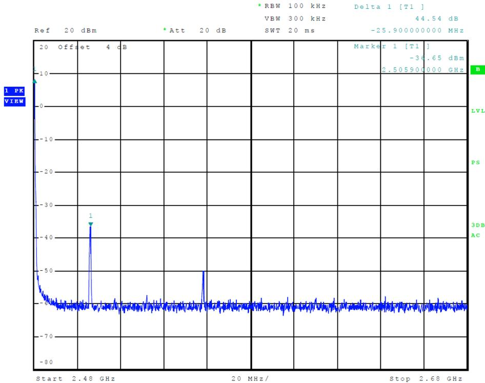
**Figure 17 Plot of Upper Band Edge (ANT-Mode 1)**
