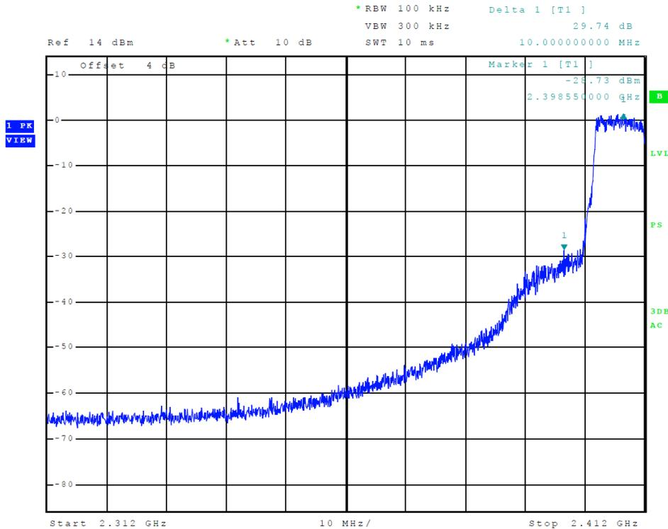
**Figure 15 Plot of Lower Band Edge (802.11 g-mode)**
