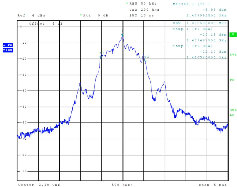
**Figure 6 Plot of Transmitter Emissions (99% Occupied Bandwidth, BLE)**
