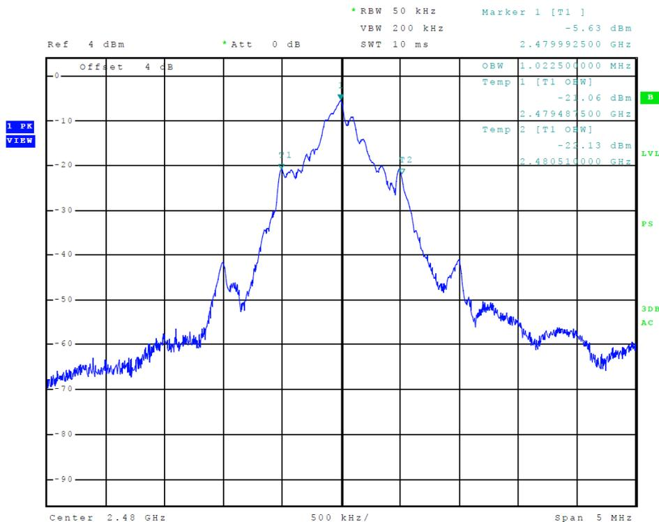
Figure 2 Plot of Transmitter Emissions (99% Occupied Bandwidth, ANT)
