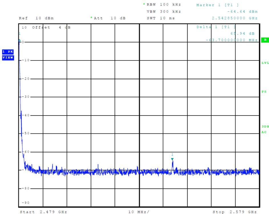
**Figure 4 Plot of Transmitter Emissions (High Band Edge, ANT GFSK)**
