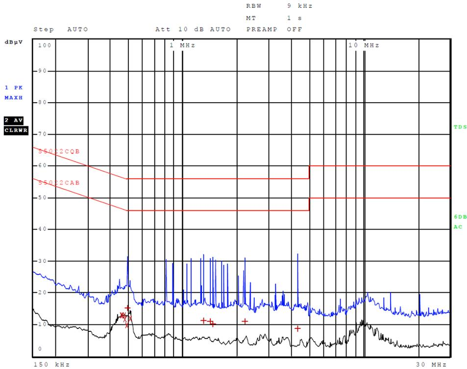
Figure 3 AC Line Conducted emissions of EUT line 1 (#3, EUT – 320-00091-00)
