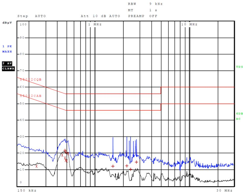
Figure 4 AC Line Conducted emissions of EUT line 2 (#3, EUT – 320-00091-00)
