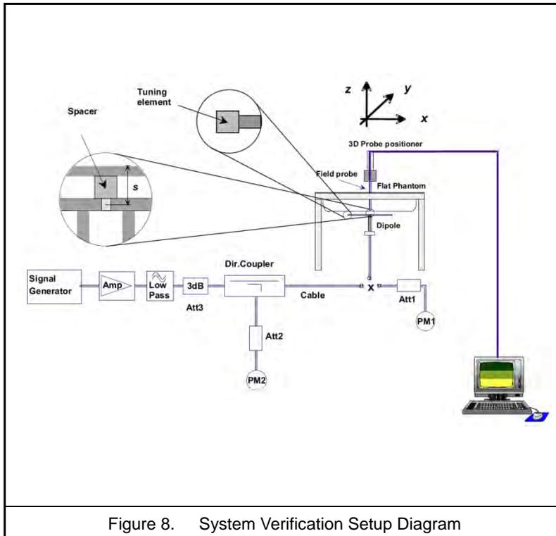
Figure 8. System Verification Setup Diagram
