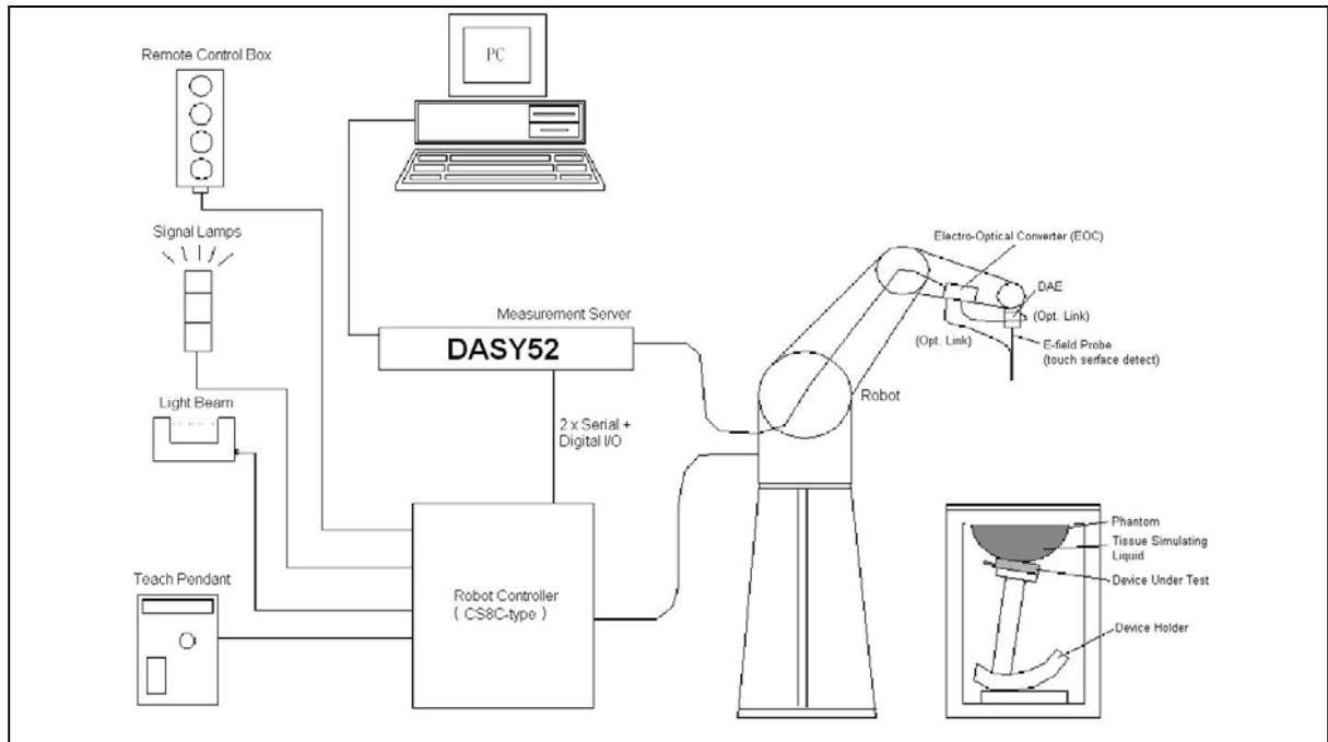
The DASY52 system for performing compliance tests consists of the following items:
