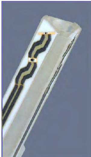
Figure 3. E-field Probe
