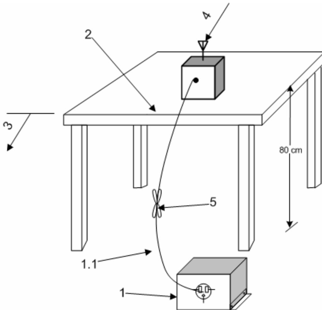
1—A LISN is optional for radiated measurements between 30 MHz and 1000 MHz but not allowed for measurements below 30 MHz and above 1000 MHz (see 6.3.1). If used, then connect EUT to one LISN. Unused LISN measuring port connectors shall be terminated in 50  $\Omega$  loads. The LISN may be placed on top of, or immediately beneath, the reference ground plane (see 6.2.2 and 6.2.3.2).
