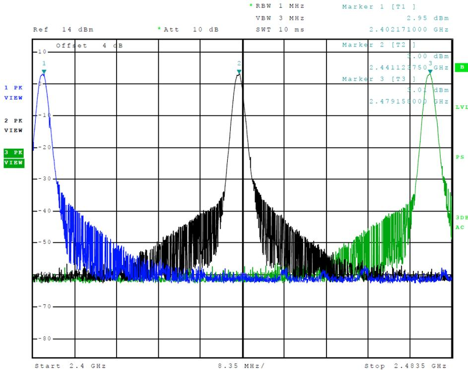
**Figure 3 Plot of Transmitter Emissions (Operation in 2402-2479 MHz)**
