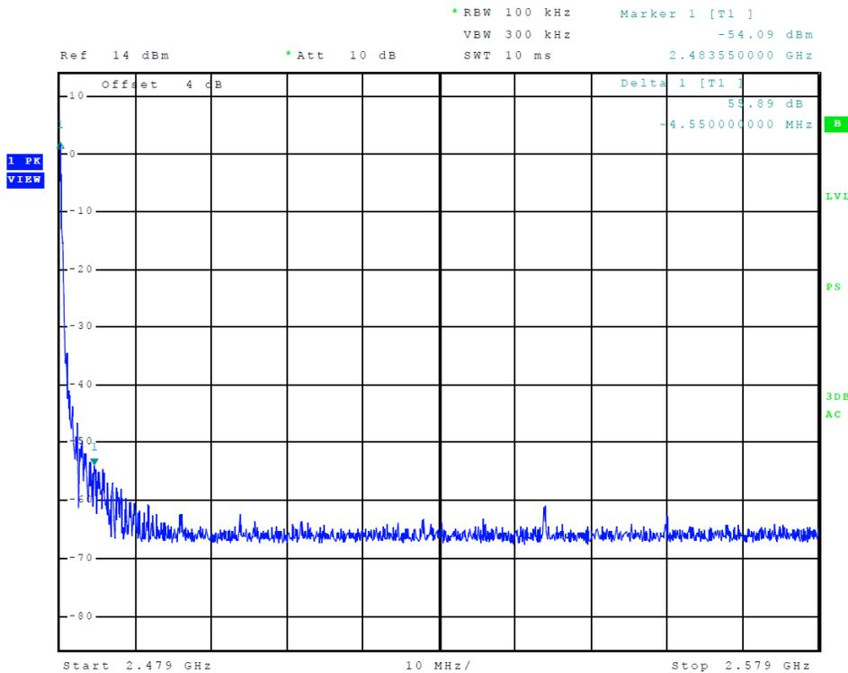
Figure 6 Plot of Transmitter Emissions (High Band Edge)
