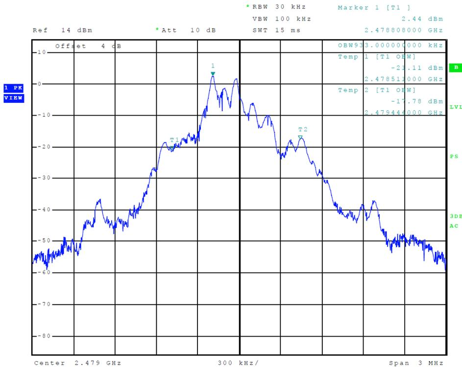
**Figure 4 Plot of Transmitter Emissions (99% Occupied Bandwidth)**
