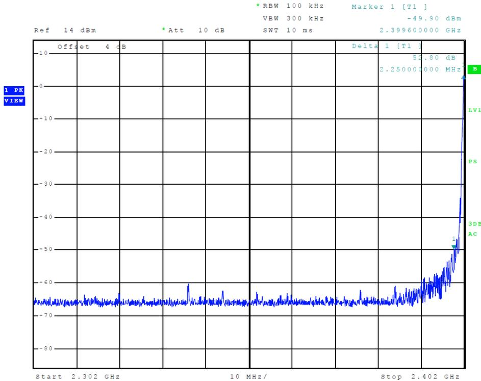
Figure 5 Plot of Transmitter Emissions (Low Band Edge)
