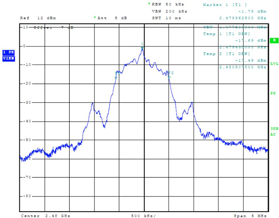
Figure 16 Plot of Transmitter Emissions (BLE 0x55, 99% Occupied Bandwidth)
