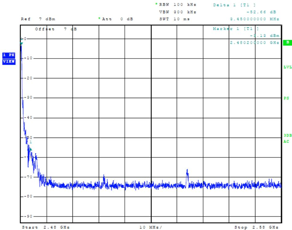
Figure 14 Plot of Transmitter Emissions (BLE 0x0F, High Band Edge)
