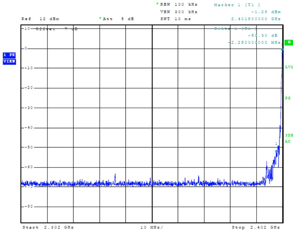
Figure 5 Plot of Transmitter Emissions (GFSK, Low Band Edge)
