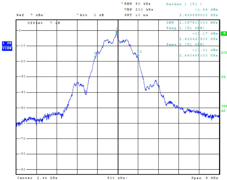
Figure 8 Plot of Transmitter Emissions (PRB29, 99% Occupied Bandwidth)
