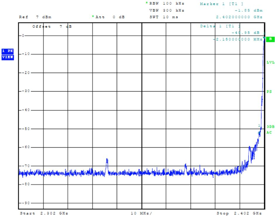
Figure 9 Plot of Transmitter Emissions (PRB29, Low Band Edge)
