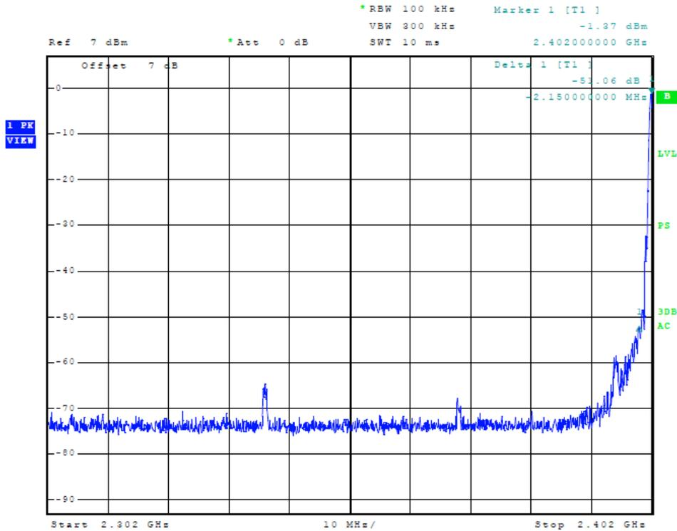
Figure 13 Plot of Transmitter Emissions (BLE 0x0F, PSK, Low Band Edge)
