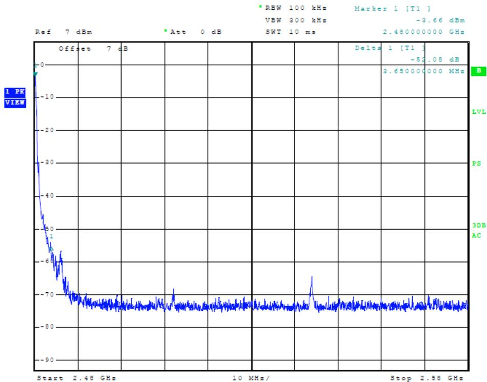
Figure 18 Plot of Transmitter Emissions (BLE 0x55, High Band Edge)
