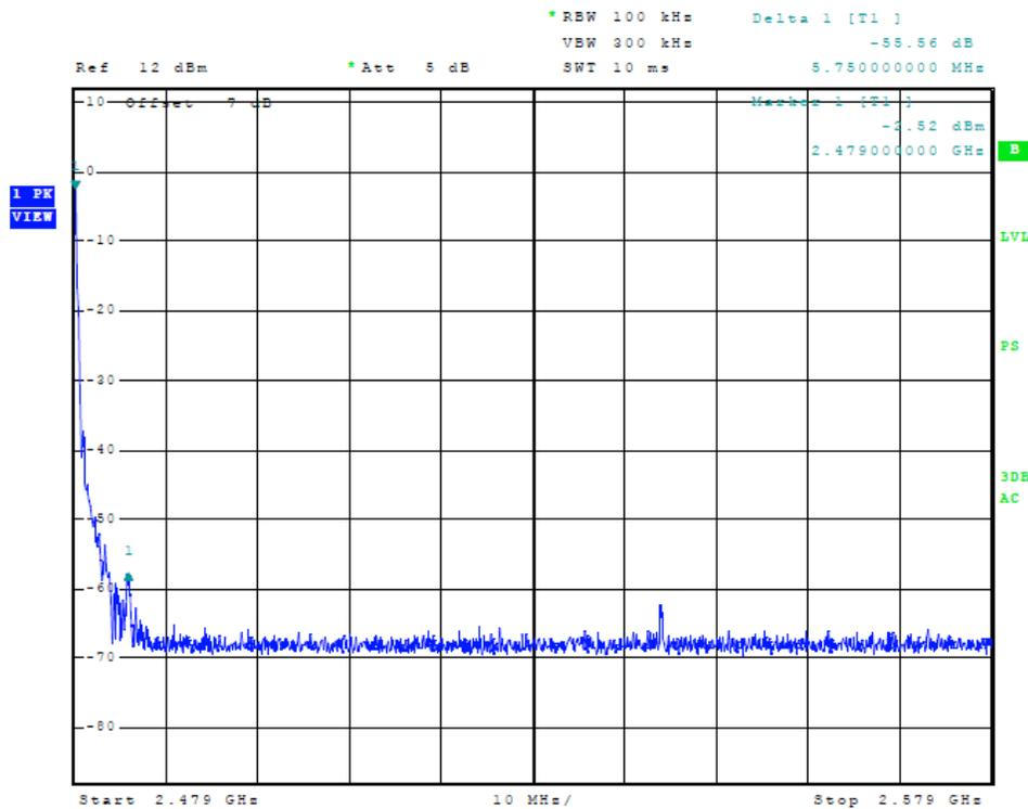
Figure 6 Plot of Transmitter Emissions (GFSK, High Band Edge)
