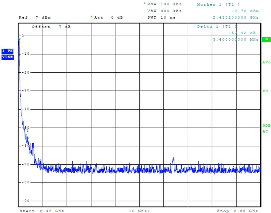
Figure 10 Plot of Transmitter Emissions (PRB29, High Band Edge)
