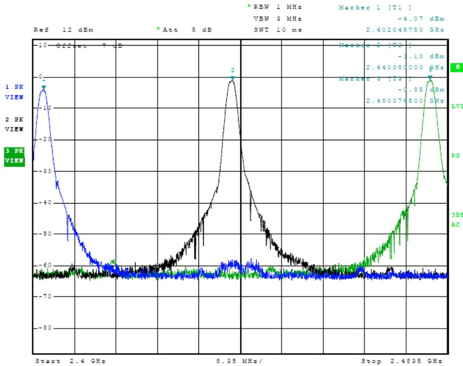
Figure 7 Plot of Transmitter Emissions (PRB29, Operation in 2402-2480 MHz)
