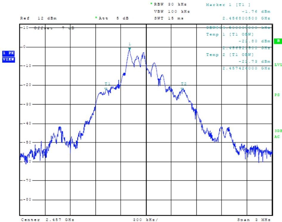
Figure 4 Plot of Transmitter Emissions (GFSK, 99% Occupied Bandwidth)
