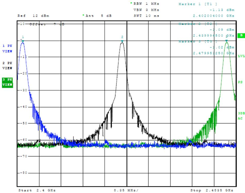
Figure 11 Plot of Transmitter Emissions (BLE 0x0F, Operation in 2402-2480 MHz)
