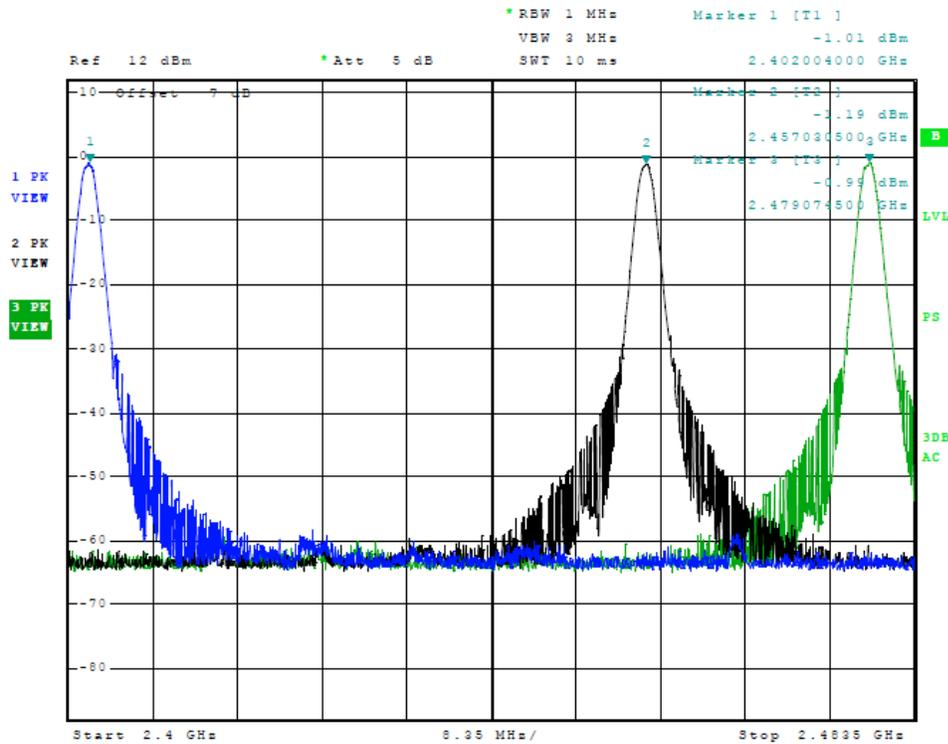
Figure 3 Plot of Transmitter Emissions (GFSK, Operation in 2402-2480 MHz)
