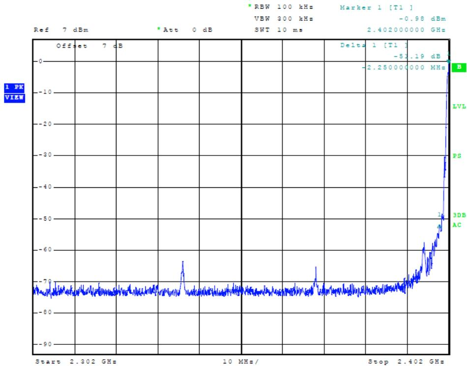
Figure 17 Plot of Transmitter Emissions (BLE 0x55, PSK, Low Band Edge)
