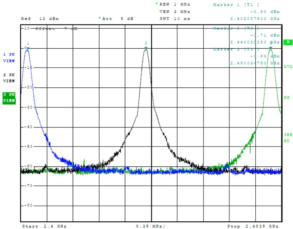
Figure 15 Plot of Transmitter Emissions (BLE 0x55, Operation in 2402-2480 MHz)
