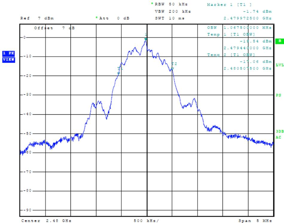
Figure 12 Plot of Transmitter Emissions (BLE 0x0F, 99% Occupied Bandwidth)
