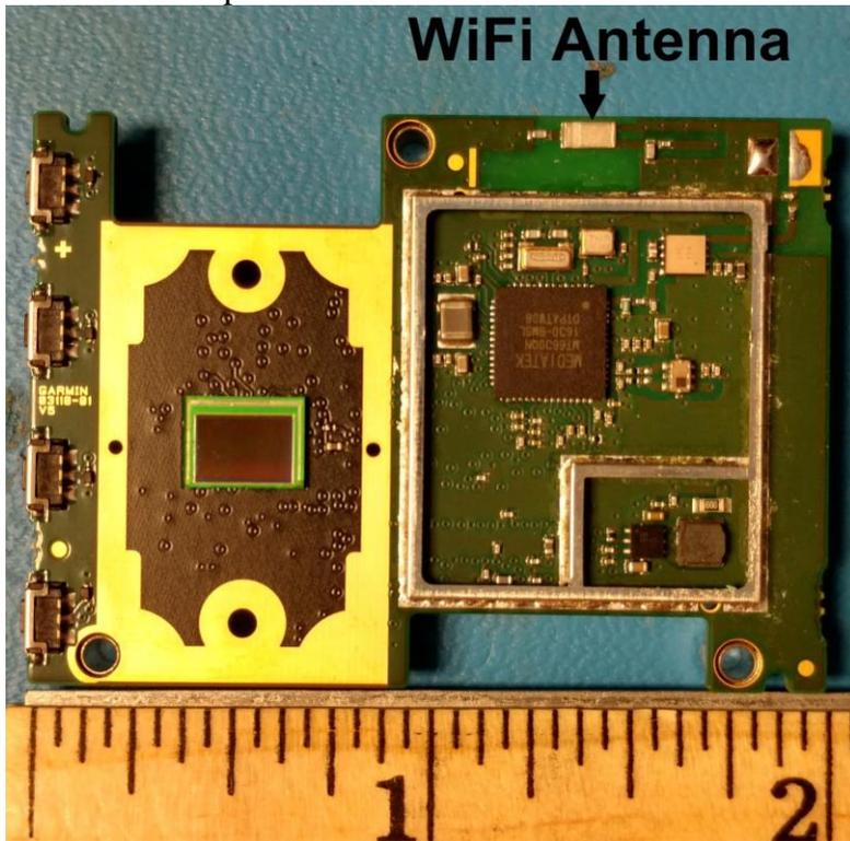
Sensor board with camera and shield
