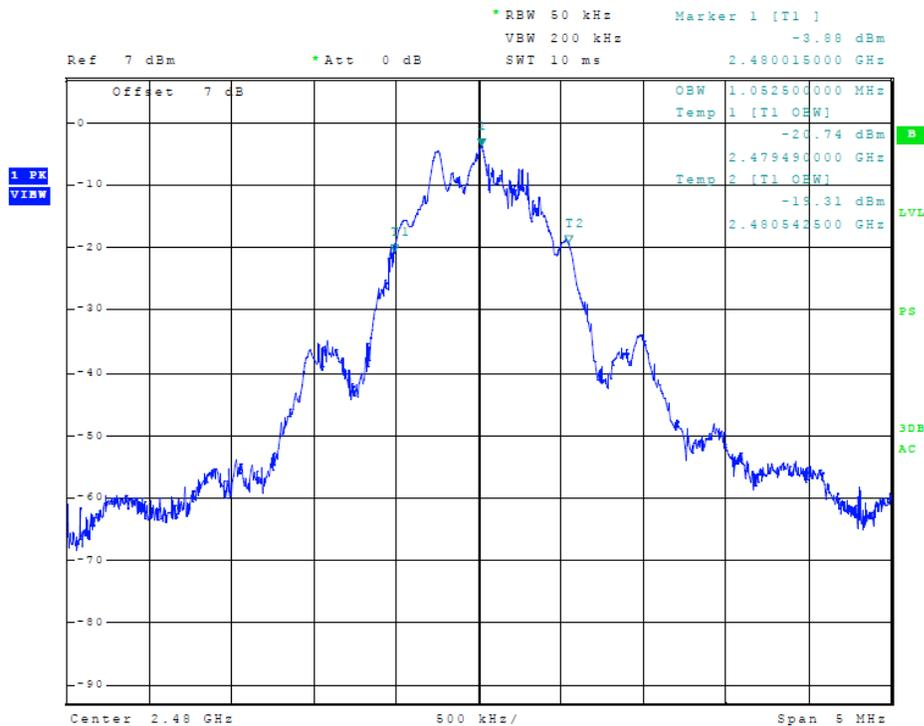
Figure 10 Plot of Transmitter Emissions (99% Occupied Bandwidth, PRB29)
