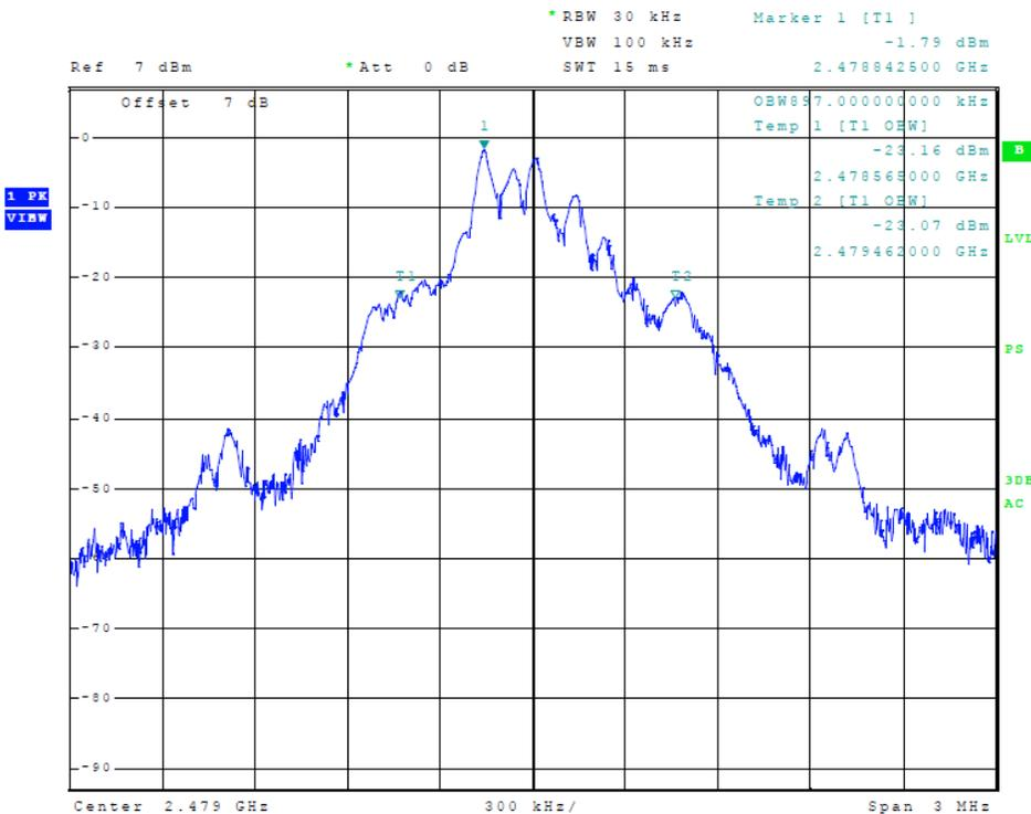
**Figure 6 Plot of Transmitter Emissions (99% Occupied Bandwidth, GFSK)**
