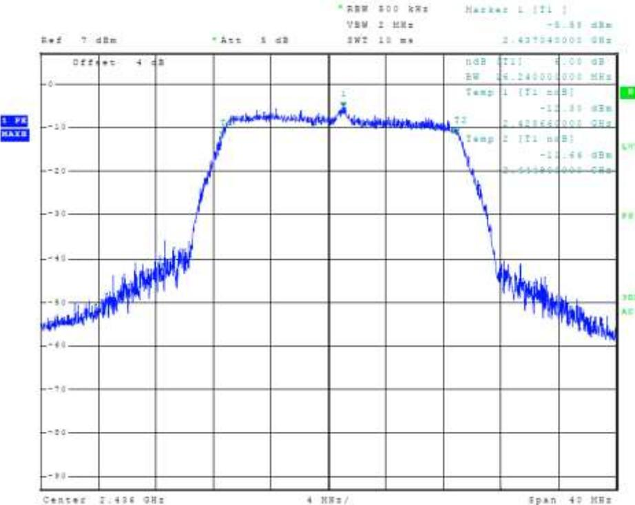
Figure 18 Plot of Transmitter 6-dB Occupied Bandwidth (802.11 g-mode)
