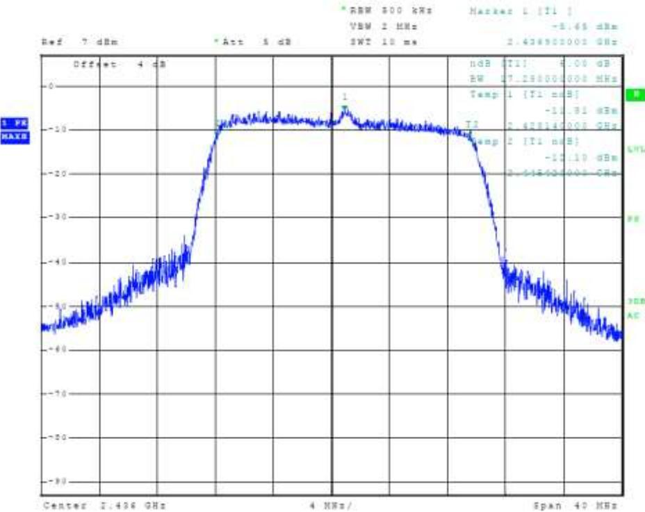
Figure 20 Plot of Transmitter 6-dB Occupied Bandwidth (802.11 n-mode)
