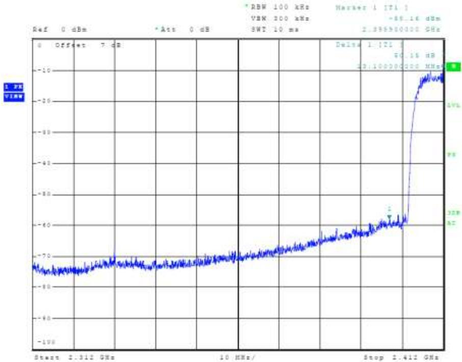
**Figure 10 Plot of Lower Band Edge (802.11 b-mode)**
