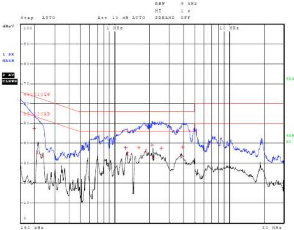
Figure 3 AC Line Conducted emissions of EUT line 1 (#3, EUT - CPU)
