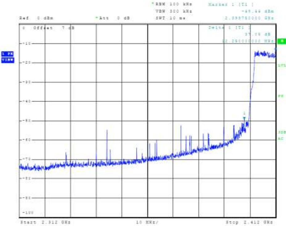
Figure 11 Plot of Lower Band Edge (802.11 g-mode)
