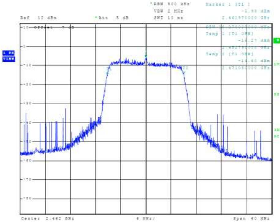
**Figure 21 Plot of Transmitter 99% Occupied Bandwidth (802.11 n-mode)**
