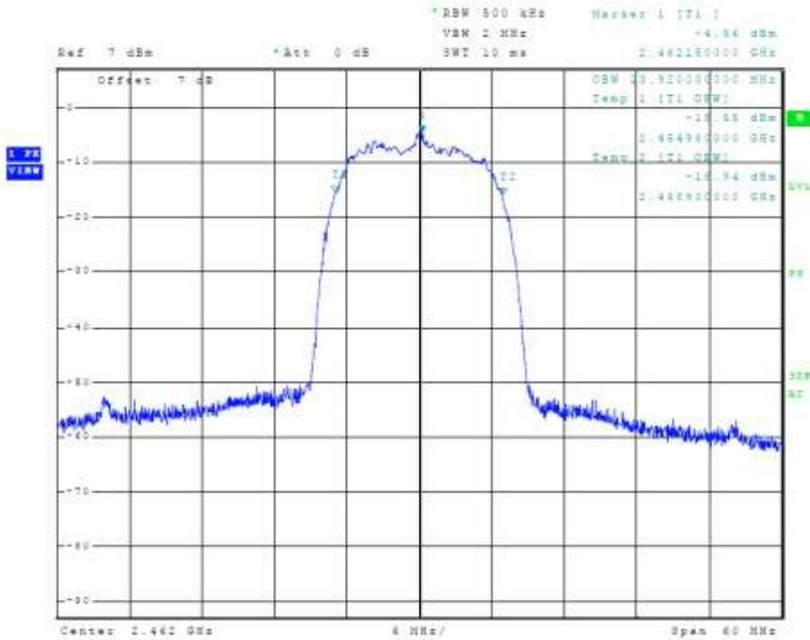
Figure 17 Plot of Transmitter 99% Occupied Bandwidth (802.11 b-mode)
