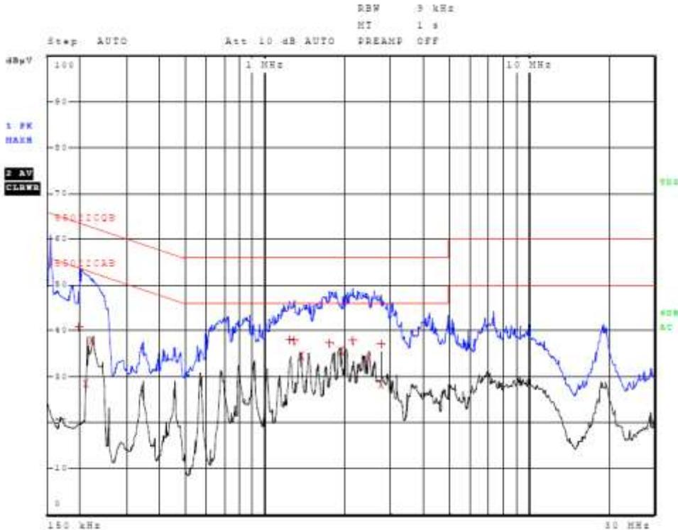
Figure 4 AC Line Conducted emissions of EUT line 2 (#3, EUT - CPU)
