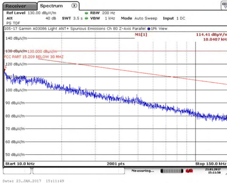
A.15.6. Measurement Results – DUT Position: Z–Axis, Perpendicular Antenna
