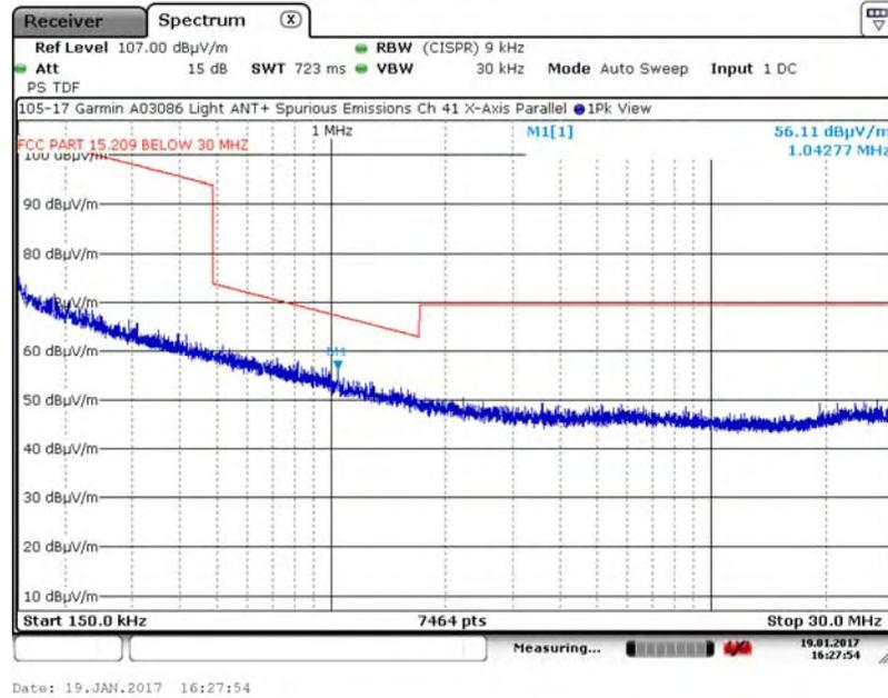
A.9.2. Measurement Results – DUT Position: X–Axis, Perpendicular Antenna
