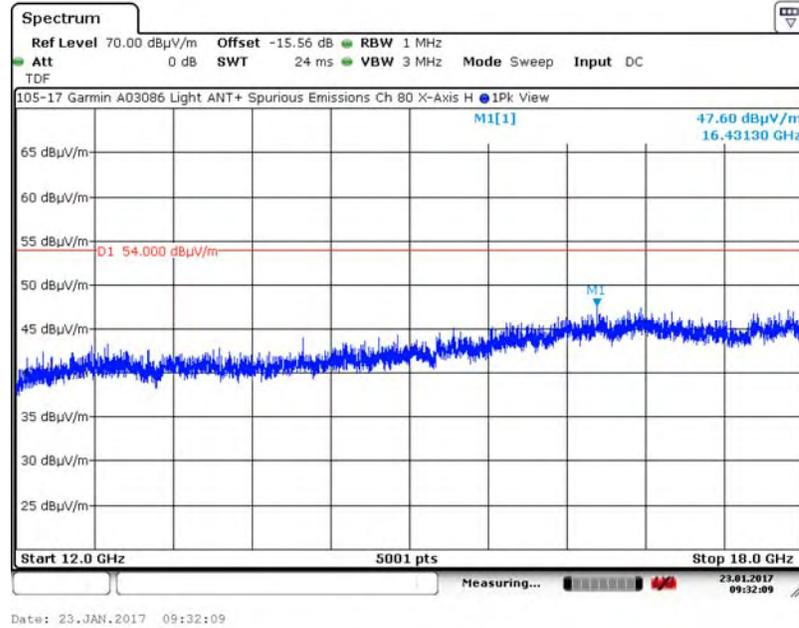
A.20.2. Measurement Results – DUT Position: X–Axis, Vertical Antenna
