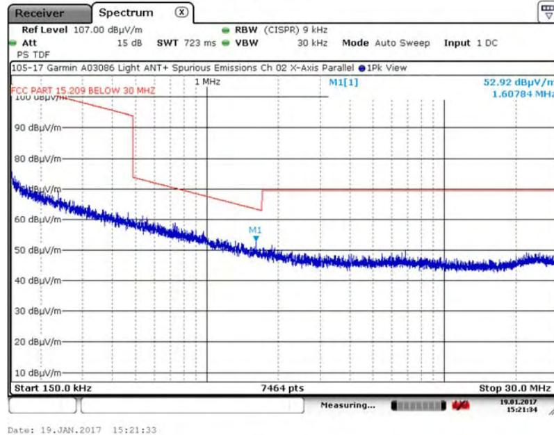
A.2.2. Measurement Results – DUT Position: X-Axis, Perpendicular Antenna
