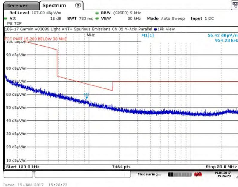
A.2.4. Measurement Results – DUT Position: Y–Axis, Perpendicular Antenna
