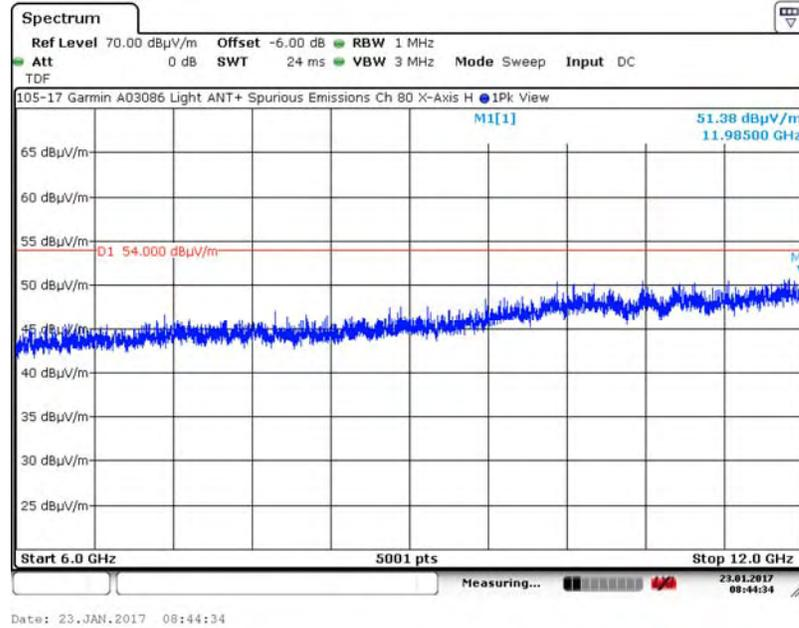
A.19.2. Measurement Results – DUT Position: X–Axis, Vertical Antenna
