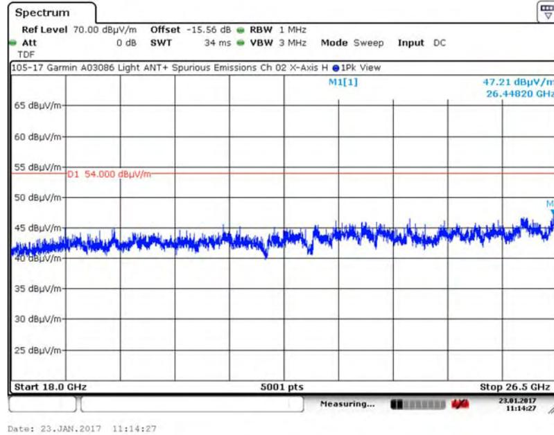
A.7.2. Measurement Results – DUT Position: X–Axis, Vertical Antenna
