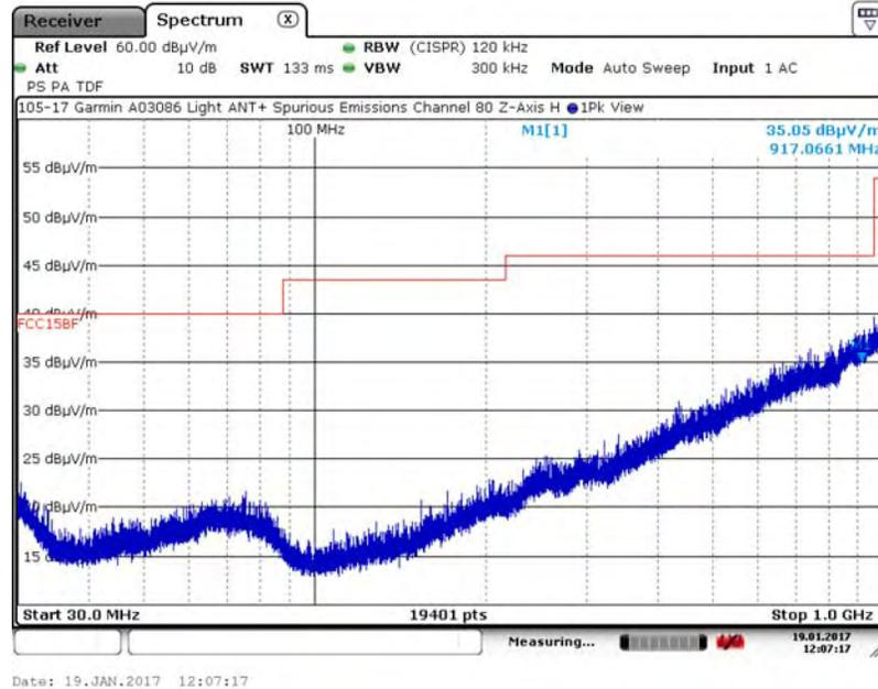
A.17.6. Measurement Results – DUT Position: Z-Axis, Vertical Antenna
