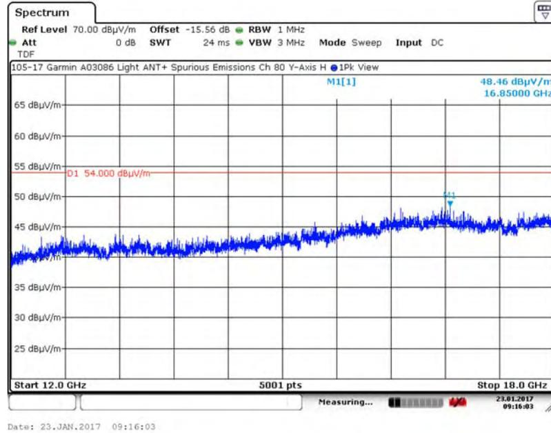
A.20.4. Measurement Results – DUT Position: Y–Axis, Vertical Antenna
