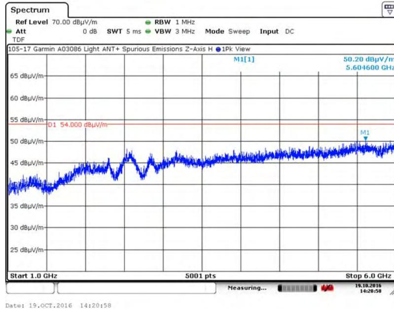
A.11.6. Measurement Results – DUT Position: Z-Axis, Vertical Antenna
