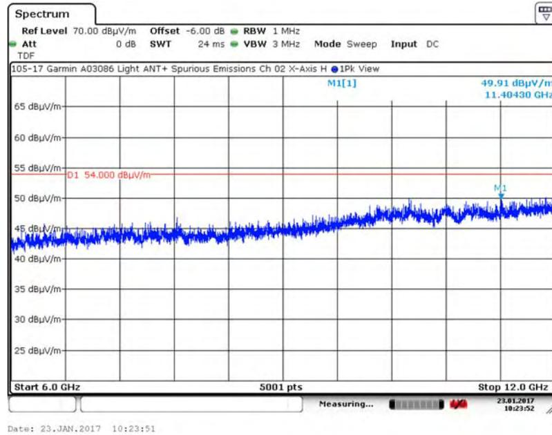
A.5.2. Measurement Results – DUT Position: X–Axis, Vertical Antenna
