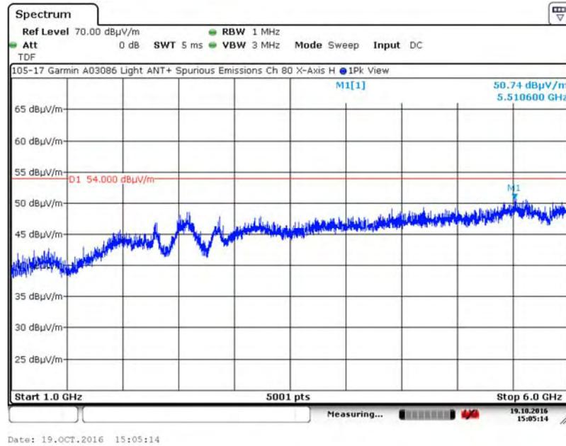
A.18.2. Measurement Results – DUT Position: X–Axis, Vertical Antenna
