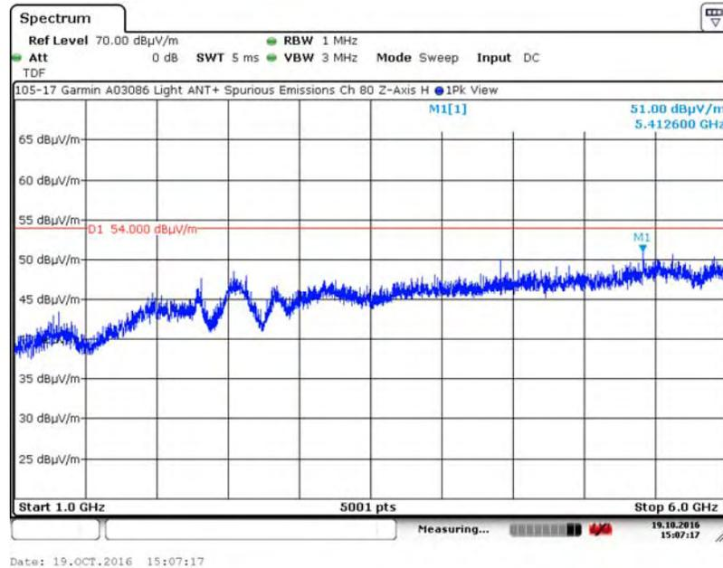
A.18.6. Measurement Results – DUT Position: Z-Axis, Vertical Antenna
