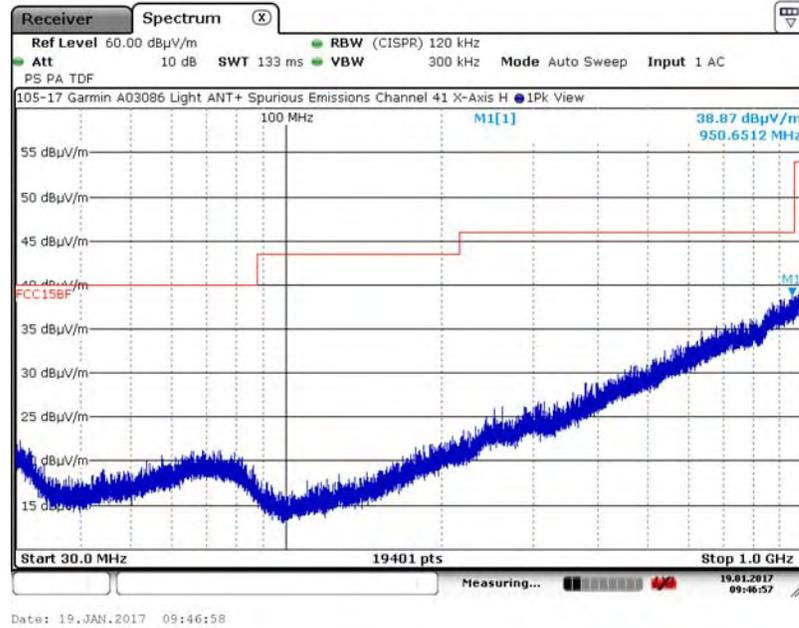
A.10.2. Measurement Results – DUT Position: X–Axis, Vertical Antenna
