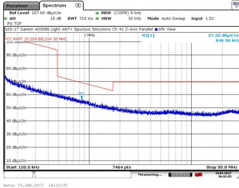
A.9.6. Measurement Results – DUT Position: Z–Axis, Perpendicular Antenna
