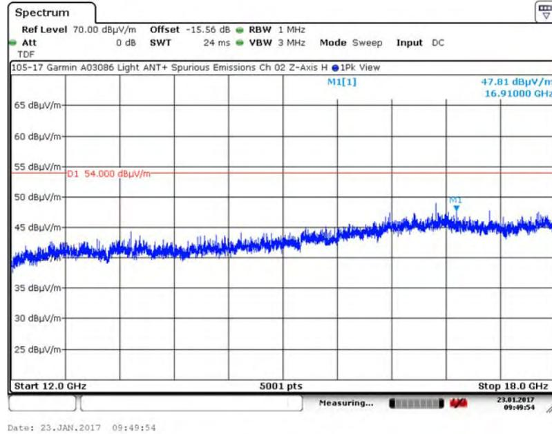
A.6.6. Measurement Results – DUT Position: Z–Axis, Vertical Antenna
