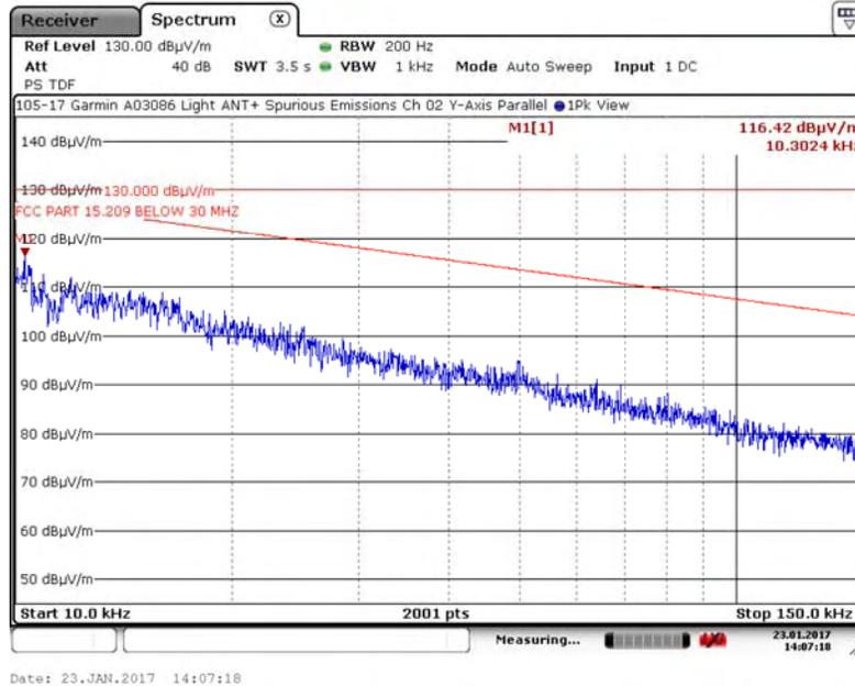
A.1.4. Measurement Results – DUT Position: Y– Axis, Perpendicular Antenna
