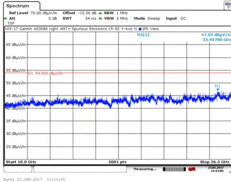
A.7.4. Measurement Results – DUT Position: Y–Axis, Vertical Antenna
