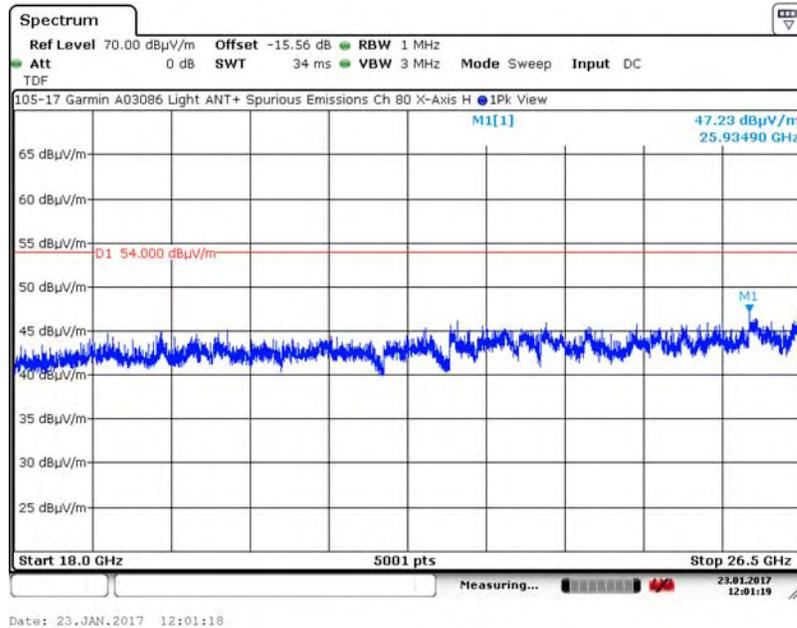
A.21.2. Measurement Results – DUT Position: X–Axis, Vertical Antenna
