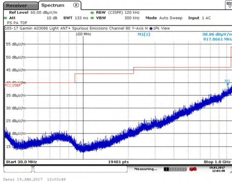
A.17.4. Measurement Results – DUT Position: Y–Axis, Vertical Antenna
