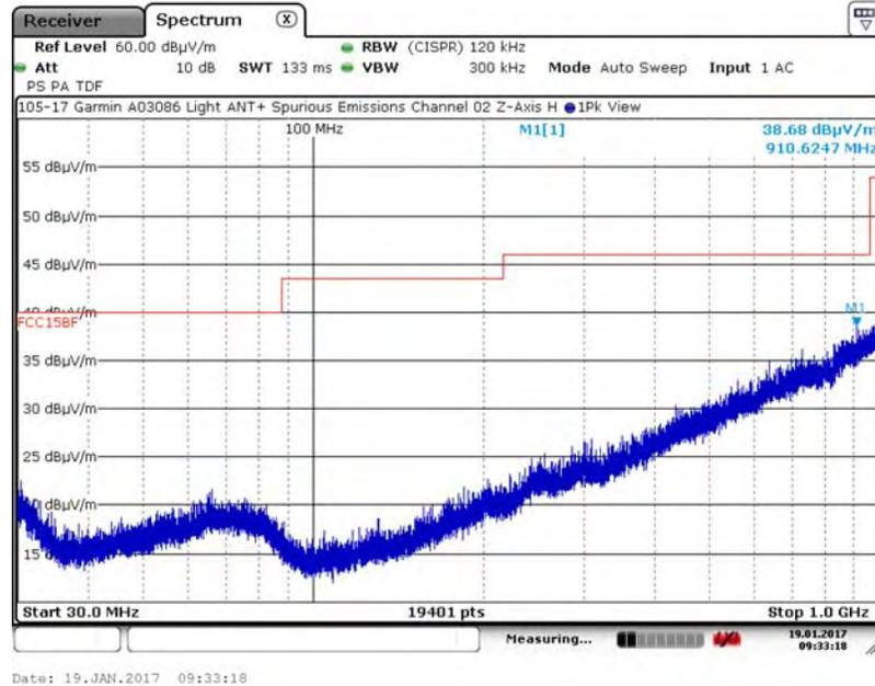
A.3.6. Measurement Results – DUT Position: Z-Axis, Vertical Antenna
