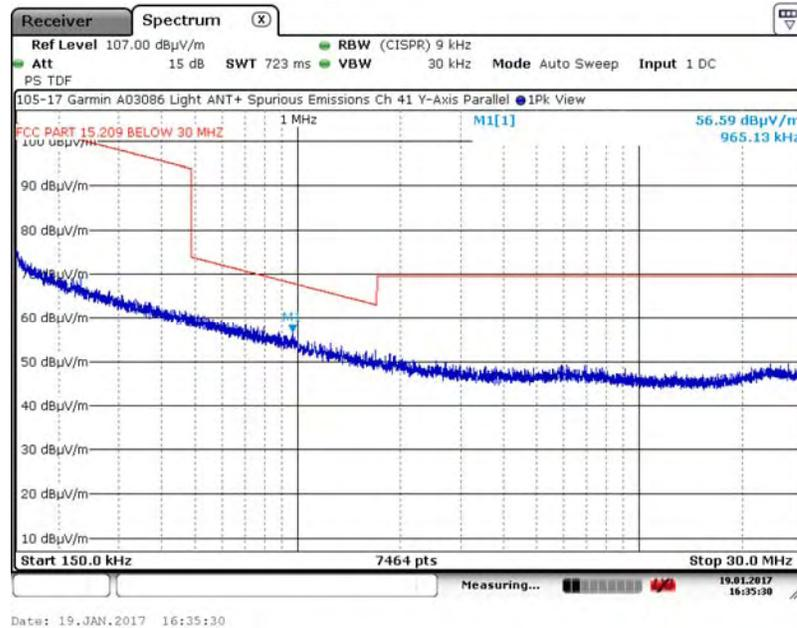
A.9.4. Measurement Results – DUT Position: Y–Axis, Perpendicular Antenna
