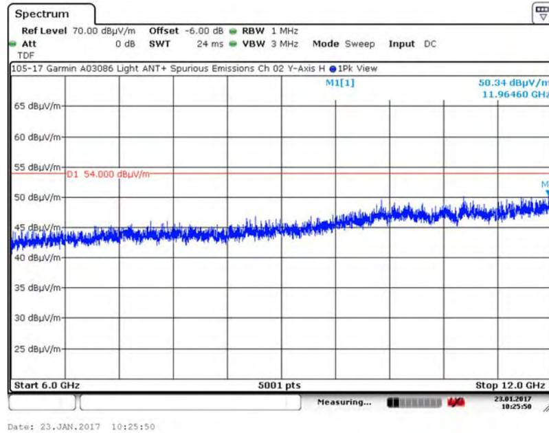
A.5.4. Measurement Results – DUT Position: Y–Axis, Vertical Antenna
