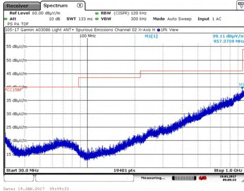
A.3.2. Measurement Results – DUT Position: X–Axis, Vertical Antenna
