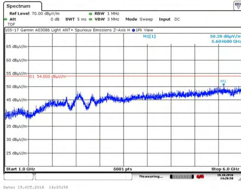
A.4.6. Measurement Results – DUT Position: Z–Axis, Vertical Antenna
