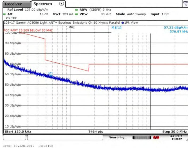
A.16.2. Measurement Results – DUT Position: X–Axis, Perpendicular Antenna
