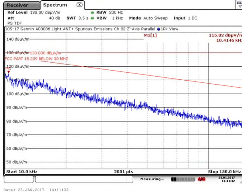
A.1.6. Measurement Results – DUT Position: Z–Axis, Perpendicular Antenna
