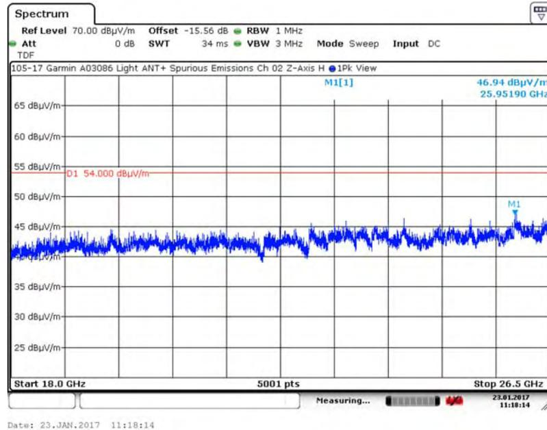
A.7.6. Measurement Results – DUT Position: Z–Axis, Vertical Antenna
