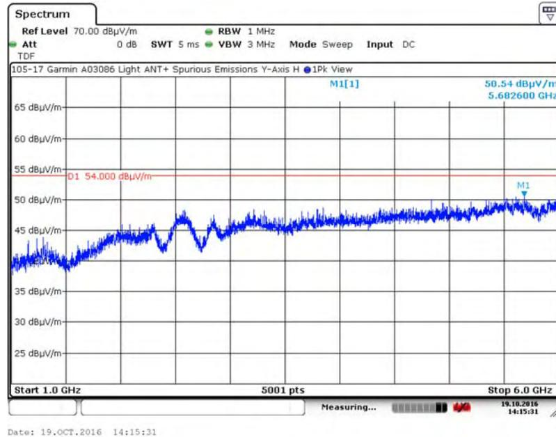
A.11.4. Measurement Results – DUT Position: Y–Axis, Vertical Antenna
