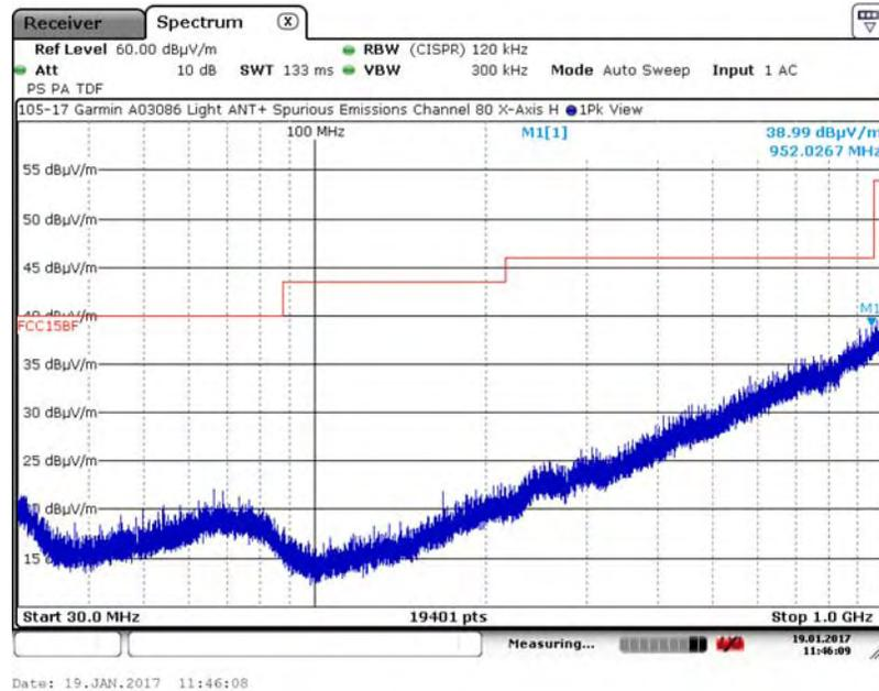
A.17.2. Measurement Results – DUT Position: X–Axis, Vertical Antenna
