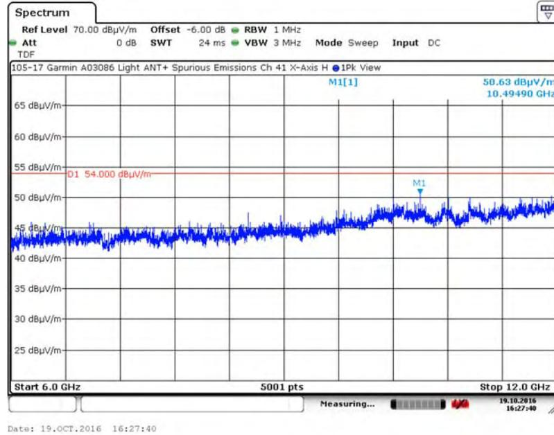
A.12.2. Measurement Results – DUT Position: X–Axis, Vertical Antenna
