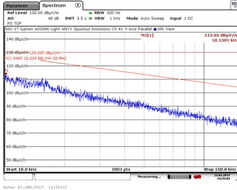
A.8.4. Measurement Results – DUT Position: Y– Axis, Perpendicular Antenna
