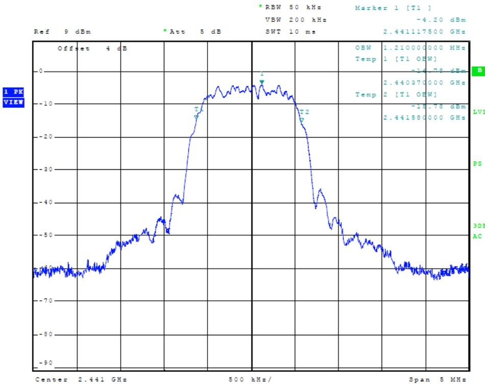
Figure 18 Plot of Transmitter Emissions (Pi4DQPSK, High Band Edge)
