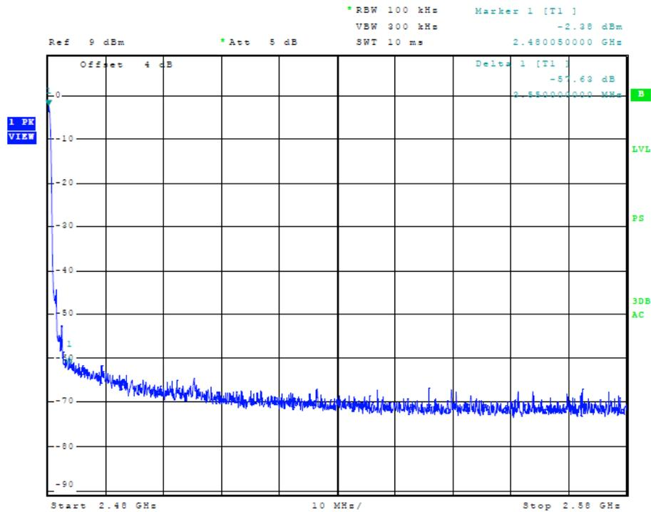
Figure 14 Plot of Transmitter Emissions (8DPSK, High Band Edge)
