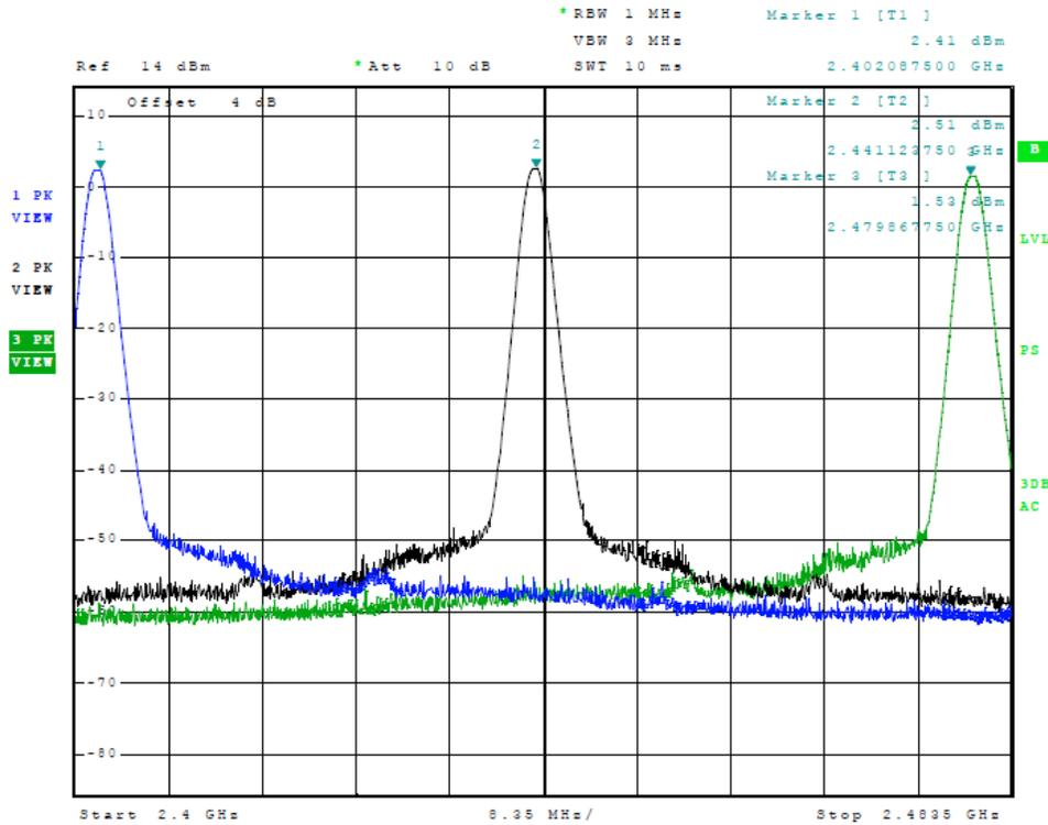
Figure 15 Plot of Transmitter Emissions (Pi4DQPSK Operation in 2402-2480 MHz)
