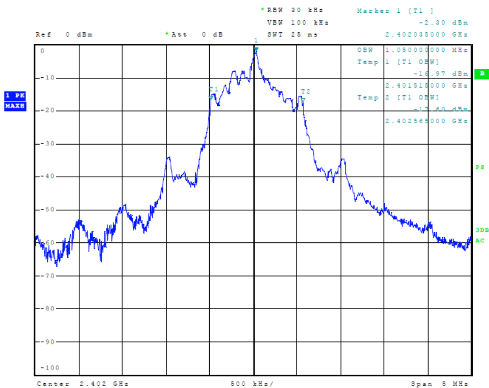
Figure 8 Plot of Transmitter Emissions (2402-2480 MHz, 99% Occupied Bandwidth)
