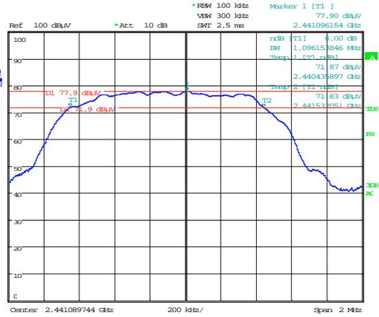
Figure 8.1-2: 6 dB bandwidth on mid channel
